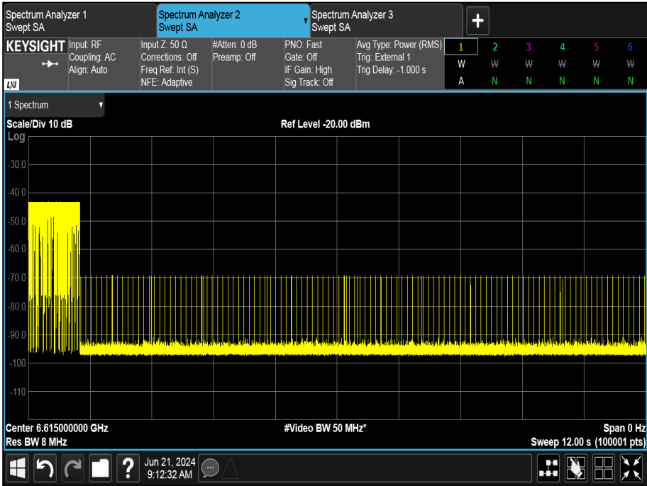
Figure 443 - U-NII-7, Minimum Bandwidth (AWGN Mid)
