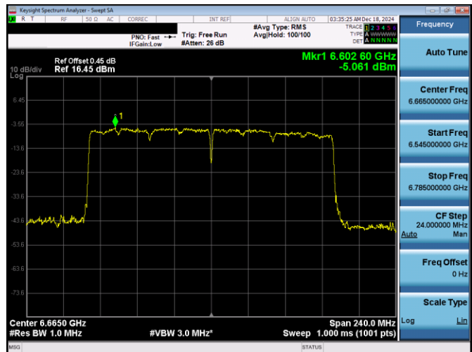
Plot 7-328. PSD Plot Antenna 1b (160MHz 802.11ax RU996x2 (UNII Band 7) – Ch. 143)
