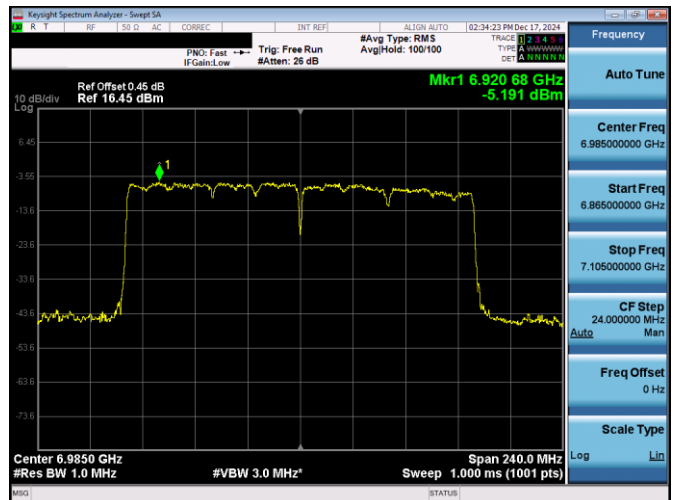
Plot 7-280. PSD Plot Antenna 3a (160MHz 802.11ax RU26 (UNII Band 8) – Ch. 207)
