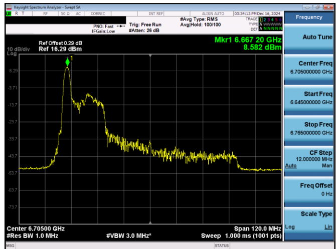
Plot 7-299. PSD Plot Antenna 1b (80MHz 802.11ax RU26 (UNII Band 7) – Ch. 151)
