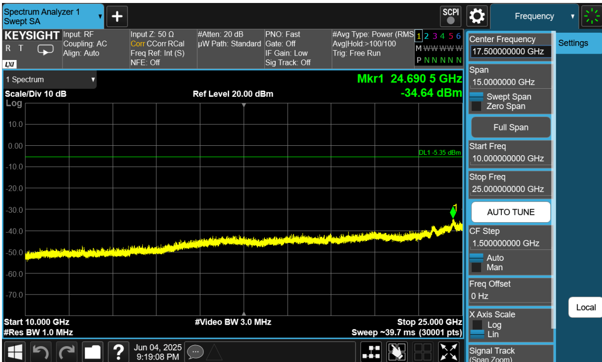
Plot 7-56. Conducted Spurious Plot Antenna 0 (Dedicated) (Bluetooth (LE), 1Mbps, iPA – Ch. 39)
