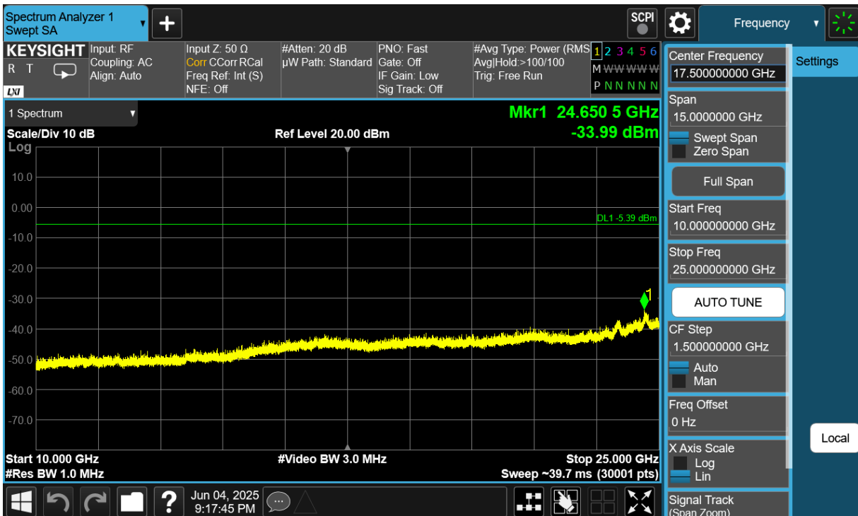
Plot 7-48. Conducted Spurious Plot Antenna 0 (Common) (Bluetooth (LE), 1Mbps, iPA – Ch. 17)
