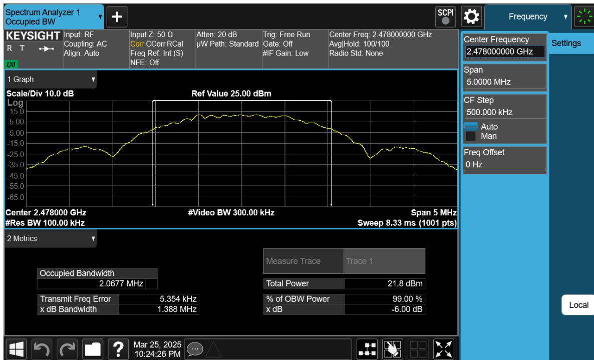
Plot 7-18. 6dB BW Plot Antenna 0 (Common) (Bluetooth (LE), 2Mbps, iPA – Ch. 36)
