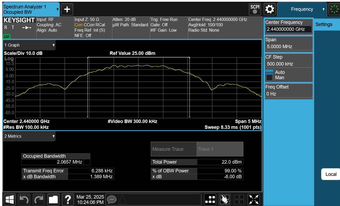
Plot 7-17. 6dB BW Plot Antenna 0 (Common) (Bluetooth (LE), 2Mbps, iPA – Ch. 17)
