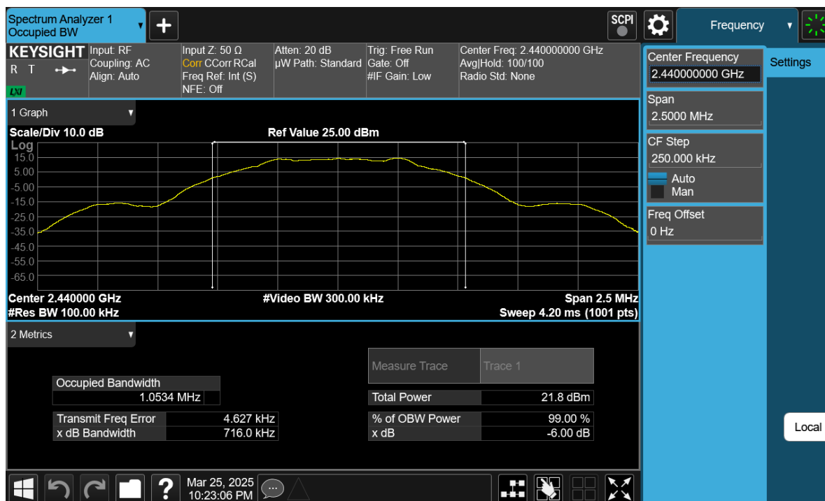
Plot 7-14. 6dB BW Plot Antenna 0 (Common) (Bluetooth (LE), 1Mbps, iPA – Ch. 17)
