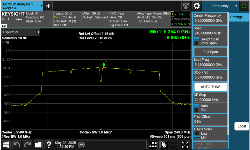
Plot 7-50. PSD CDD Antenna 1 (160MHz BW 802.11ac - Ch. 50)
