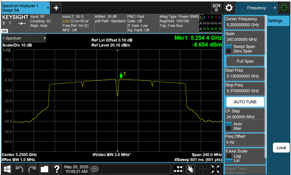
Plot 7-49. PSD CDD Antenna 0 (160MHz BW 802.11ac – Ch. 50)
