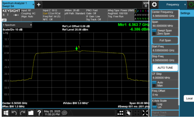
Plot 7-53. Power Spectral Density Plot Antenna 0 (40MHz 802.11ax (UNII Band 7) – Ch. 123, MCS4)
