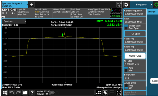
Plot 7-62. Power Spectral Density Plot Antenna 0 (40MHz 802.11ax (UNII Band 6) – Ch. 107)
