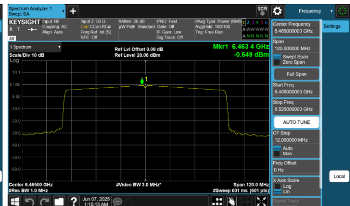
Plot 7-126. Power Spectral Density Plot CDD Antenna 1 (80MHz 802.11ax (UNII Band 6) – Ch. 103)
