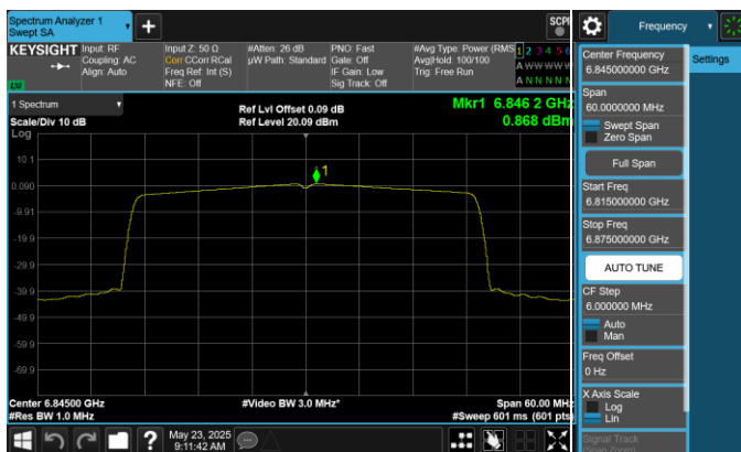
Plot 7-66. Power Spectral Density Plot Antenna 0 (40MHz 802.11ax (UNII Band 7) – Ch. 179)
