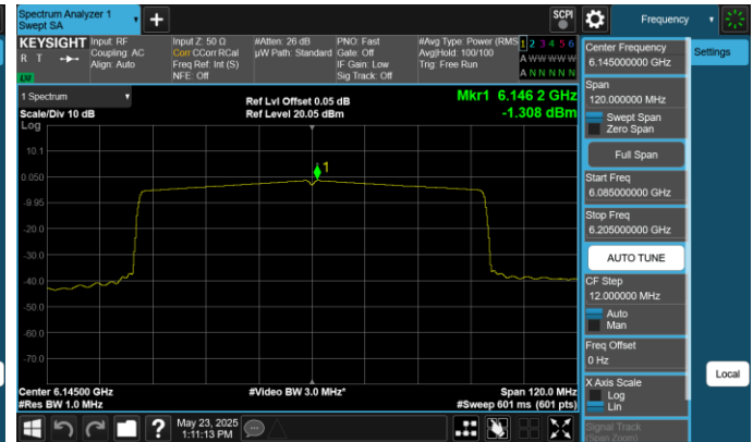
Plot 7-87. Power Spectral Density Plot Antenna 1 (80MHz 802.11ax (UNII Band 5) – Ch. 39)
