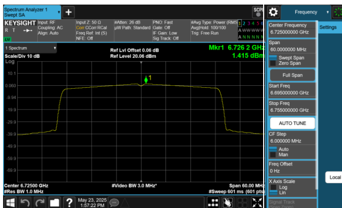
Plot 7-94. Power Spectral Density Plot Antenna 1 (40MHz 802.11ax (UNII Band 7) – Ch. 155)
