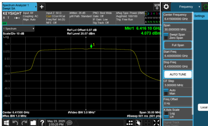
Plot 7-114. Power Spectral Density Plot CDD Antenna 1 (20MHz 802.11ax (UNII Band 5) – Ch. 93)
