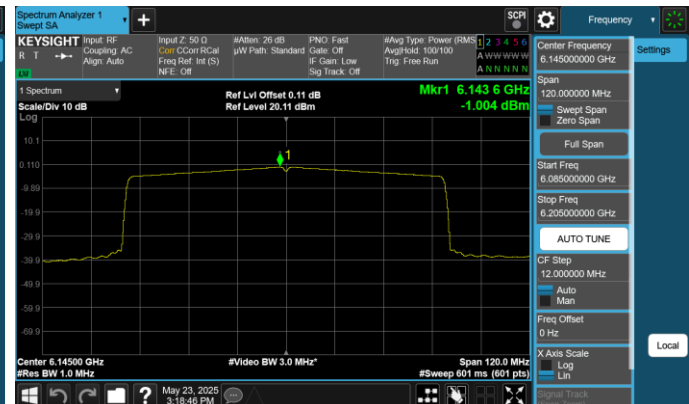
Plot 7-118. Power Spectral Density Plot CDD Antenna 1 (80MHz 802.11ax (UNII Band 5) – Ch. 39)
