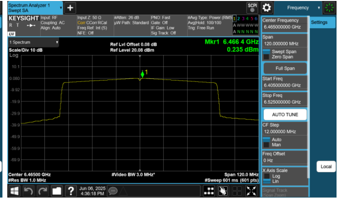
Plot 7-63. Power Spectral Density Plot Antenna 0 (80MHz 802.11ax (UNII Band 6) – Ch. 103)
