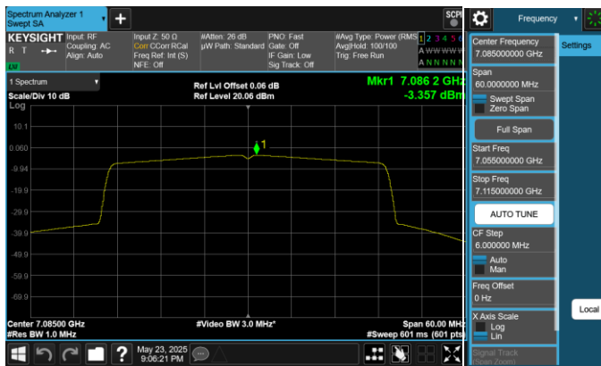
Plot 7-110. Power Spectral Density Plot Antenna 1 (40MHz 802.11ax (UNII Band 8) – Ch. 227)
