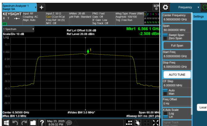
Plot 7-106. Power Spectral Density Plot Antenna 1 (40MHz 802.11ax (UNII Band 7) – Ch. 123)
