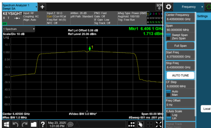
Plot 7-86. Power Spectral Density Plot Antenna 1 (40MHz 802.11ax (UNII Band 5) – Ch. 91)
