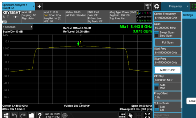
Plot 7-123. Power Spectral Density Plot CDD Antenna 0 (40MHz 802.11ax (UNII Band 6) – Ch. 99)
