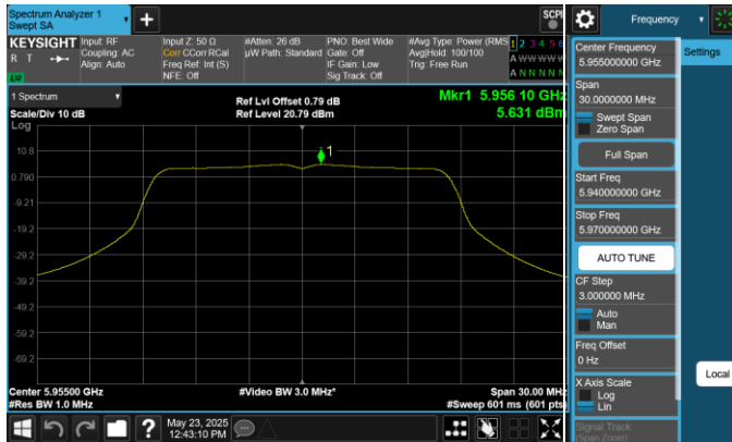
Plot 7-85. Power Spectral Density Plot Antenna 1 (20MHz 802.11a (UNII Band 5) – Ch. 1)
