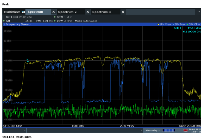
Plot 7-298. 160MHz Bandwidth, AWGN Signal Injected – 6110Mhz
