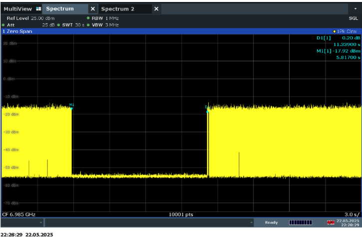
Plot 7-297. Contention Based Protocol Timing Plot – UNII 8 – 160MHz Channel 207 – High
