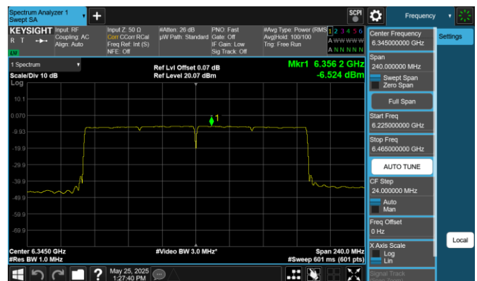
Plot 7-144. PSD Plot Antenna 0 (160MHz 802.11ax RU996x2 (UNII Band 5) – Ch. 79)
