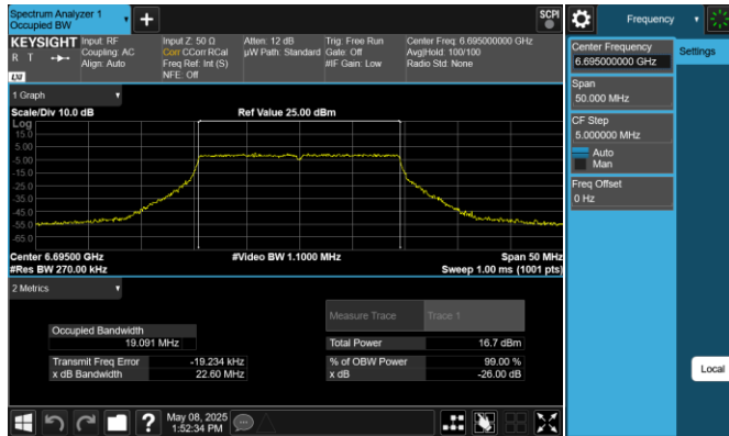
Plot 7-101. 26dB & 99% Bandwidth Plot Antenna 1 (20MHz 802.11ax RU242 (UNII Band 7) – Ch. 149)
