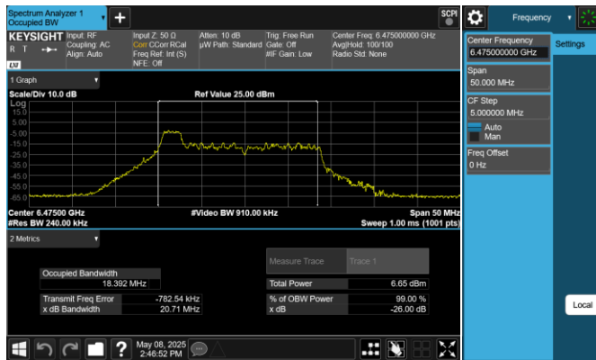
Plot 7-89. 26dB & 99% Bandwidth Plot Antenna 1 (20MHz 802.11ax RU26 (UNII Band 6) – Ch. 105)
