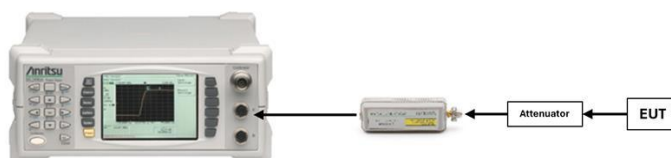
Figure 7-2. Test Instrument & Measurement Setup
