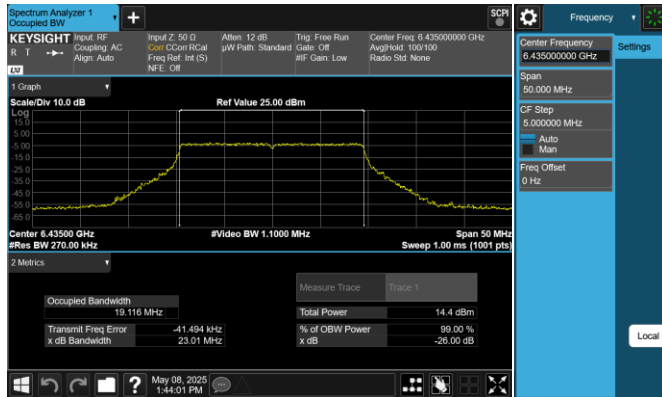
Plot 7-93. 26dB & 99% Bandwidth Plot Antenna 1 (20MHz 802.11ax RU242 (UNII Band 6) – Ch. 97)
