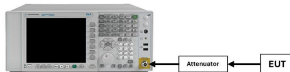
Figure 7-3. Test Instrument & Measurement Setup
