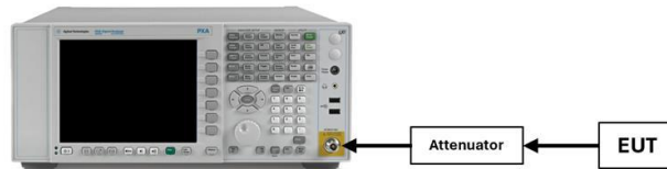
Figure 7-4. Test Instrument & Measurement Setup
