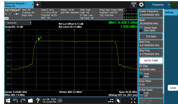
Plot 7-182. PSD Plot Antenna 1 (40MHz 802.11ax RU484 (UNII Band 6) – Ch. 99)
