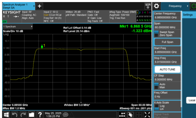
Plot 7-166. PSD Plot Antenna 0 (40MHz 802.11ax RU484 (UNII Band 8) – Ch. 187)
