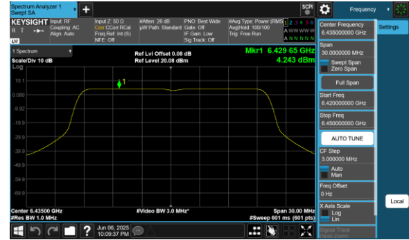
Plot 7-181. PSD Plot Antenna 1 (20MHz 802.11ax RU242 (UNII Band 6) – Ch. 97)
