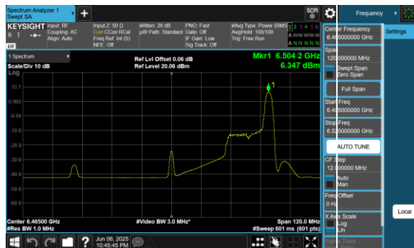
Plot 7-179. PSD Plot Antenna 1 (80MHz 802.11ax RU26 (UNII Band 6) – Ch. 103)
