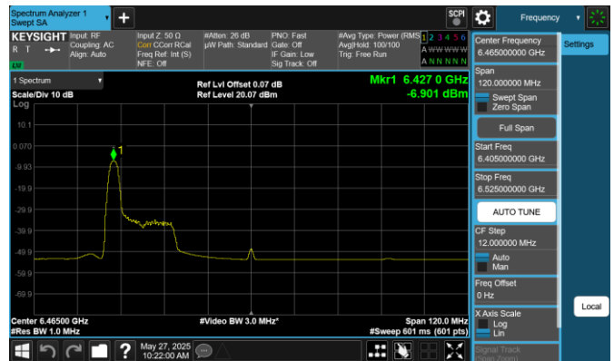
Plot 7-203. PSD Plot Antenna 1 (80MHz 802.11ax RU26 (UNII Band 6) – Ch. 103)
