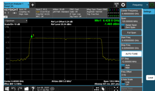
Plot 7-183. PSD Plot Antenna 1 (80MHz 802.11ax RU996 (UNII Band 6) – Ch. 103)
