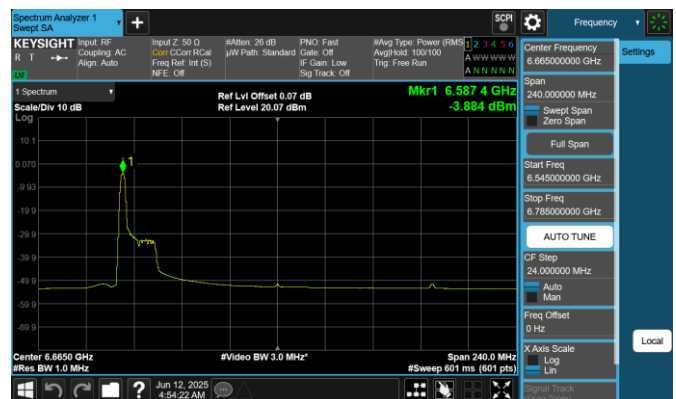
Plot 7-156. PSD Plot Antenna 0 (160MHz 802.11ax RU26 (UNII Band 7) – Ch. 143)
