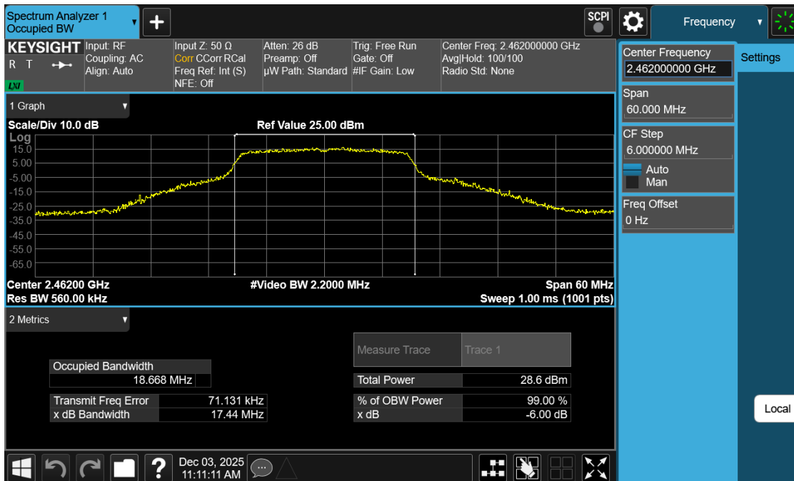
Plot 7-15. 99% OBW Plot Antenna 1 Dedicated (802.11n – Ch. 11)
