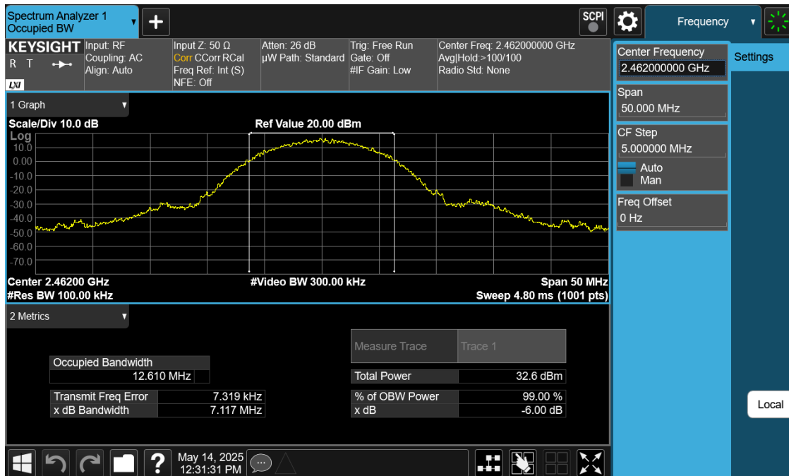
Plot 7-25. 6 dB BW Plot Antenna 0 Dedicated (802.11b – Ch. 11)
