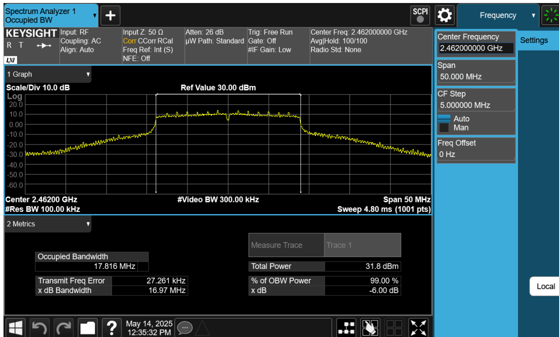
Plot 7-27. 6 dB BW Plot Antenna 0 Dedicated (802.11n – Ch. 11)
