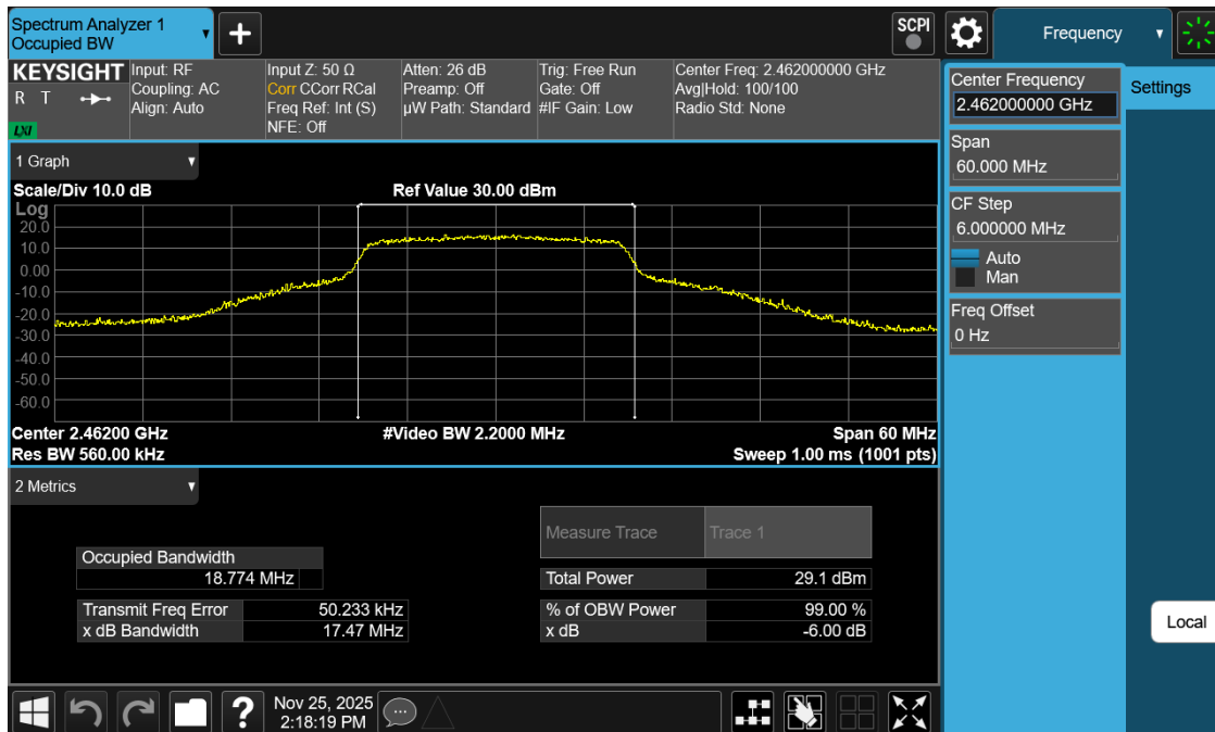
Plot 7-11. 99% OBW Plot Antenna 0 Dedicated (802.11n – Ch. 11)
