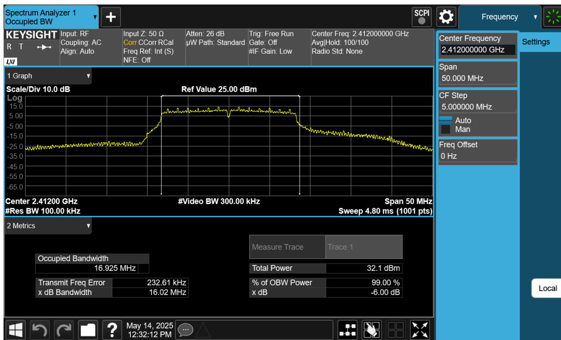
Plot 7-26. 6 dB BW Plot Antenna 0 Dedicated (802.11g – Ch. 1)
