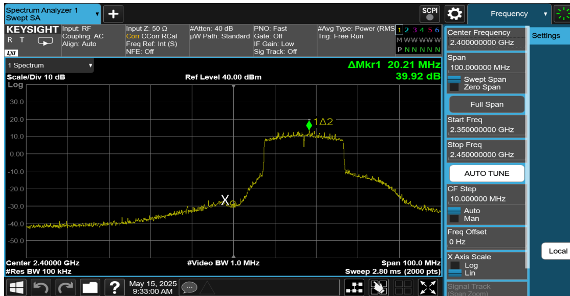
Plot 7-118. Band Edge Plot Antenna 1 Dedicated (802.11ax (SU - 2.4GHz) – Ch. 2)
