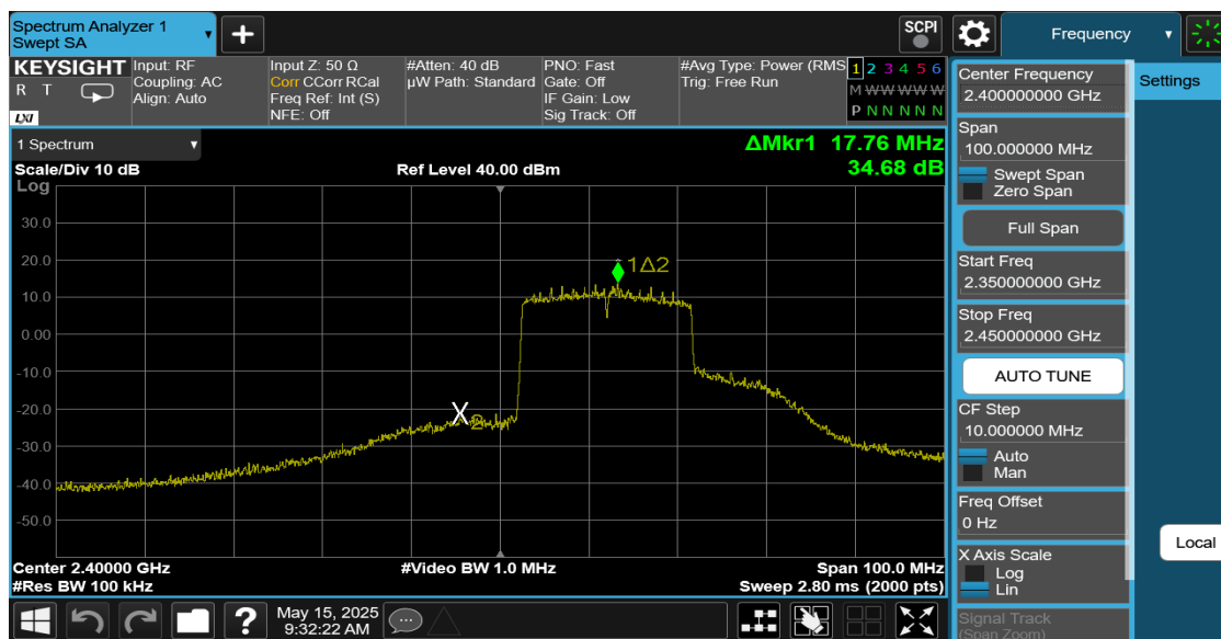
Plot 7-117. Band Edge Plot Antenna 1 Dedicated (802.11ax (SU - 2.4GHz) – Ch. 1)
