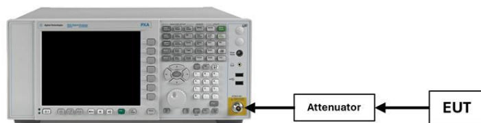
Figure 7-4. Test Instrument & Measurement Setup
