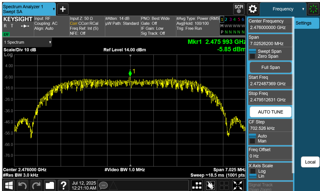
Plot 7-117. Power Spectral Density Plot Antenna WF7 (Bluetooth (HDRPM16), 16Mbps, ePA – Ch. 73)
