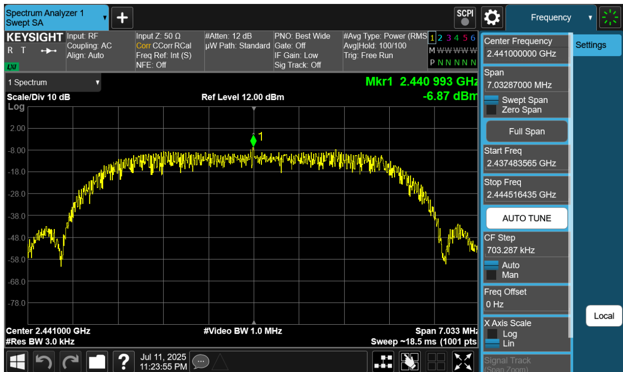
Plot 7-80. Power Spectral Density Plot Antenna WF8 (Bluetooth (HDRPM16), 16Mbps, ePA – Ch. 38)
