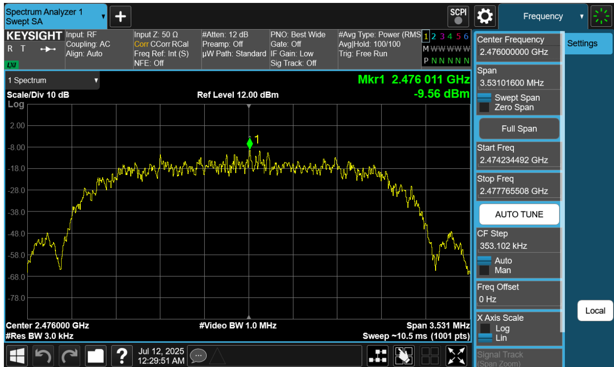
Plot 7-96. Power Spectral Density Plot Antenna WF7 (Bluetooth (HDR4), 4Mbps, iPA – Ch. 73)
