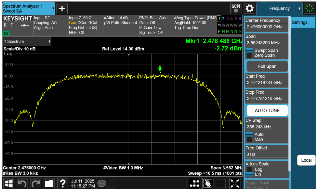
Plot 7-69. Power Spectral Density Plot Antenna WF8 (Bluetooth (HDRPS2), 2Mbps, ePA – Ch. 73)
