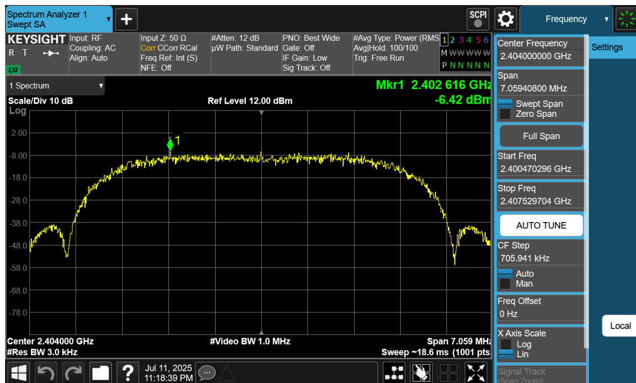
Plot 7-73. Power Spectral Density Plot Antenna WF8 (Bluetooth (XHDRPM6), 6Mbps, ePA – Ch. 1)
