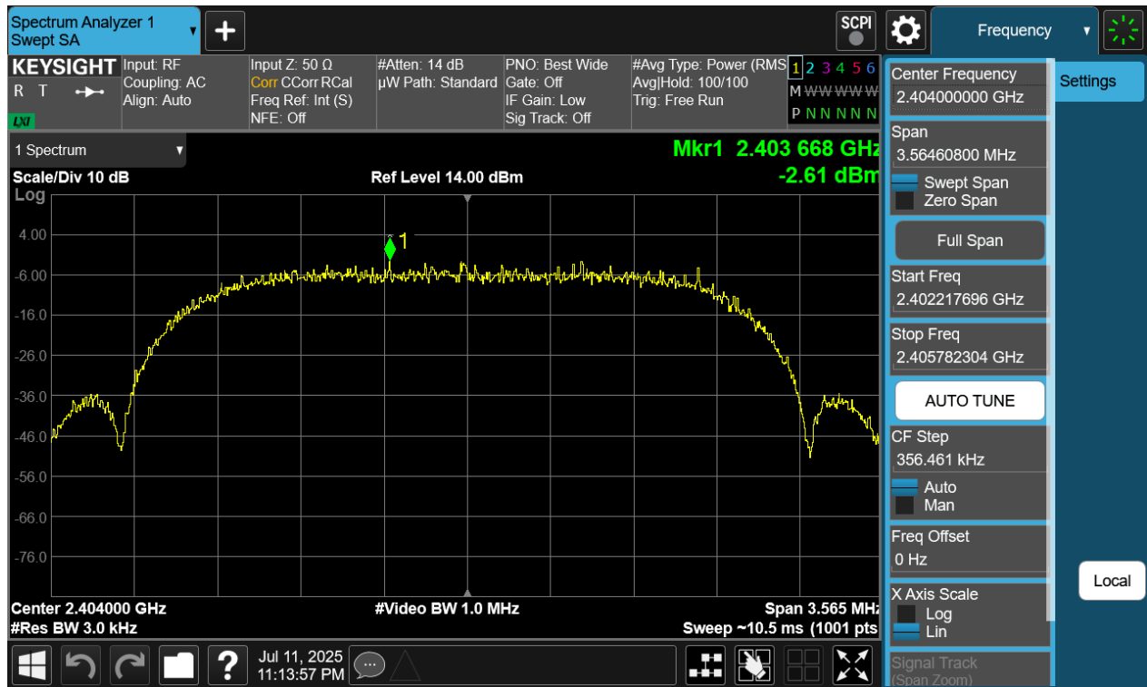
Plot 7-67. Power Spectral Density Plot Antenna WF8 (Bluetooth (HDRPS2), 2Mbps, ePA – Ch. 1)
