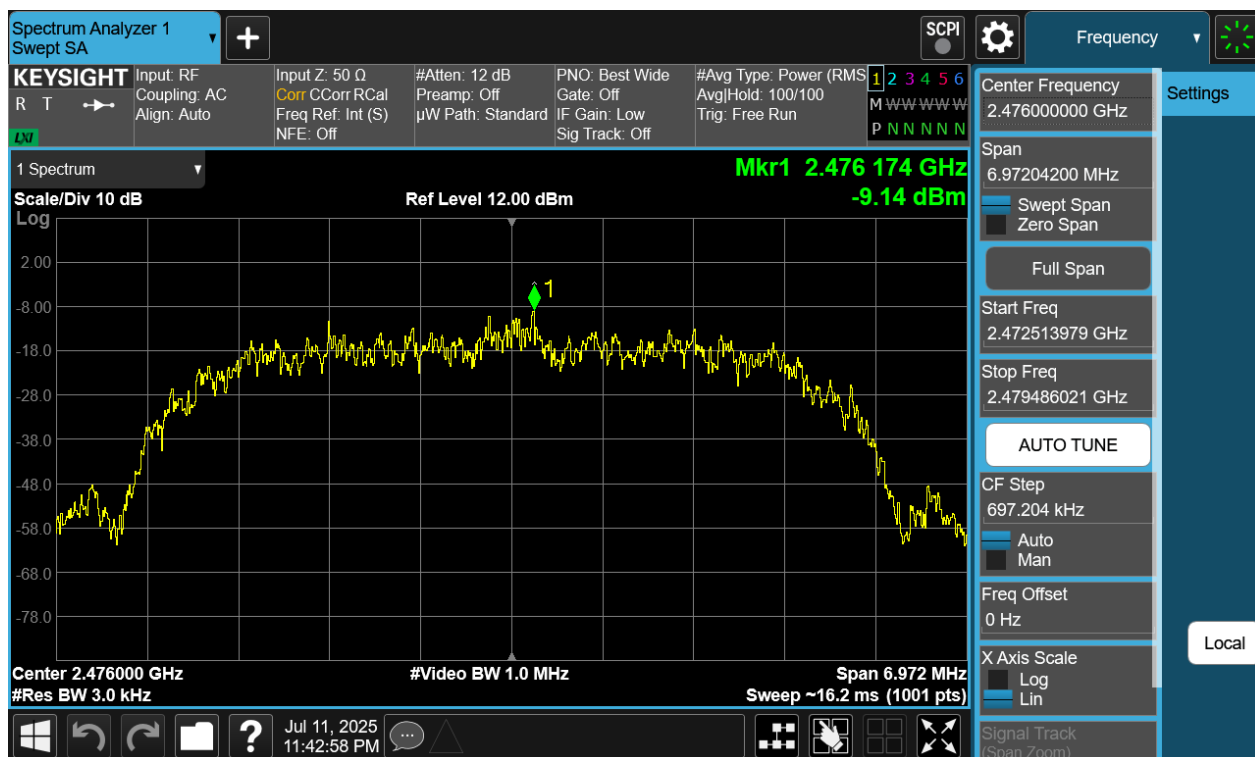
Plot 7-66. Power Spectral Density Plot Antenna WF8 (Bluetooth (HDR8), 8Mbps, iPA – Ch. 73)
