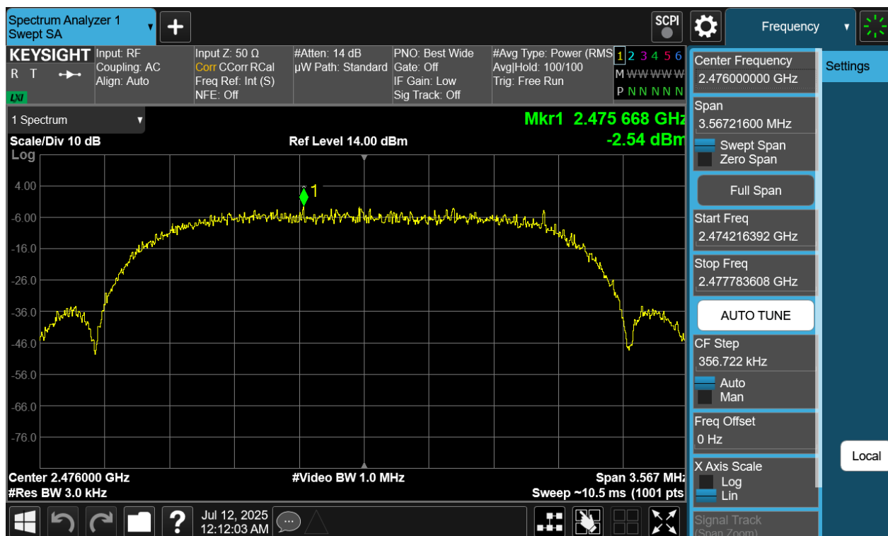
Plot 7-105. Power Spectral Density Plot Antenna WF7 (Bluetooth (HDRPS2), 2Mbps, ePA – Ch. 73)
