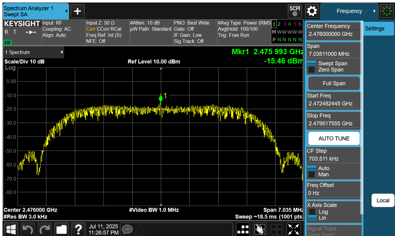
Plot 7-84. Power Spectral Density Plot Antenna WF8 (Bluetooth (HDRPM16), 16Mbps, iPA – Ch. 73)
