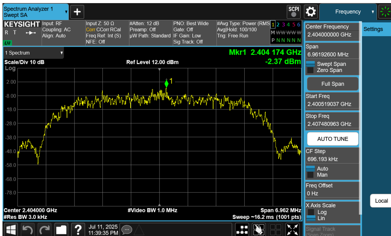
Plot 7-61. Power Spectral Density Plot Antenna WF8 (Bluetooth (HDR8), 8Mbps, ePA – Ch. 1)
