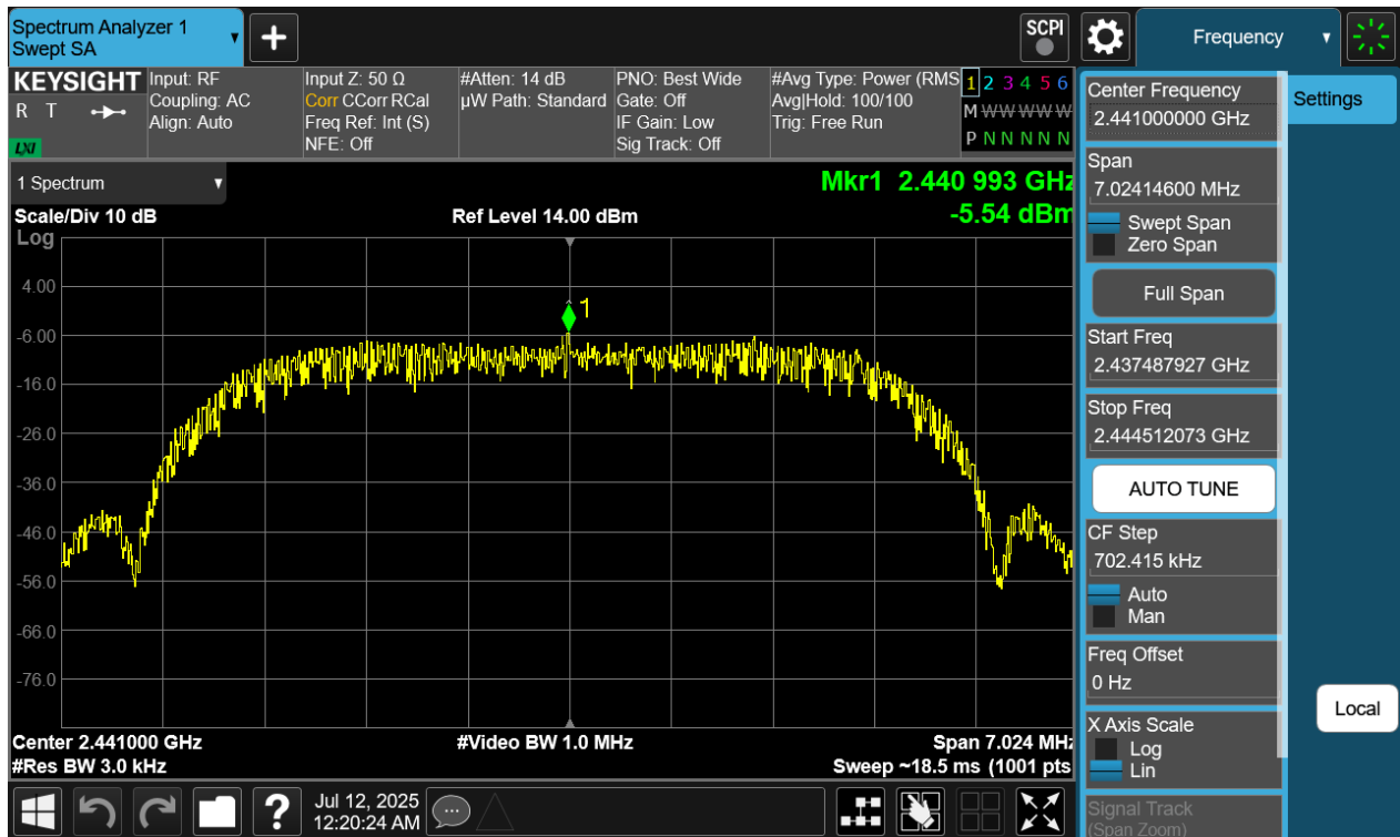
Plot 7-116. Power Spectral Density Plot Antenna WF7 (Bluetooth (HDRPM16), 16Mbps, ePA – Ch. 38)
