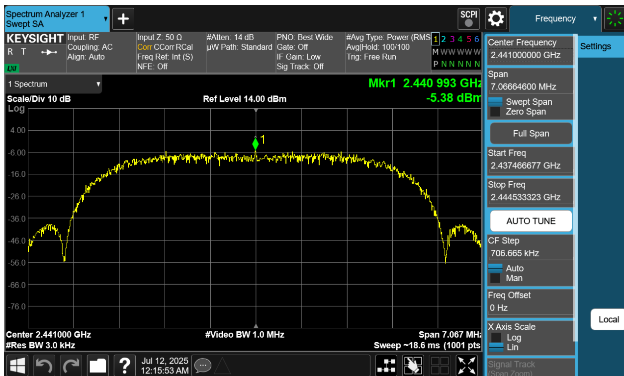
Plot 7-110. Power Spectral Density Plot Antenna WF7 (Bluetooth (XHDRPM6), 6Mbps, ePA – Ch. 38)
