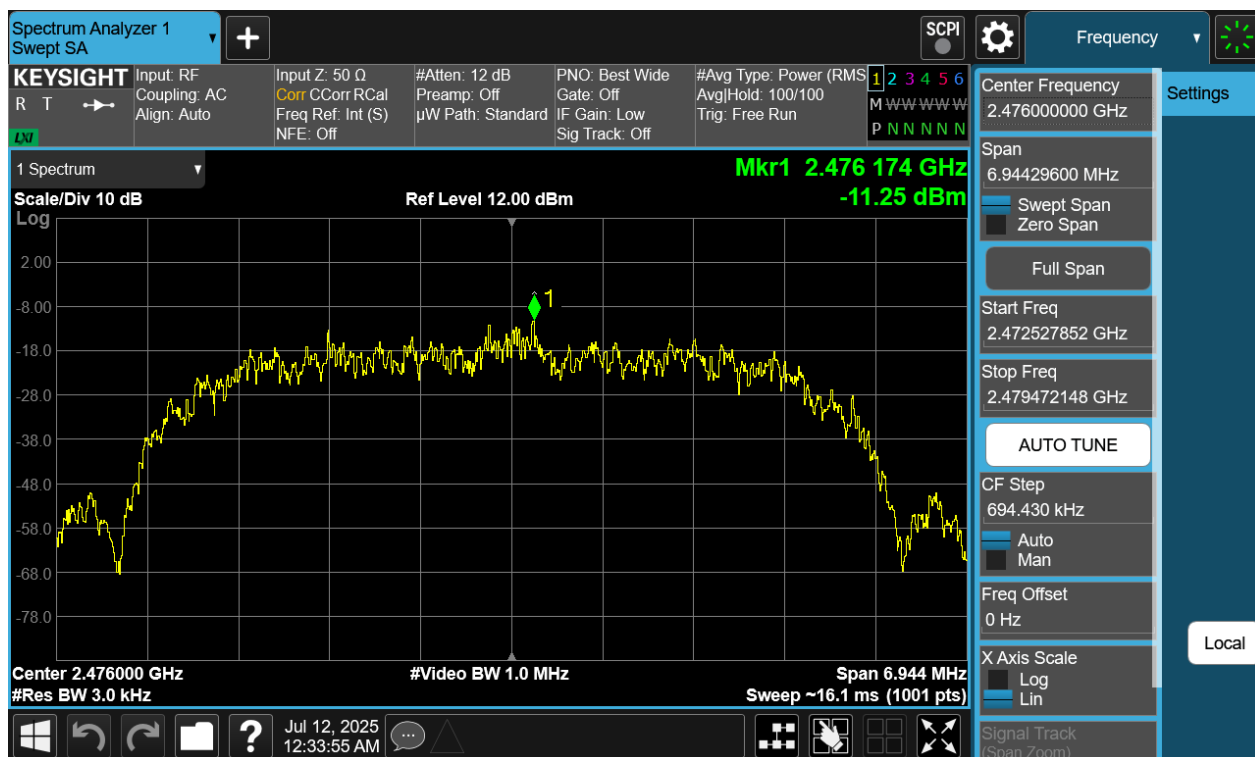
Plot 7-102. Power Spectral Density Plot Antenna WF7 (Bluetooth (HDR8), 8Mbps, iPA – Ch. 73)
