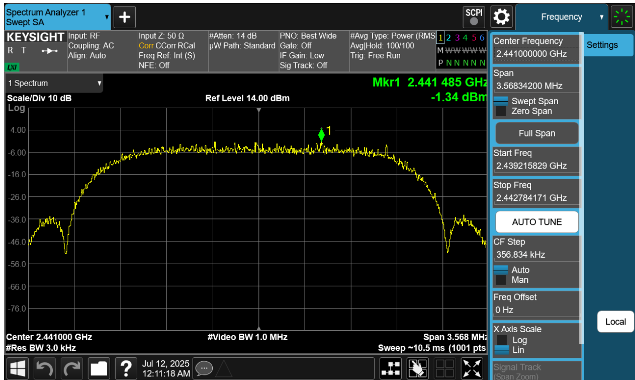
Plot 7-104. Power Spectral Density Plot Antenna WF7 (Bluetooth (HDRPS2), 2Mbps, ePA – Ch. 38)
