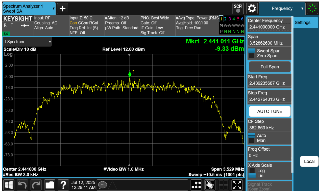
Plot 7-95. Power Spectral Density Plot Antenna WF7 (Bluetooth (HDR4), 4Mbps, iPA – Ch. 38)
