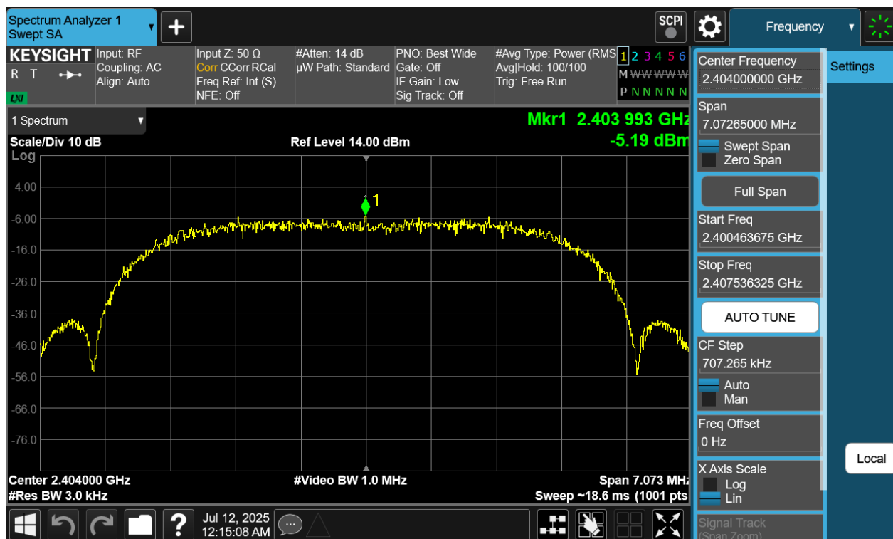
Plot 7-109. Power Spectral Density Plot Antenna WF7 (Bluetooth (XHDRPM6), 6Mbps, ePA – Ch. 1)
