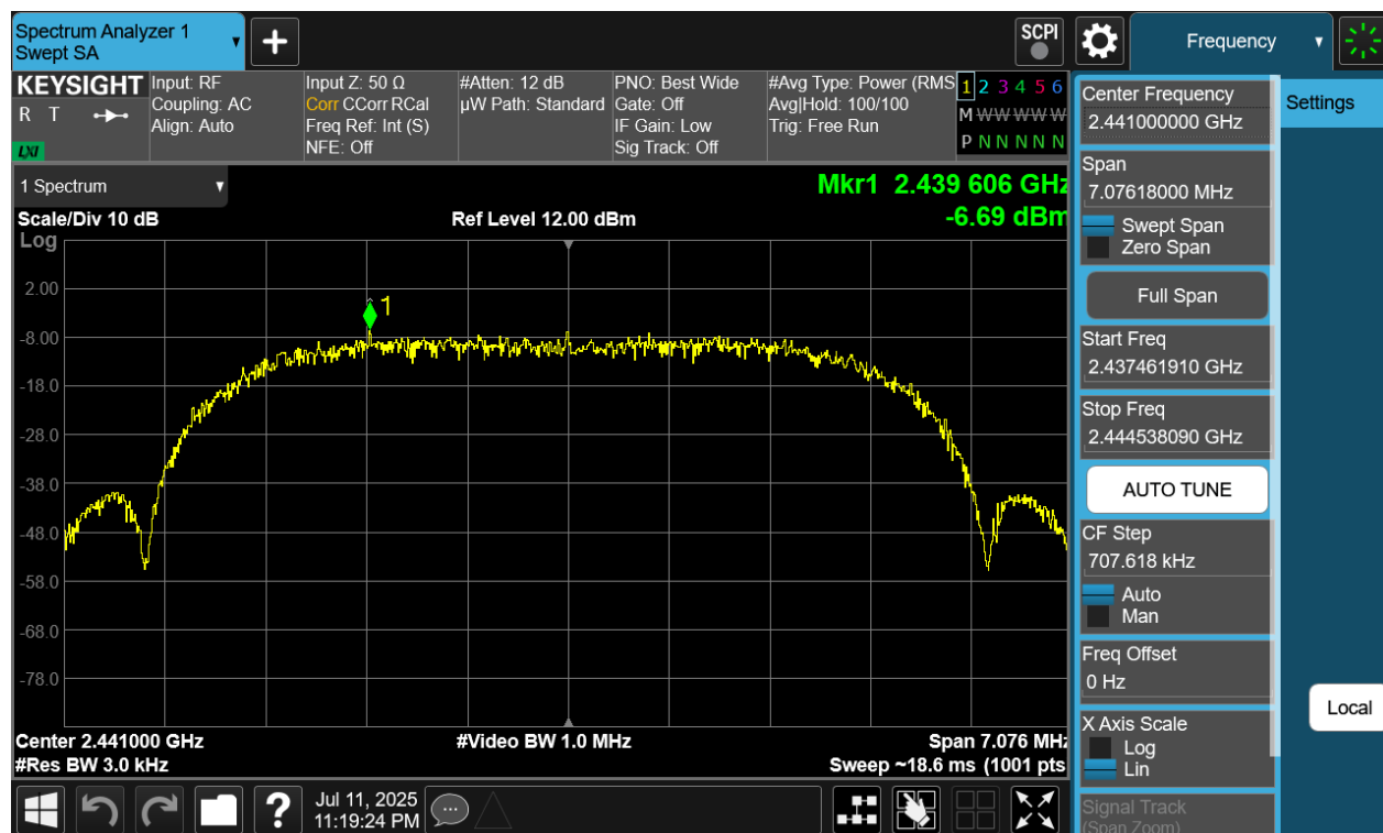
Plot 7-74. Power Spectral Density Plot Antenna WF8 (Bluetooth (XHDRPM6), 6Mbps, ePA – Ch. 38)
