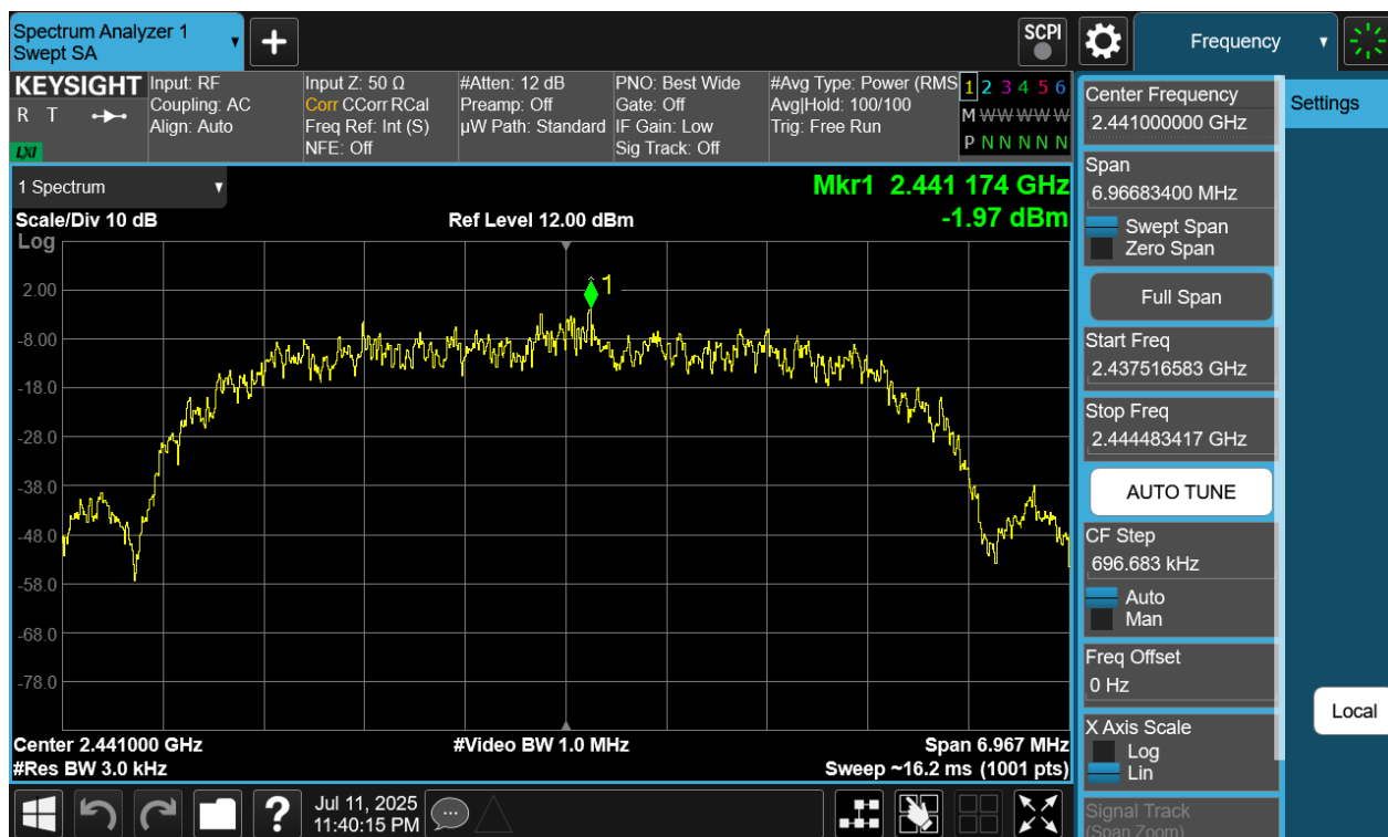
Plot 7-62. Power Spectral Density Plot Antenna WF8 (Bluetooth (HDR8), 8Mbps, ePA – Ch. 38)
