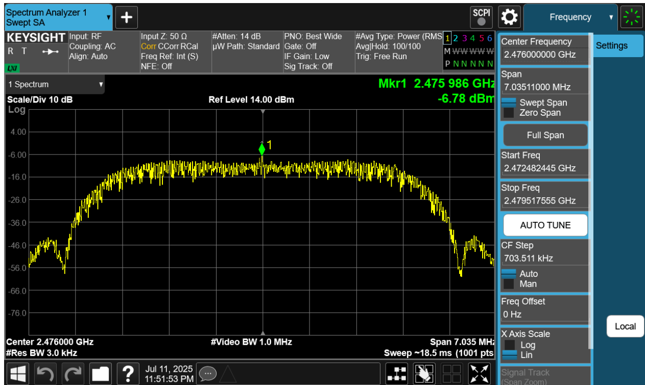
Plot 7-287. Power Spectral Density Plot Tx BF Diversity Antenna WF8 (Bluetooth (HDRPM16), 16Mbps, ePA – Ch. 73)
