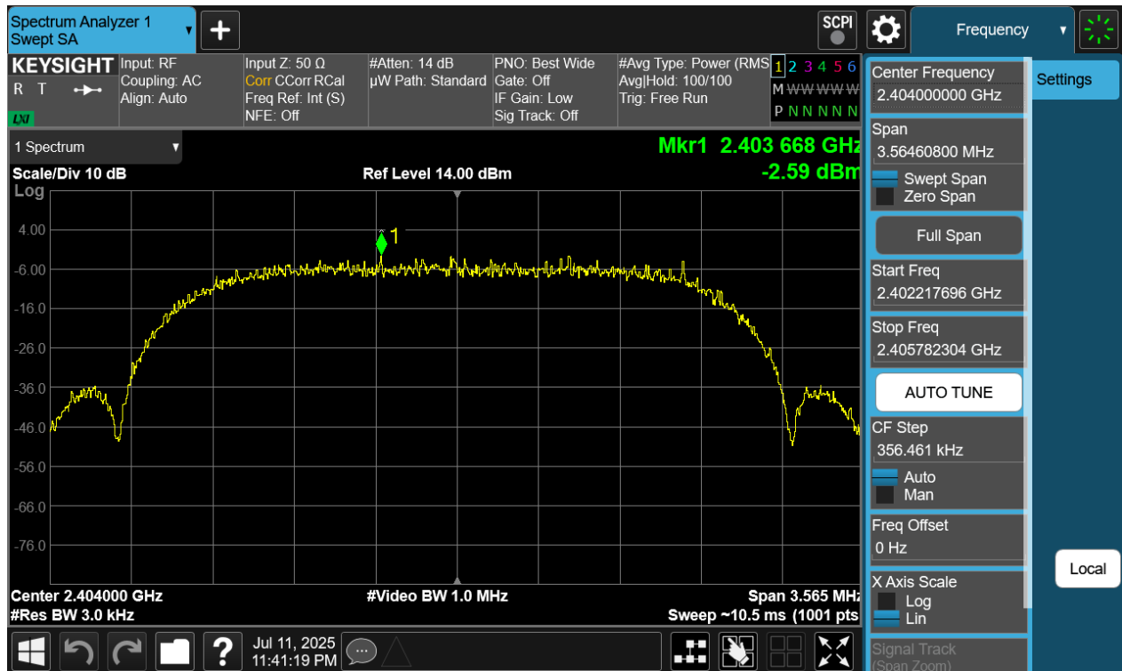
Plot 7-259. Power Spectral Density Plot TxBF Diversity Antenna WF8 (Bluetooth (HDRPS2), 8Mbps, ePA – Ch. 1)
