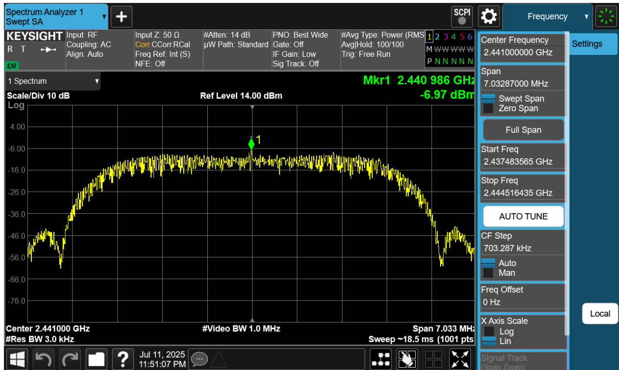
Plot 7-285. Power Spectral Density Plot Tx BF Diversity Antenna WF8 (Bluetooth (HDRPM16), 16Mbps, ePA – Ch. 38)
