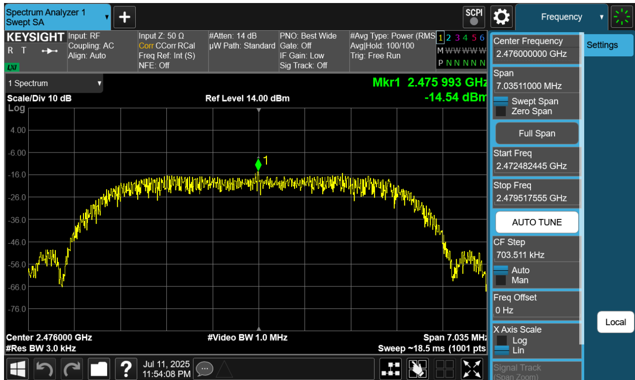
Plot 7-293. Power Spectral Density Plot Tx BF Diversity Antenna WF8 (Bluetooth (HDRPM16), 16Mbps, iPA – Ch. 73)
