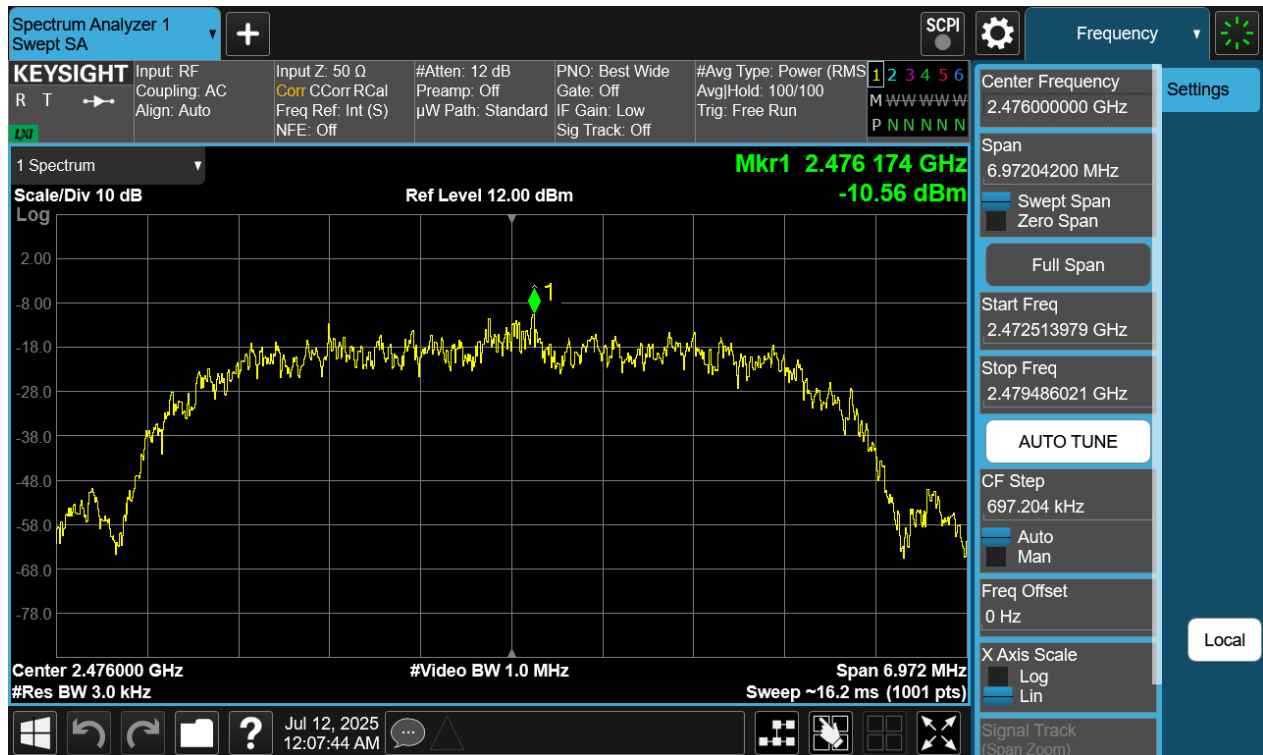
Plot 7-257. Power Spectral Density Plot Tx BF Diversity Antenna WF8 (Bluetooth (HDR8), 8Mbps, iPA – Ch. 73)
