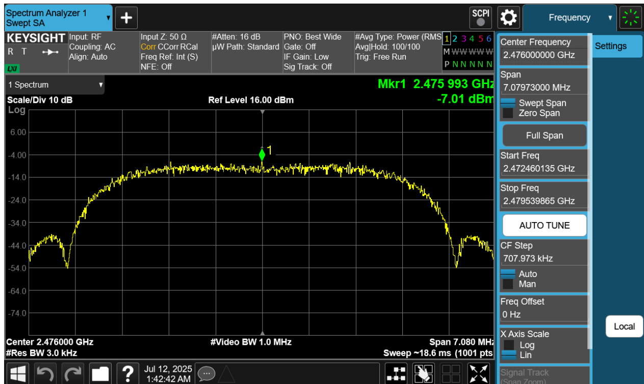
Plot 7-276. Power Spectral Density Plot Tx BF Diversity Antenna WF9 (Bluetooth (XHDRPM6), 6Mbps, ePA – Ch. 73)
