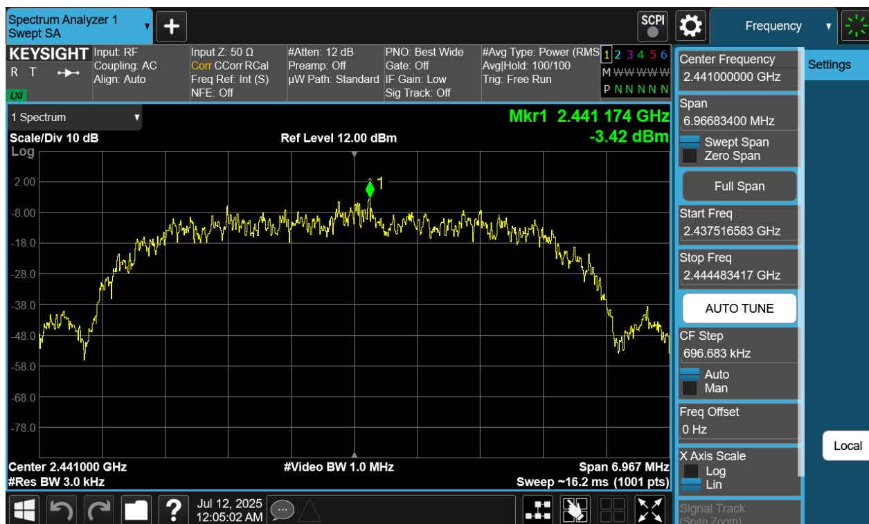
Plot 7-249. Power Spectral Density Plot Tx BF Diversity Antenna WF8 (Bluetooth (HDR8), 8Mbps, ePA – Ch. 38)
