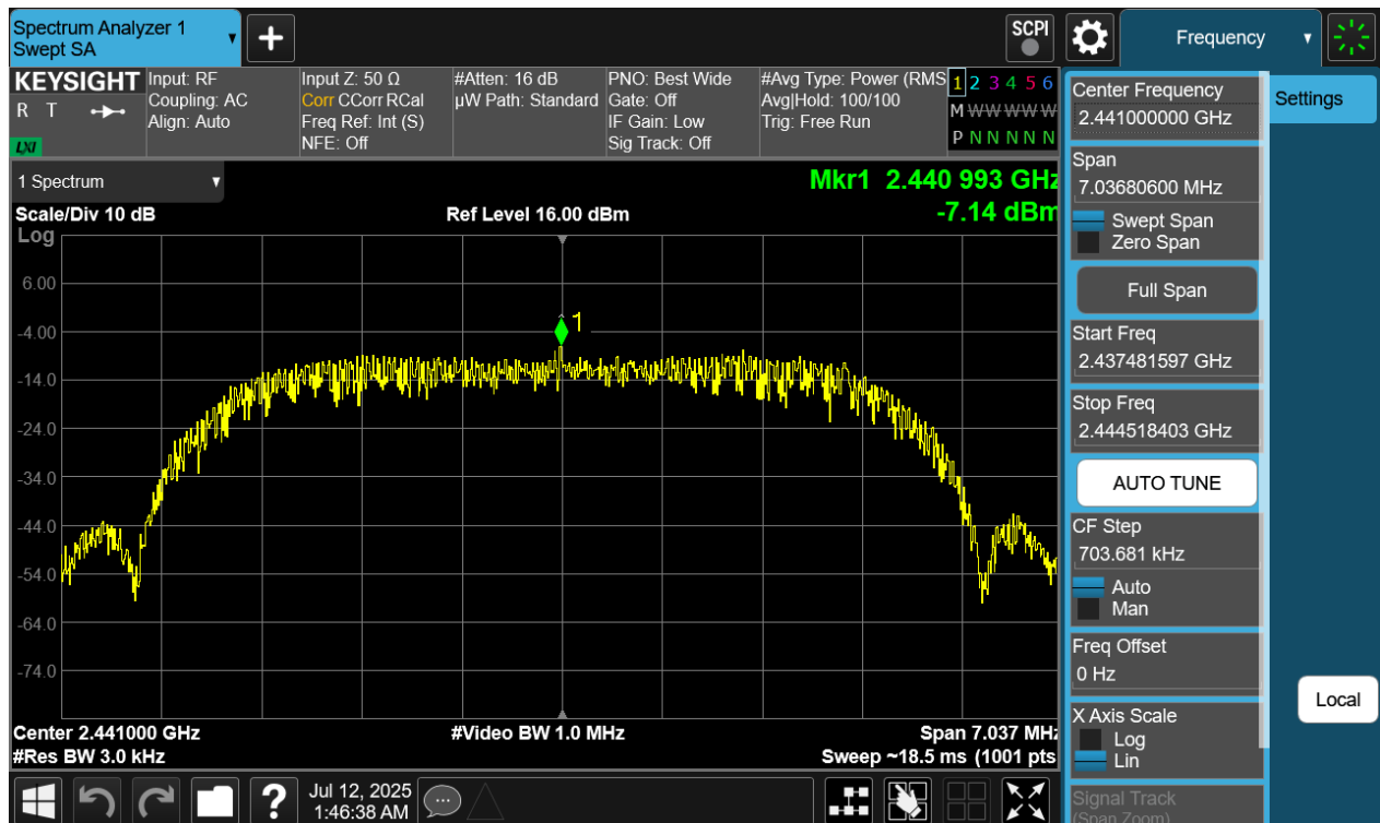
Plot 7-286. Power Spectral Density Plot Tx BF Diversity Antenna WF9 (Bluetooth (HDRPM16), 16Mbps, ePA – Ch. 38)
