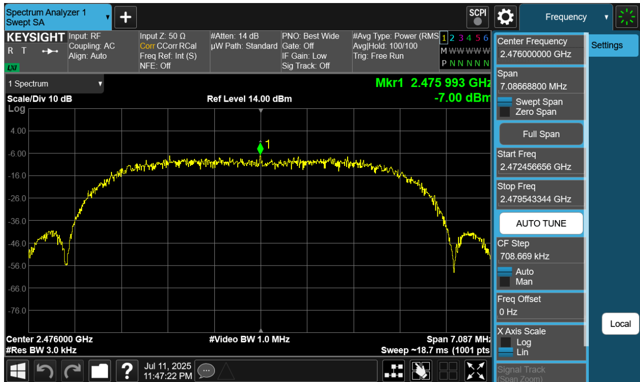
Plot 7-275. Power Spectral Density Plot Tx BF Diversity Antenna WF8 (Bluetooth (XHDRPM6), 6Mbps, ePA – Ch. 73)
