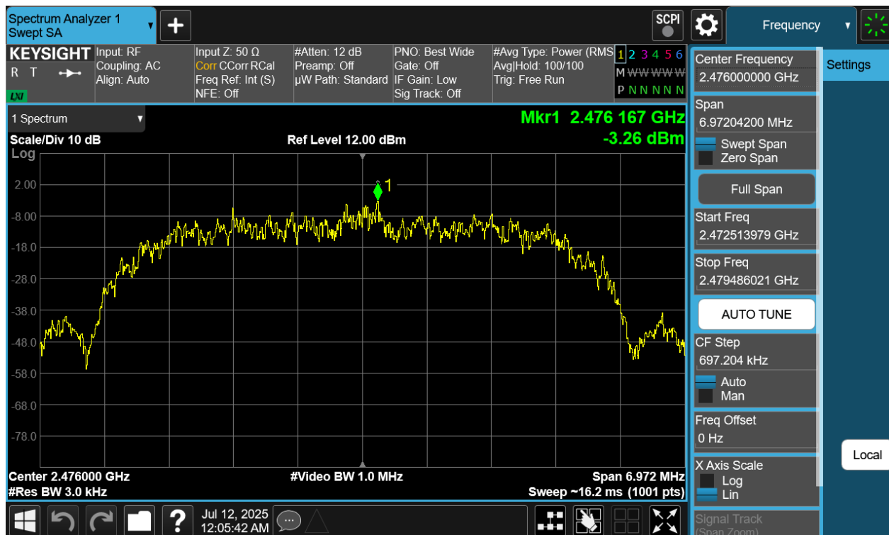
Plot 7-251. Power Spectral Density Plot Tx BF Diversity Antenna WF8 (Bluetooth (HDR8), 8Mbps, ePA – Ch. 73)
