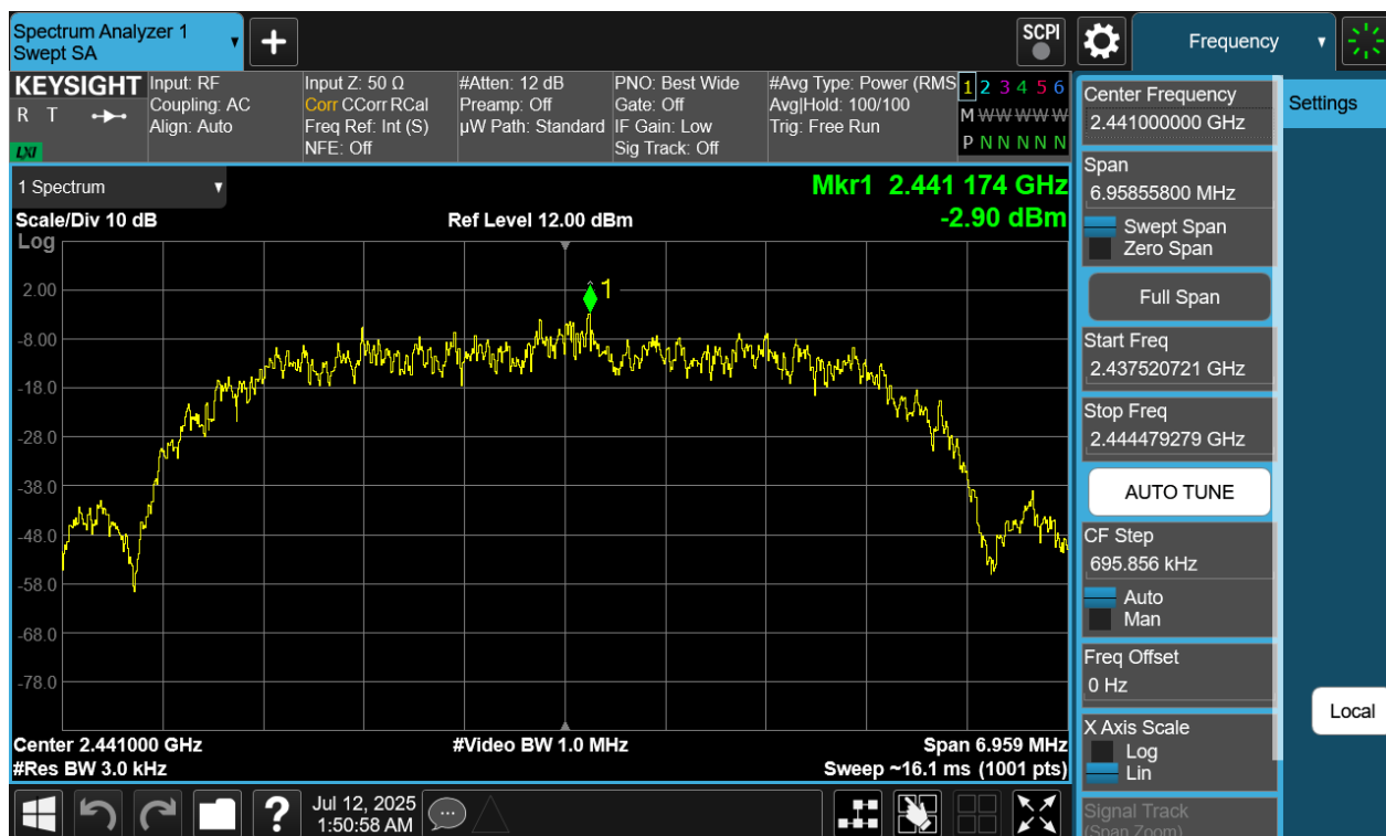
Plot 7-250. Power Spectral Density Plot Tx BF Diversity Antenna WF9 (Bluetooth (HDR8), 8Mbps, ePA – Ch. 38)
