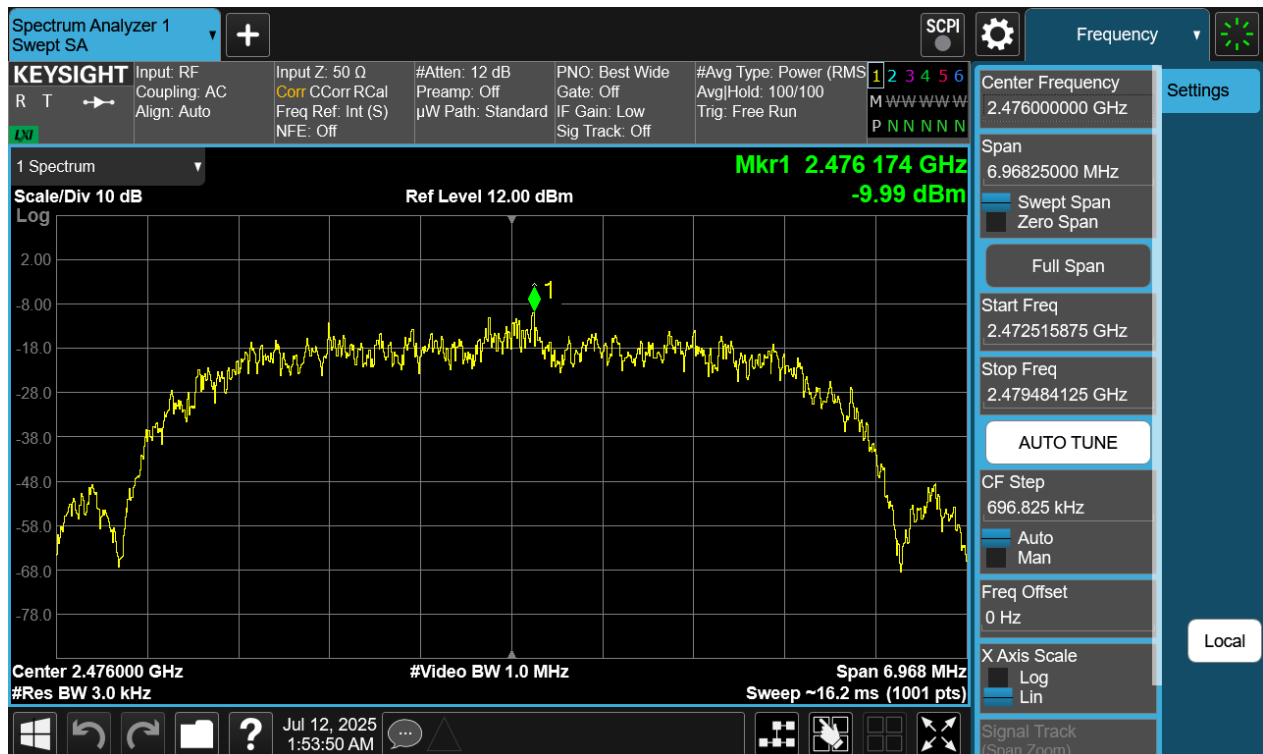
Plot 7-258. Power Spectral Density Plot Tx BF Diversity Antenna WF9 (Bluetooth (HDR8), 8Mbps, iPA – Ch. 73)
