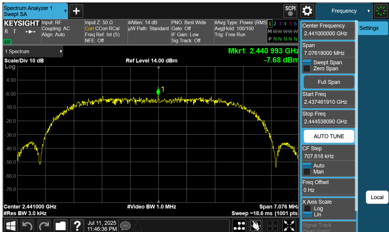
Plot 7-273. Power Spectral Density Plot Tx BF Diversity Antenna WF8 (Bluetooth (XHDRPM6), 6Mbps, ePA – Ch. 38)
