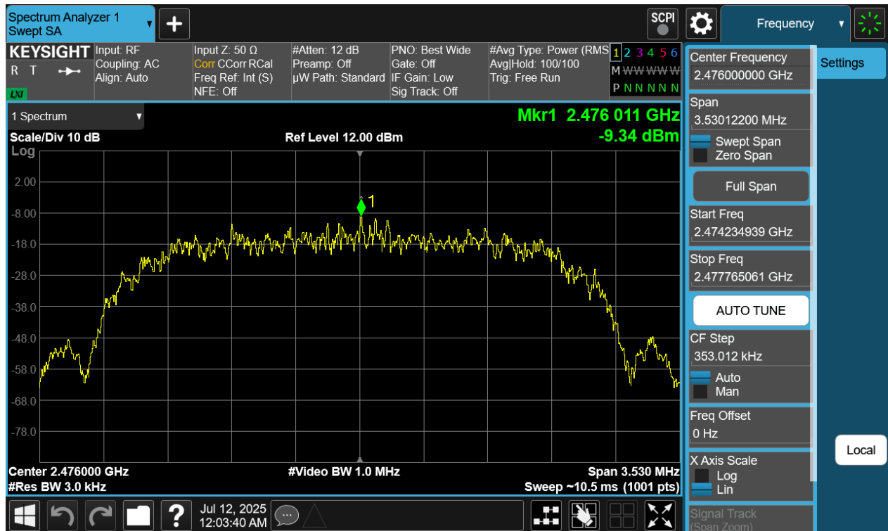
Plot 7-245. Power Spectral Density Plot Tx BF Diversity Antenna WF8 (Bluetooth (HDR4), 4Mbps, iPA – Ch. 73)
