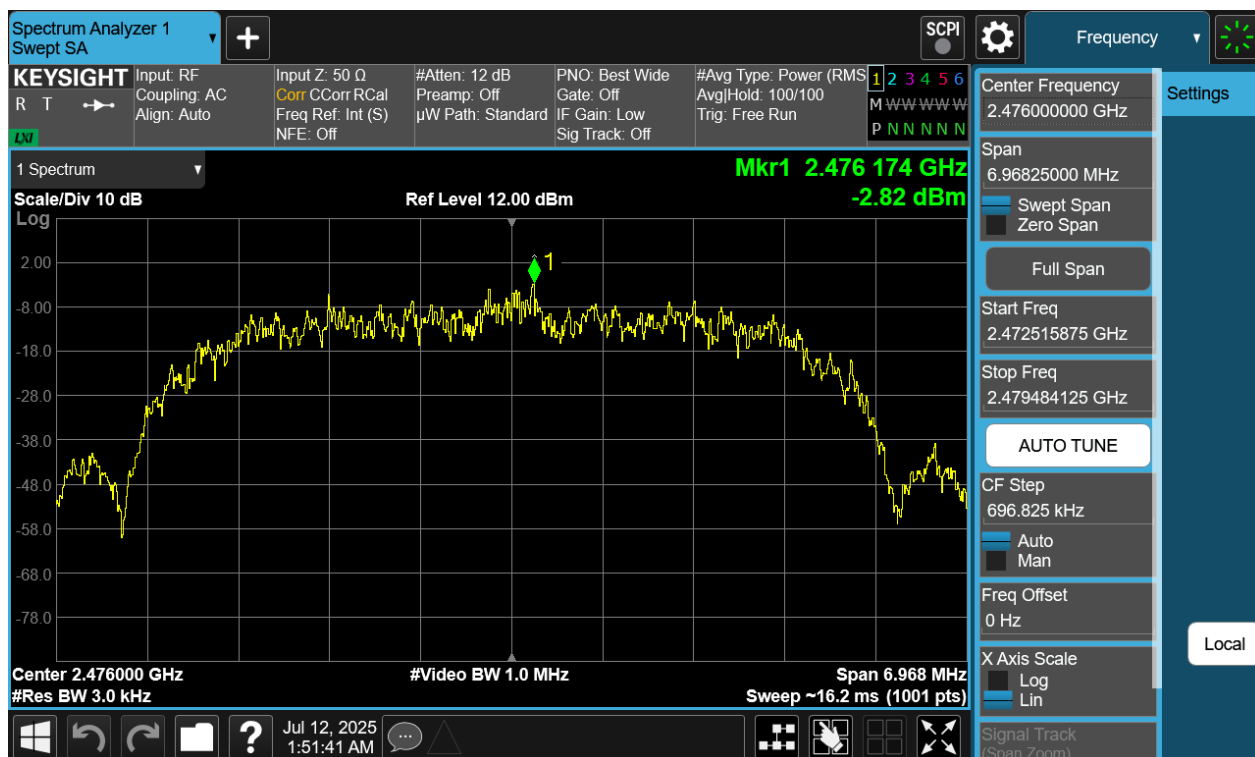
Plot 7-252. Power Spectral Density Plot Tx BF Diversity Antenna WF9 (Bluetooth (HDR8), 8Mbps, ePA – Ch. 73)
