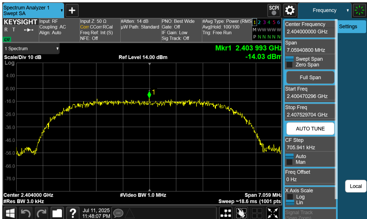
Plot 7-277. Power Spectral Density Plot Tx BF Diversity Antenna WF8 (Bluetooth (XHDRPM6), 6Mbps, iPA – Ch. 1)
