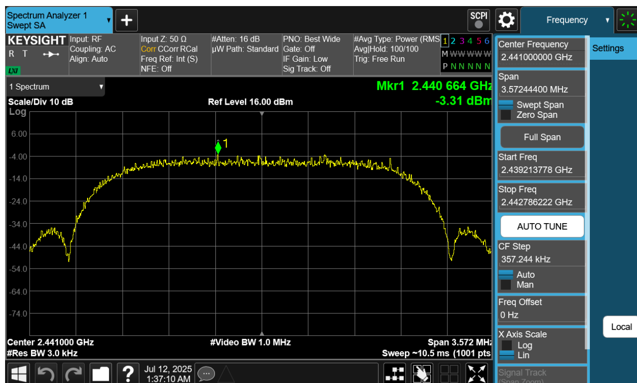
Plot 7-262. Power Spectral Density Plot Tx BF Diversity Antenna WF9 (Bluetooth (HDRPS2), 8Mbps, ePA – Ch. 38)
