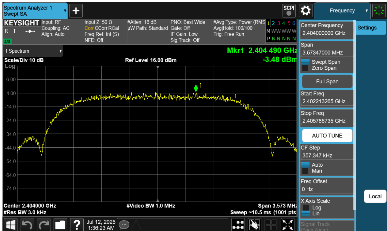
Plot 7-260. Power Spectral Density Plot TxBF Diversity Antenna WF9 (Bluetooth (HDRPS2), 8Mbps, ePA – Ch. 1)
