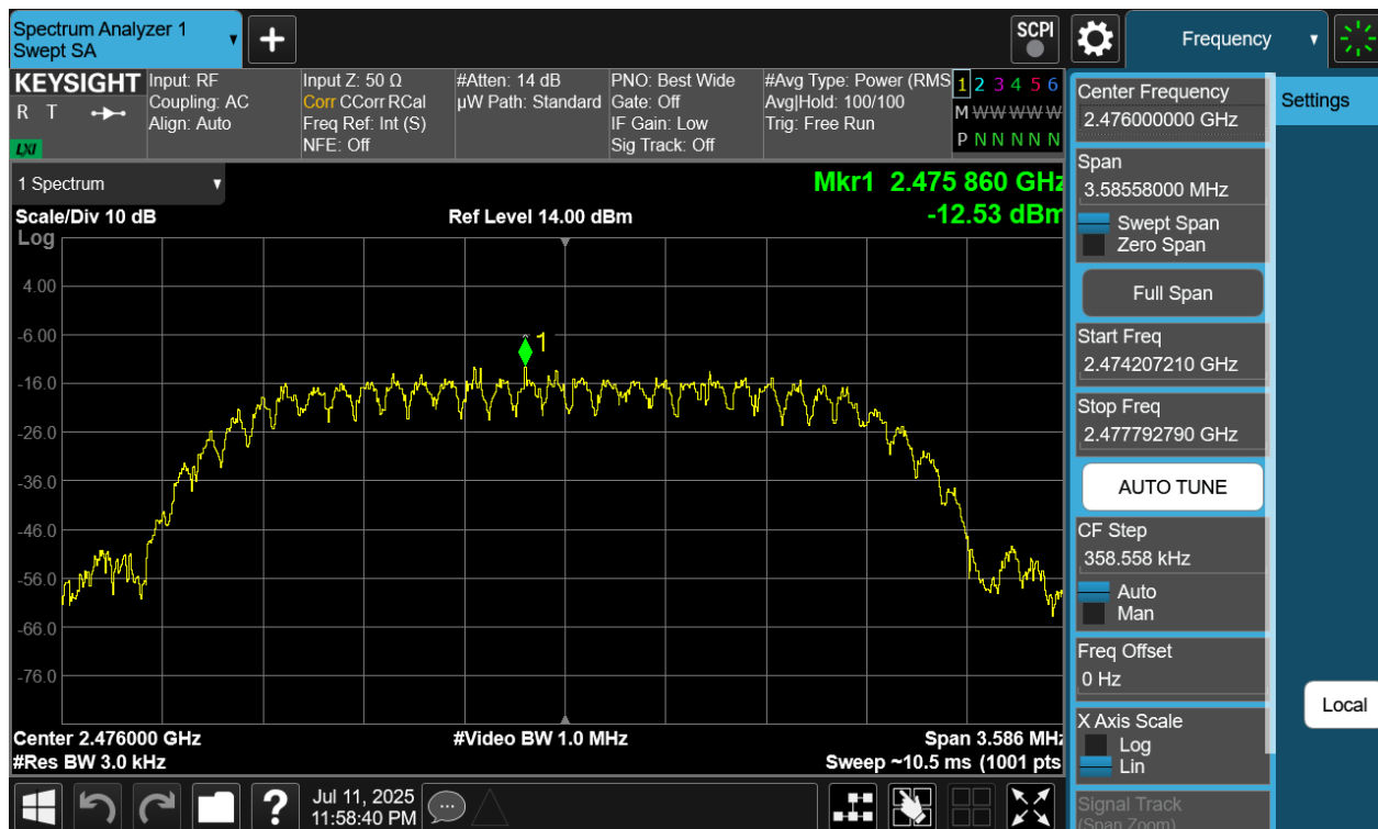
Plot 7-305. Power Spectral Density Plot Tx B Diversity Antenna WF8 (Bluetooth (HDT2), 2Mbps, iPA – Ch. 73)
