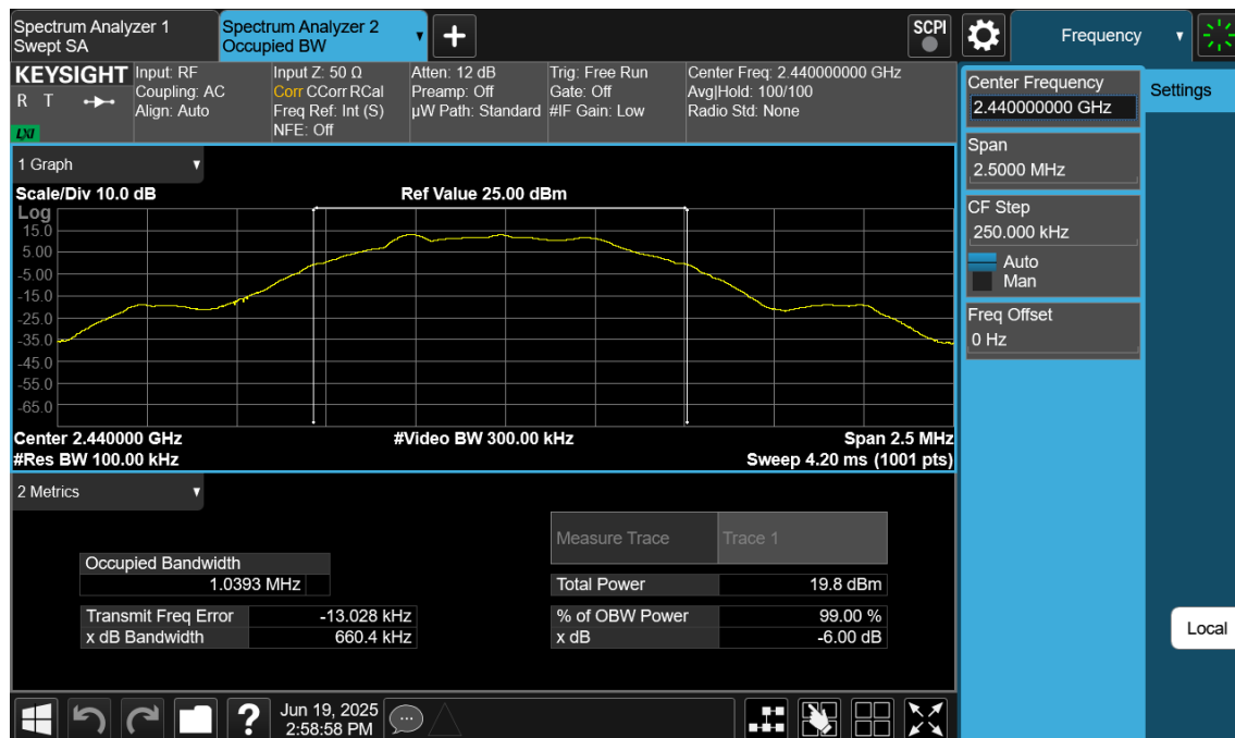
Plot 7-17.6dB BW & 99% OBW Plot Antenna WF7 (Bluetooth (LE), 500kbps, ePA – Ch. 19)
