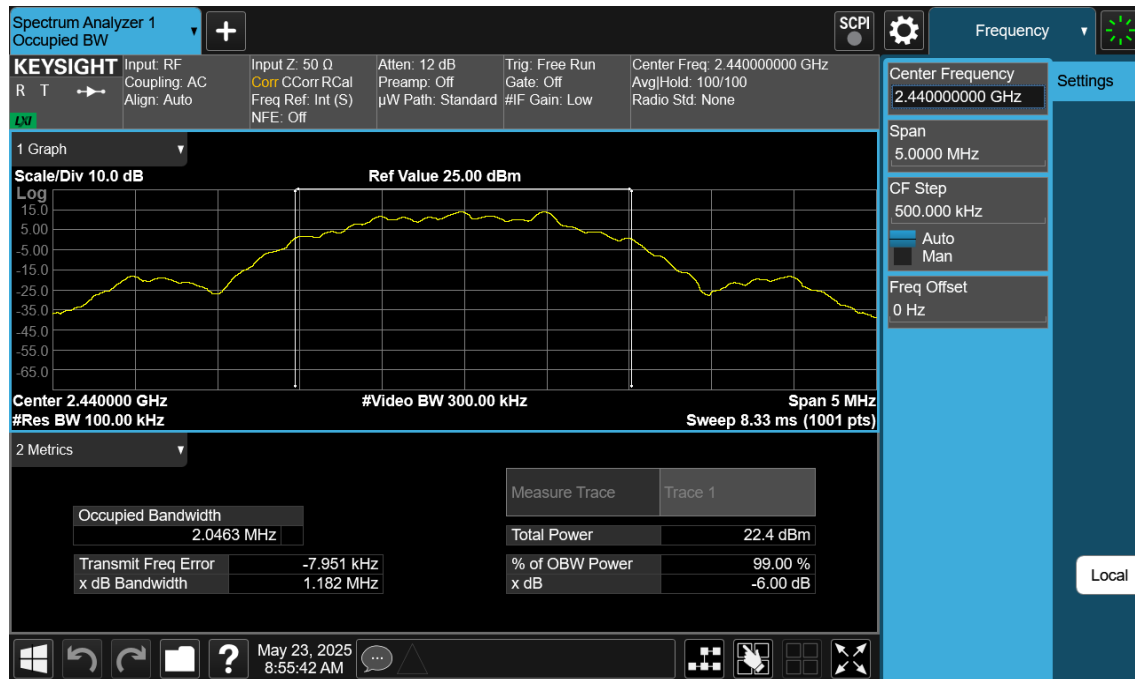
Plot 7-11. 6dB BW & 99% OBW Plot Antenna WF8 (Bluetooth (LE), 2Mbps, ePA – Ch. 19)
