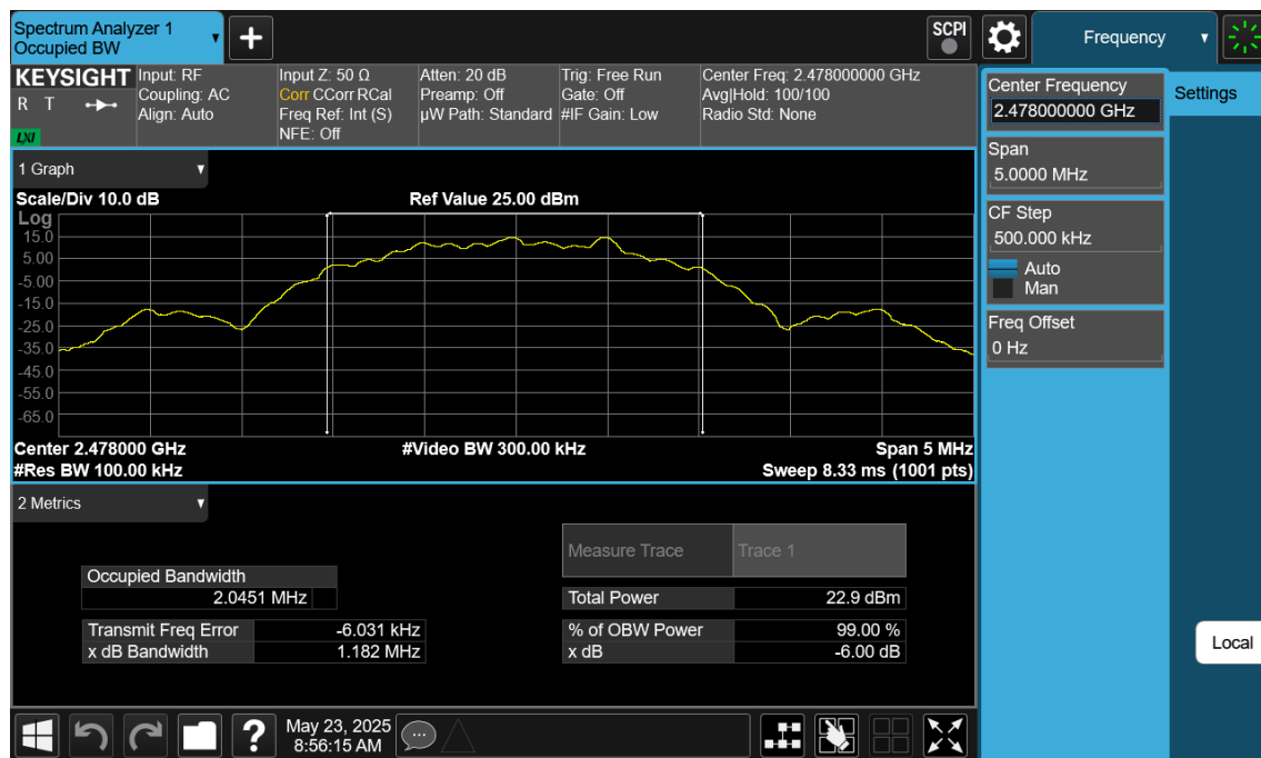
Plot 7-12. 6dB BW & 99% OBW Plot Antenna WF8 (Bluetooth (LE), 2Mbps, ePA – Ch. 38)
