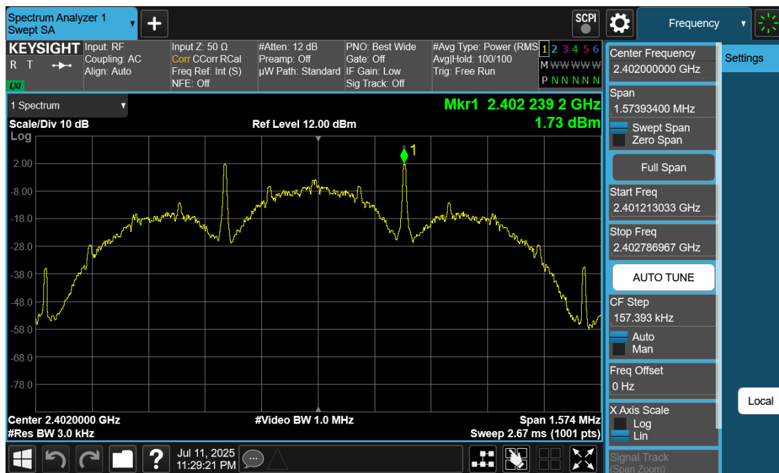
Plot 7-40. Power Spectral Density Plot Antenna WF8 (Bluetooth (LE), 125kbps, iPA – Ch. 0)
