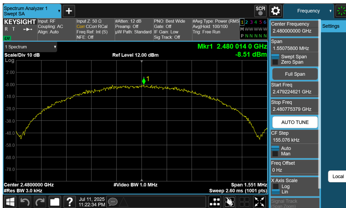
Plot 7-54. Power Spectral Density Plot Antenna WF8 (Bluetooth (LE), 1Mbps, iPA – Ch. 39)
