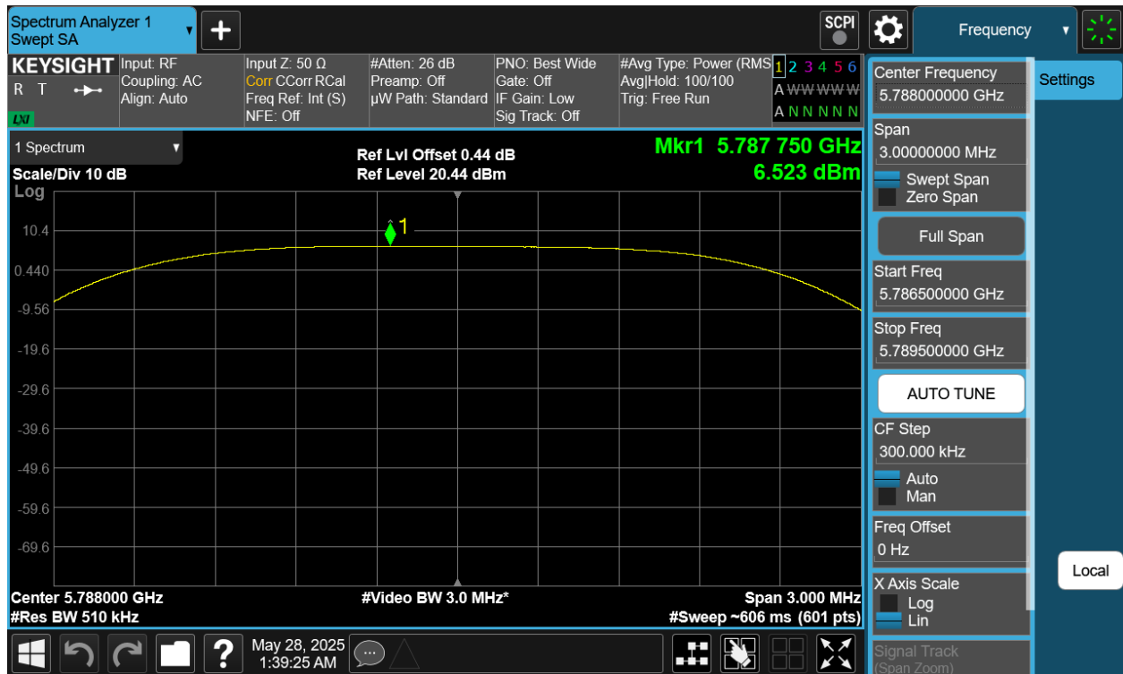
Plot 7-439. PSD TxBF Diversity Antenna WF8 (NB UNII HDT6, ePA – 5788MHz)
