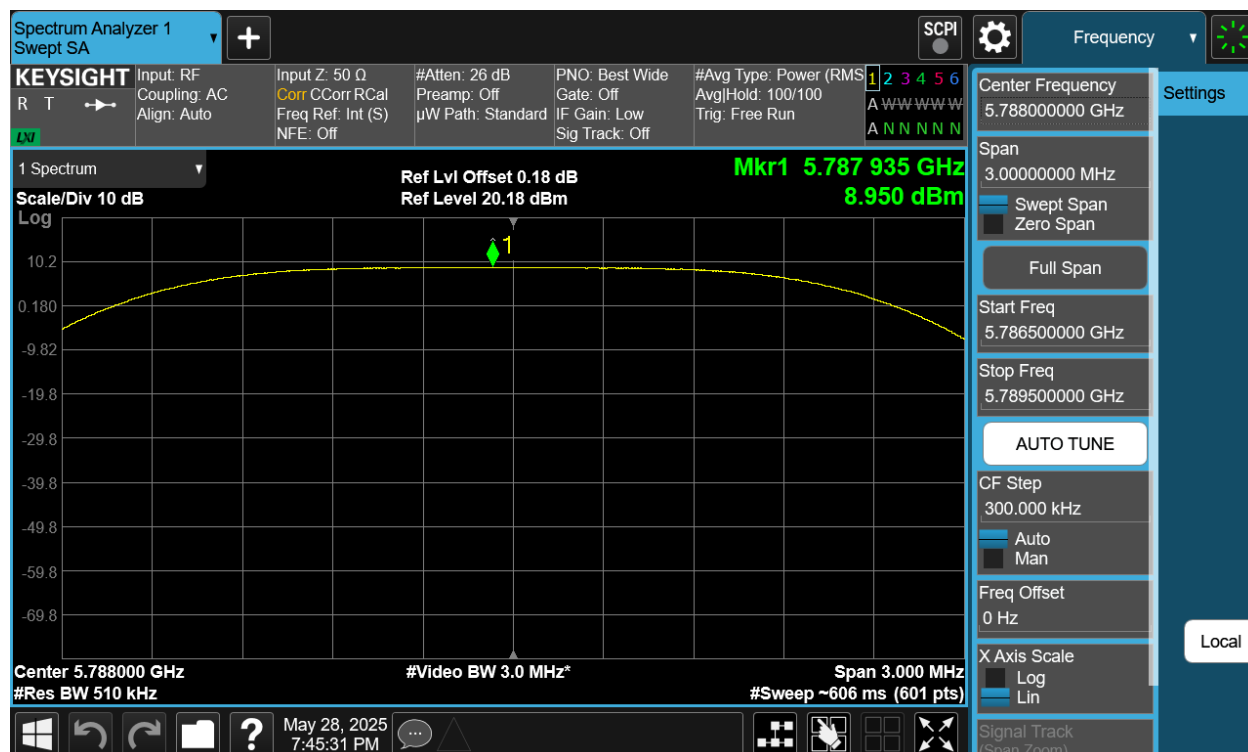
Plot 7-432. PSD TxBF Diversity Antenna WF7 (NB UNII HDT2, ePA – 5788MHz)
