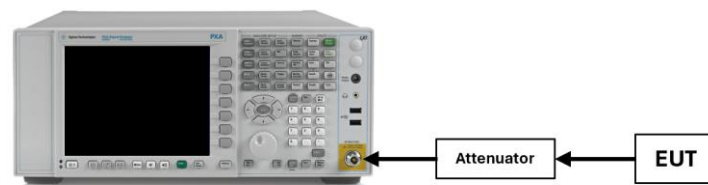
Figure 7-1. Test Instrument & Measurement Setup
