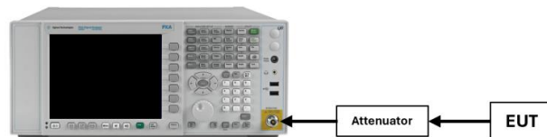
Figure 7-3. Test Instrument & Measurement Setup
