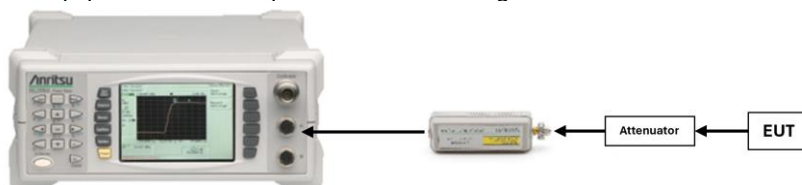
Figure 7-2. Test Instrument & Measurement Setup
