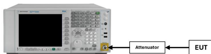
Figure 7-4. Test Instrument & Measurement Setup
