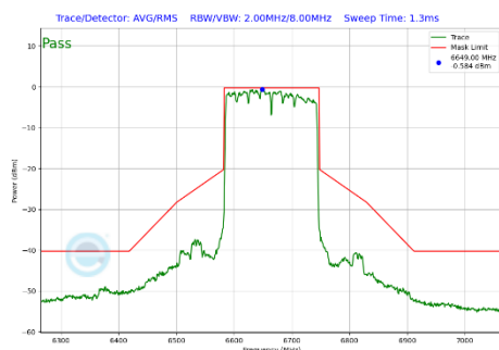
Plot 7-304 In-Band Emission Plot Antenna WF5B (160MHz BW 802.11be(SU) (UNII Band 7) - Ch.143)
