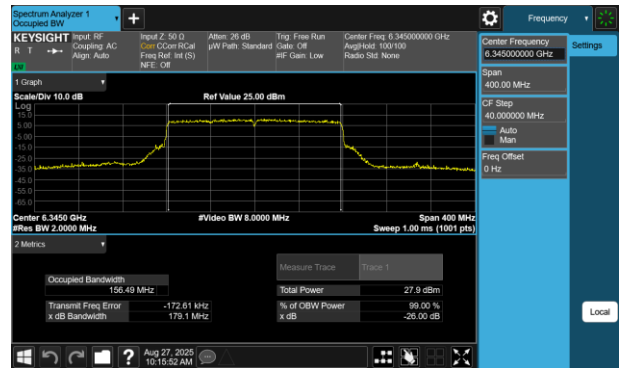
Plot 7-121 26dB BW & 99% OBW Antenna WF8 (160MHz BW 802.11be(RU) RU996X2 Index68 - Ch.79)
