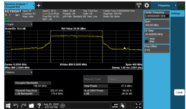
Plot 7-99 26dB BW & 99% OBW Antenna WF8 (160MHz BW 802.11be(RU) RU996X2 Index68 - Ch.111)
