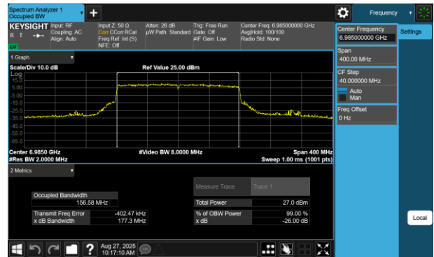
Plot 7-154 26dB BW & 99% OBW Antenna WF8 (160MHz BW 802.11be(RU) RU996X2 Index68 - Ch.207)
