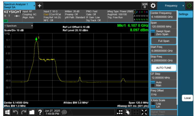
Plot 7-311 PSD Antenna WF8 (80MHz BW 802.11be(RU) RU26 Index0 - Ch.39)
