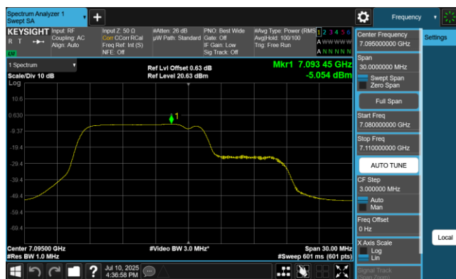
Plot 7-302 PSD Antenna WF5B (20MHz BW 802.11be(RU) RU106+26 Index82 - Ch.229)
