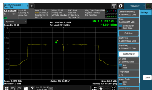
Plot 7-374 PSD SDM Diversity Antenna WF7 (160MHz BW 802.11be(RU) RU996X2 Index68 - Ch.47)
