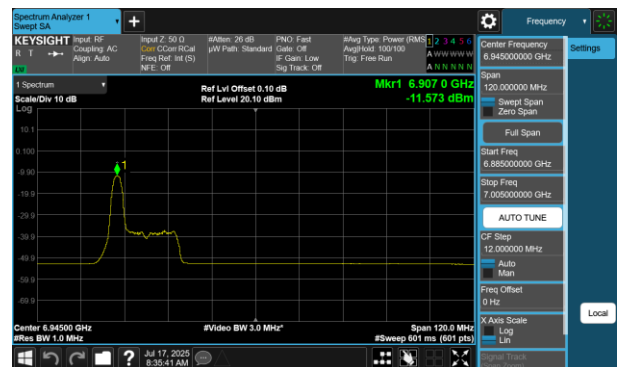
Plot 7-337 PSD SDM Primary Antenna WF8 (80MHz BW 802.11be(RU) RU26 Index0 - Ch.199)
