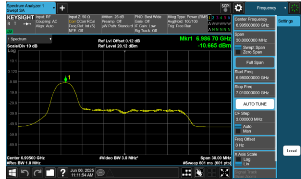
Plot 7-335 PSD SDM Primary Antenna WF8 (20MHz BW 802.11be(RU) RU26 Index0 - Ch.209)
