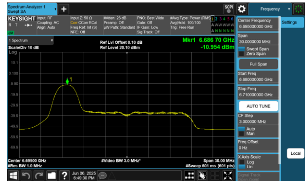
Plot 7-401 PSD SDM Diversity Antenna WF7 (20MHz BW 802.11be(RU) RU26 Index0 - Ch.149)
