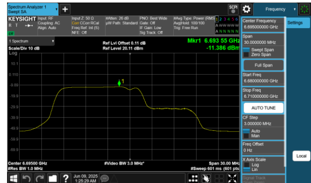
Plot 7-408 PSD SDM Diversity Antenna WF7 (20MHz BW 802.11be(RU) RU106+26 Index82 - Ch.149)
