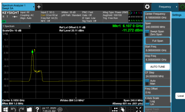
Plot 7-356 PSD SDM Diversity Antenna WF8 (160MHz BW 802.11be(RU) RU26 Index0 - Ch.47)
