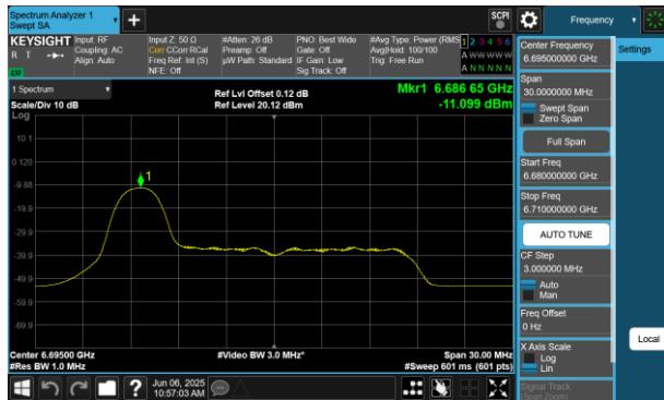
Plot 7-397 PSD SDM Diversity Antenna WF8 (20MHz BW 802.11be(RU) RU26 Index0 - Ch.149)
