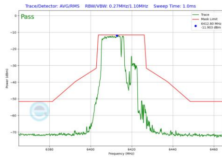
Plot 7-501 In-Band Emission Plot Antenna WF8 (20MHz BW 802.11be(RU) RU106+26 Index82 (UNII Band 5) - Ch.93)
