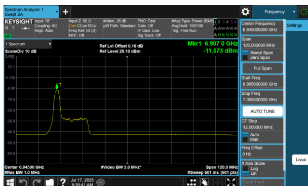
Plot 7-421 PSD SDM Diversity Antenna WF8 (80MHz BW 802.11be(RU) RU26 Index0 - Ch.199)
