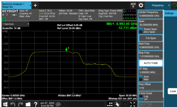
Plot 7-427 PSD SDM Diversity Antenna WF8 (20MHz BW 802.11be(RU) RU106+26 Index82 - Ch.209)
