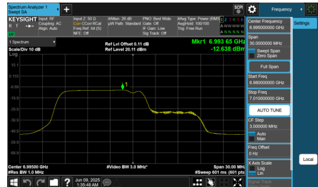
Plot 7-430 PSD SDM Diversity Antenna WF7 (20MHz BW 802.11be(RU) RU106+26 Index82 - Ch.209)
