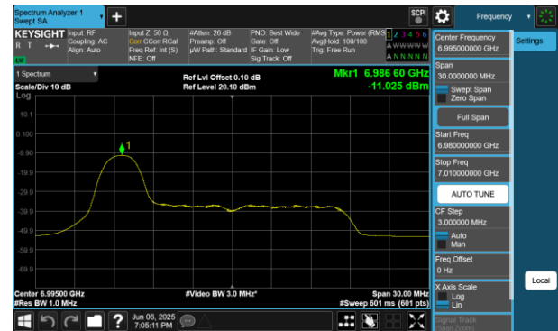
Plot 7-423 PSD SDM Diversity Antenna WF7 (20MHz BW 802.11be(RU) RU26 Index0 - Ch.209)
