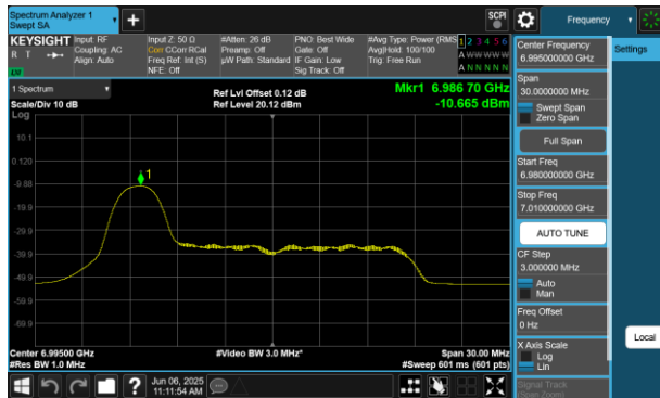
Plot 7-419 PSD SDM Diversity Antenna WF8 (20MHz BW 802.11be(RU) RU26 Index0 - Ch.209)
