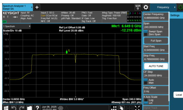
Plot 7-414 PSD SDM Diversity Antenna WF8 (160MHz BW 802.11be(RU) RU996X2 Index68 - Ch.143)
