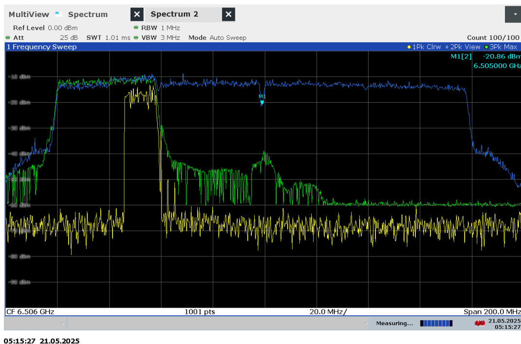
Plot 7-782. 160MHz Bandwidth, AWGN Signal Injected – 6505MHz
