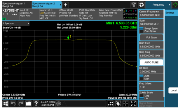
Plot 7-675 PSD CDD Diversity Antenna WF8 (20MHz BW 802.11be(RU) RU242 Index61 - Ch.117)
