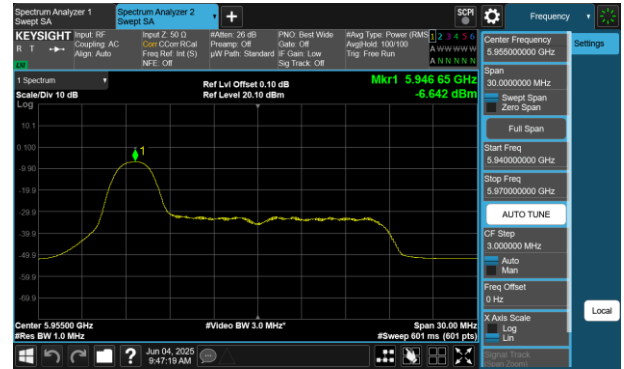
Plot 7-687 PSD CDD Diversity Antenna WF7 (20MHz BW 802.11be(RU) RU26 Index0 - Ch.1)
