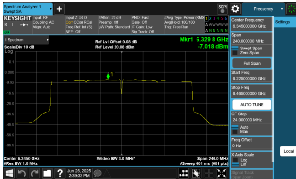
Plot 7-700 PSD CDD Diversity Antenna WF8 (160MHz BW 802.11be(RU) RU996X2 Index68 - Ch.79)
