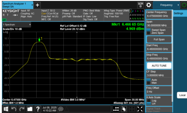
Plot 7-639 PSD CDD Diversity Antenna WF8 (20MHz BW 802.11be(RU) RU26 Index0 - Ch.105)
