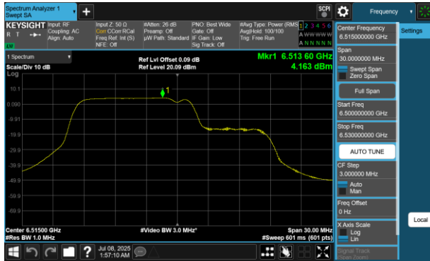
Plot 7-647 PSD CDD Diversity Antenna 1 (20MHz BW 802.11be(RU) RU106+26 Index82 - Ch.113)
