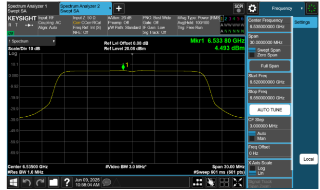
Plot 7-679 PSD CDD Diversity Antenna WF7 (20MHz BW 802.11be(RU) RU242 Index61 - Ch.117)
