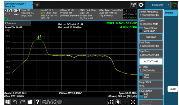
Plot 7-665 PSD CDD Diversity Antenna WF7 (20MHz BW 802.11be(RU) RU26 Index0 - Ch.117)
