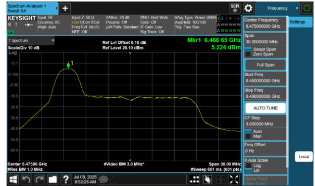
Plot 7-643 PSD CDD Diversity Antenna WF7 (20MHz BW 802.11be(RU) RU26 Index0 - Ch.105)
