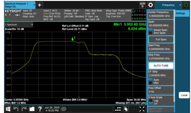
Plot 7-628 PSD SDM Diversity Antenna WF7 (20MHz BW 802.11be(RU) RU106+26 Index82 - Ch.1)
