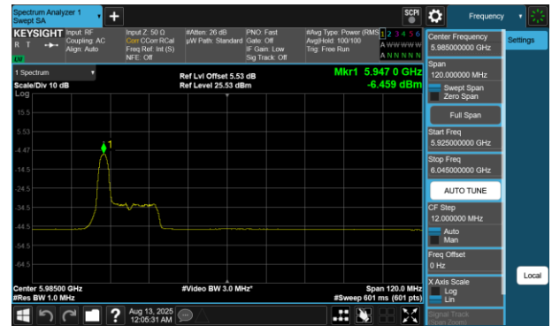
Plot 7-689 PSD CDD Diversity Antenna WF7 (80MHz BW 802.11be(RU) RU26 Index0 - Ch.7)
