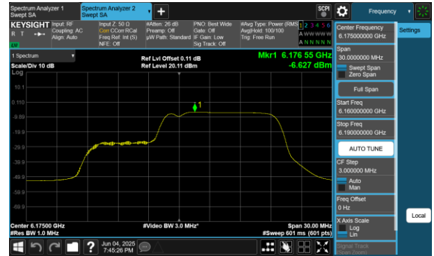
Plot 7-694 PSD CDD Diversity Antenna WF7 (20MHz BW 802.11be(RU) RU106+26 Index83 - Ch.45)
