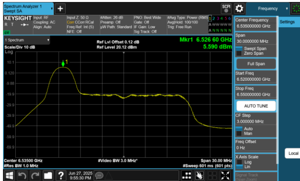
Plot 7-661 PSD CDD Diversity Antenna WF8 (20MHz BW 802.11be(RU) RU26 Index0 - Ch.117)
