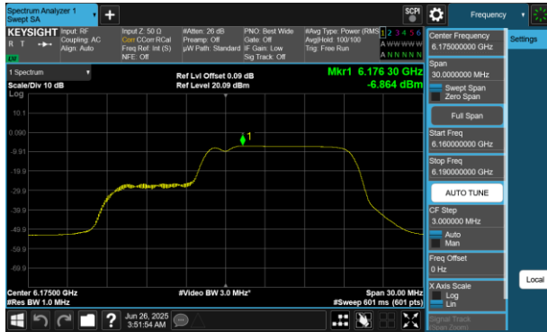
Plot 7-691 PSD CDD Diversity Antenna 1 (20MHz BW 802.11be(RU) RU106+26 Index83 - Ch.45)
