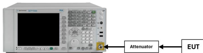
Figure 7-1. Test Instrument & Measurement Setup
