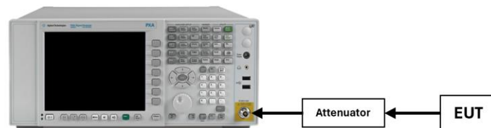
Figure 7-3. Test Instrument & Measurement Setup
