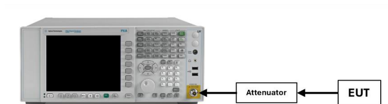
Figure 7-1. Test Instrument & Measurement Setup
