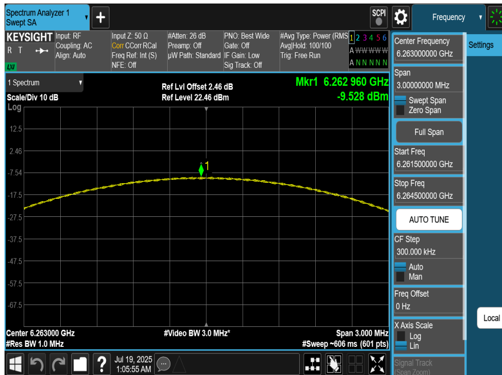
Plot 7-70. PSD Antenna 4a (NB UNII LE2M, ePA – 6263MHz)
