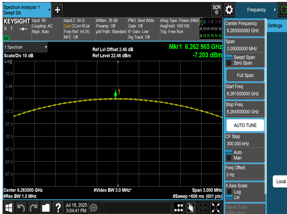
Plot 7-96. PSD Antenna 2a (NB UNII LE2M, ePA – 6263MHz)
