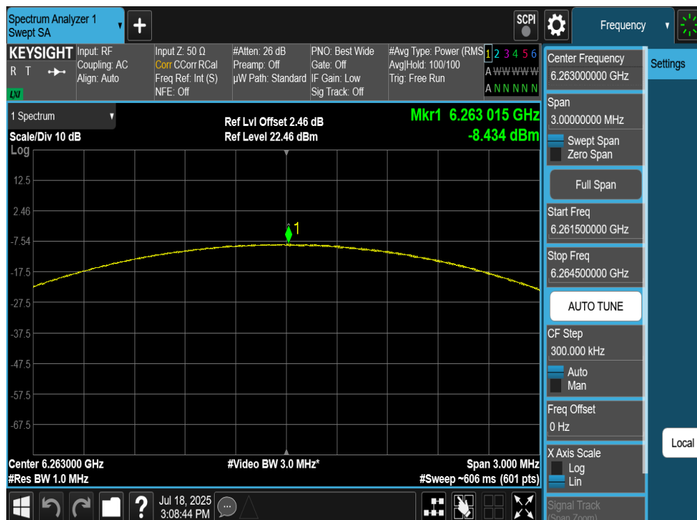
Plot 7-97. PSD Antenna 2a (NB UNII LE2M, iPA – 6263MHz)
