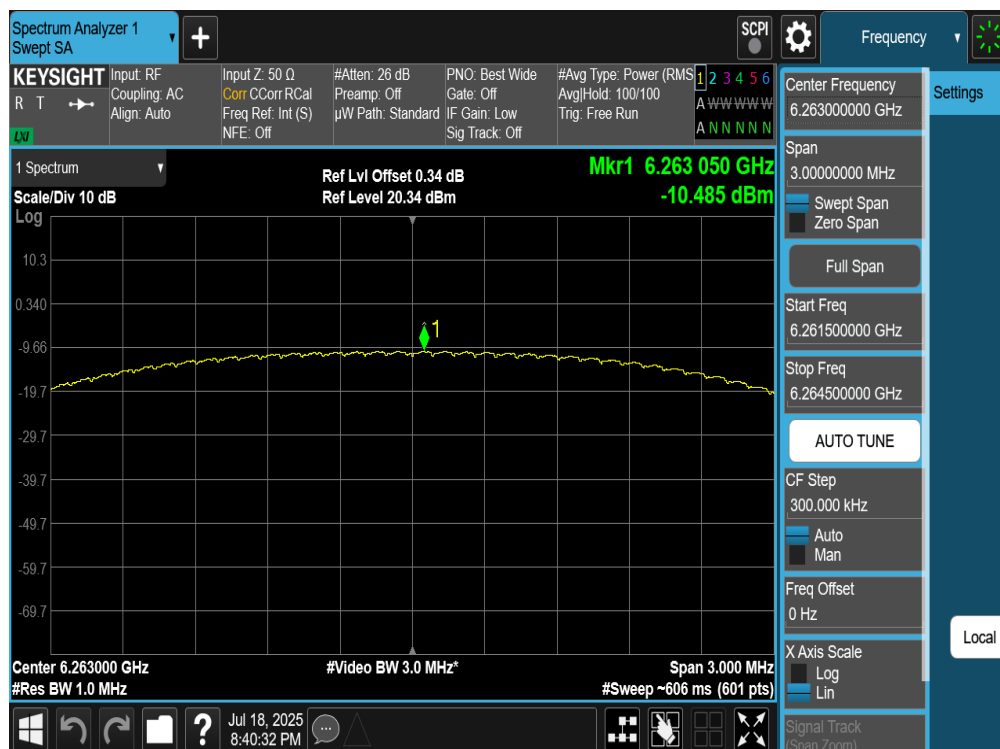
Plot 7-103. PSD Antenna 2a (NB UNII HDRPS2, iPA – 6263MHz)
