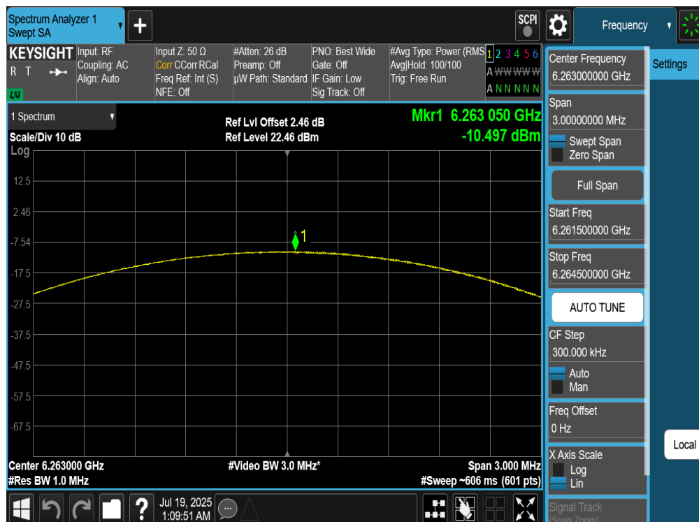
Plot 7-71. PSD Antenna 4a (NB UNII LE2M, iPA – 6263MHz)
