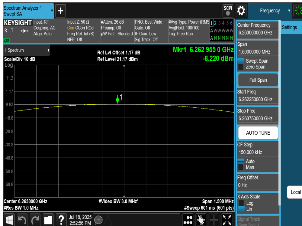
Plot 7-93. PSD Antenna 2a (NB UNII BDR, iPA – 6263MHz)
