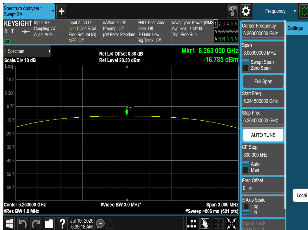
Plot 7-163. PSD Tx BF Primary Antenna 4a (NB UNII HDT4, ePA – 6263MHz)
