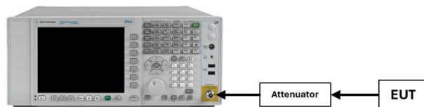
Figure 7-4. Test Instrument & Measurement Setup
