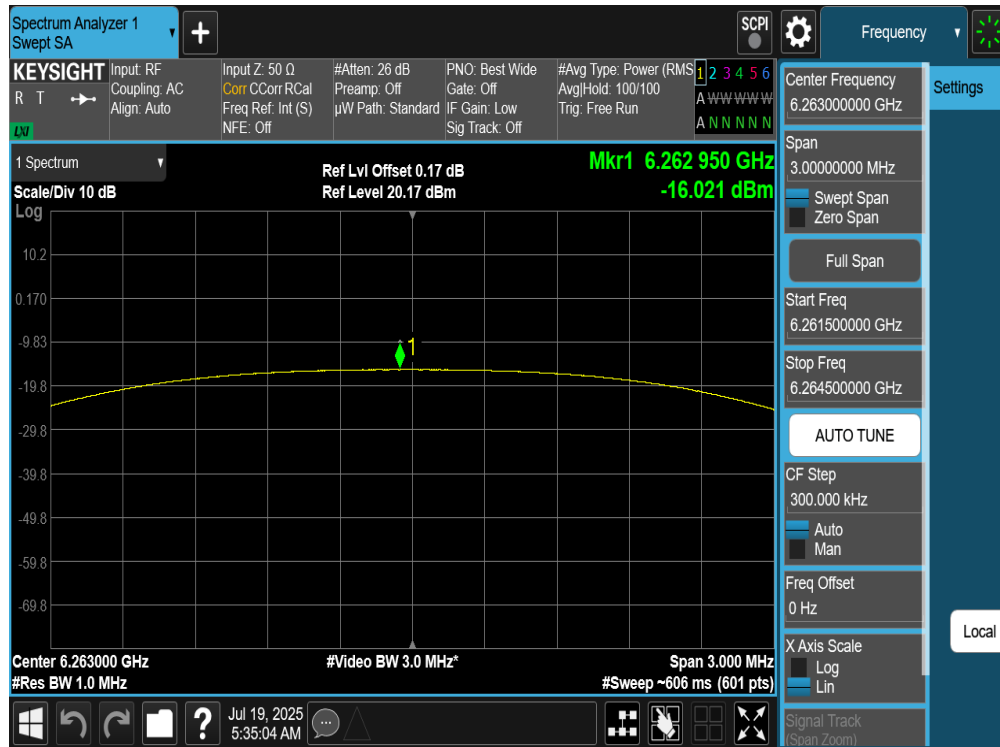
Plot 7-212. PSD Tx BF Diversity Antenna 4a (NB UNII HDT2, iPA – 6263MHz)
