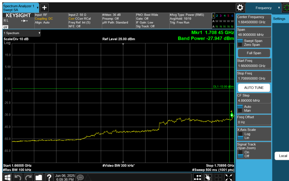
Plot 7-330. Lower Extended Band Edge Plot (NR Band n66 – 20.0MHz DFT-s-OFDM QPSK - Full RB)
