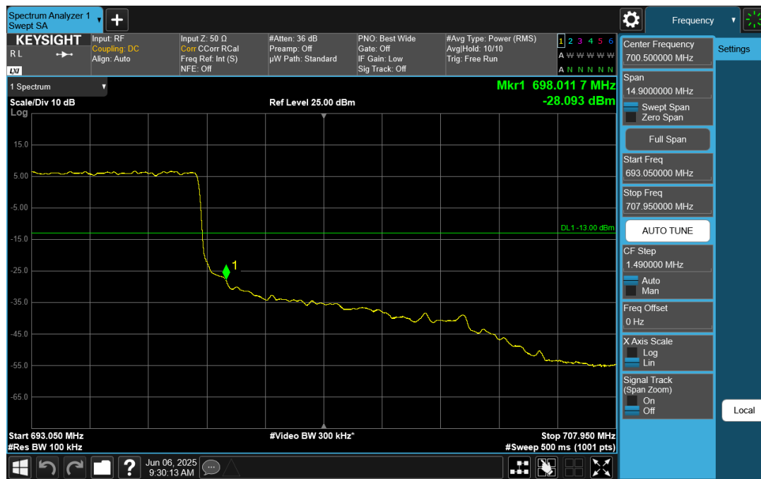
Plot 7-368. Upper Band Edge Plot (NR Band n71 – 10.0MHz DFT-s-OFDM QPSK - Full RB)
