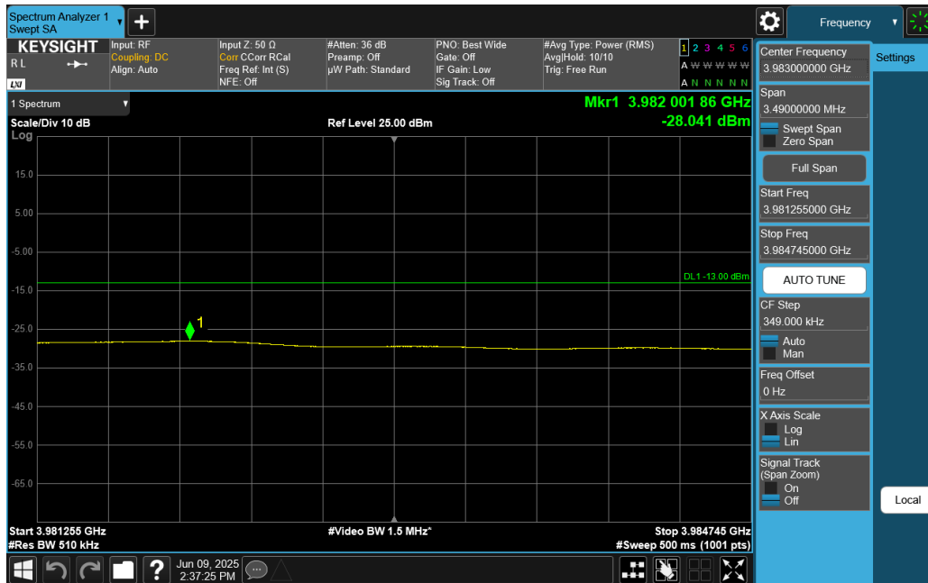
Plot 7-221. Extended Upper Band Edge Plot (NR Band n77 C-Band - 15MHz DFT-s-OFDM QPSK – Full RB)
