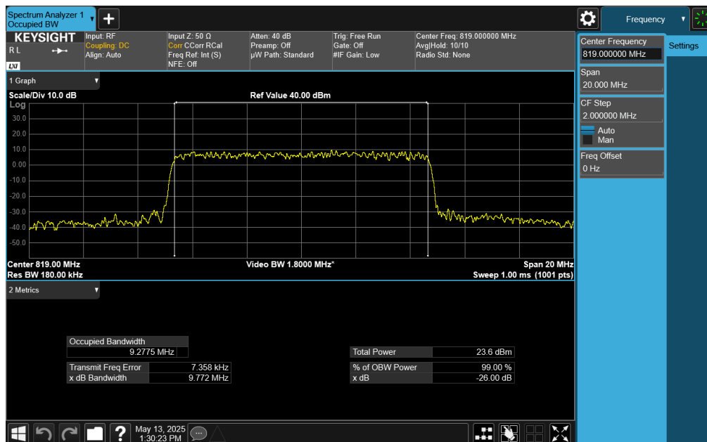
Plot 7-32. Occupied Bandwidth Plot (NR Band n26 - 10MHz CP-OFDM 16-QAM - Full RB)
