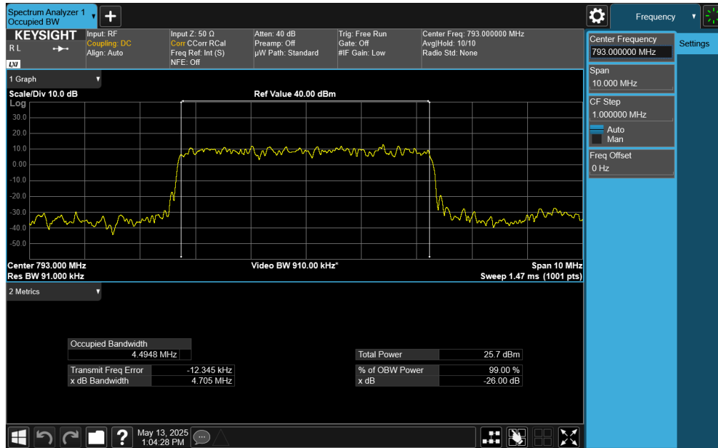
Plot 7-35. Occupied Bandwidth Plot (NR Band n14 - 5MHz DFT-s-OFDM \pi/2 BPSK - Full RB)
