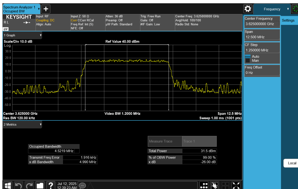
Plot 7-1. Occupied Bandwidth Plot (LTE Band 48 - 5MHz QPSK - Full RB Configuration)
