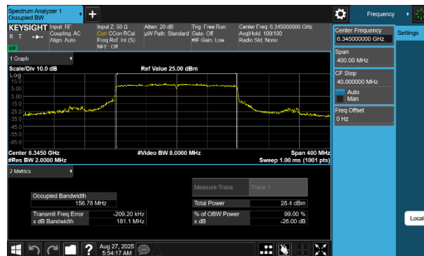
Plot 7-32 26dB BW & 99% OBW Antenna 4a (160MHz BW 802.11be(SU) - Ch.79)
