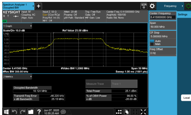
Plot 7-29 26dB BW & 99% OBW Antenna 4a (20MHz BW 802.11a - Ch.93)
