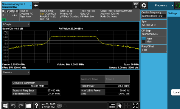
Plot 7-9 26dB BW & 99% OBW Antenna WF5B (20MHz BW 802.11a - Ch.181)
