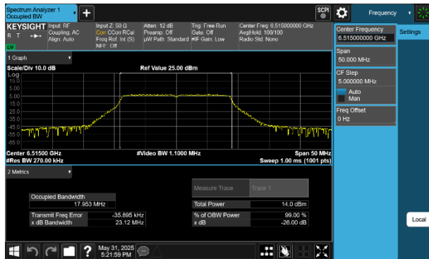
Plot 7-17 26dB BW & 99% OBW Antenna WF5B (20MHz BW 802.11a - Ch.113)
