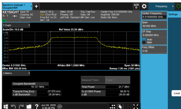
Plot 7-5 26dB BW & 99% OBW Antenna WF5B (20MHz BW 802.11a - Ch.113)
