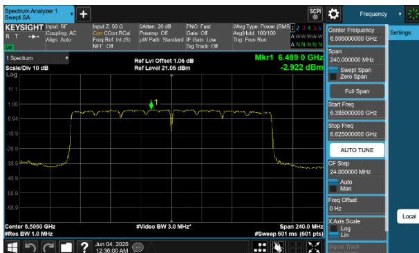
Plot 7-180 PSD CDD Primary Antenna WF5B (160MHz BW 802.11be(SU) - Ch.111)
