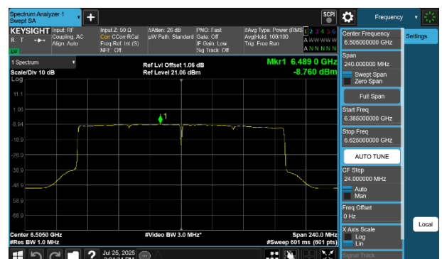
Plot 7-208 PSD SDM Primary Antenna 4a (160MHz BW 802.11be(SU) - Ch.111)
