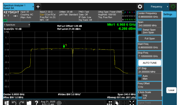
Plot 7-224 PSD SDM Primary Antenna 4a (160MHz BW 802.11be(SU) - Ch.207)
