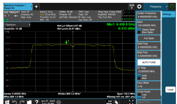
Plot 7-183 PSD CDD Primary Antenna 4a (80MHz BW 802.11be(SU) - Ch.103)
