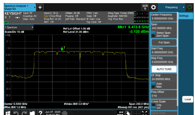
Plot 7-184 PSD CDD Primary Antenna 4a (160MHz BW 802.11be(SU) - Ch.111)
