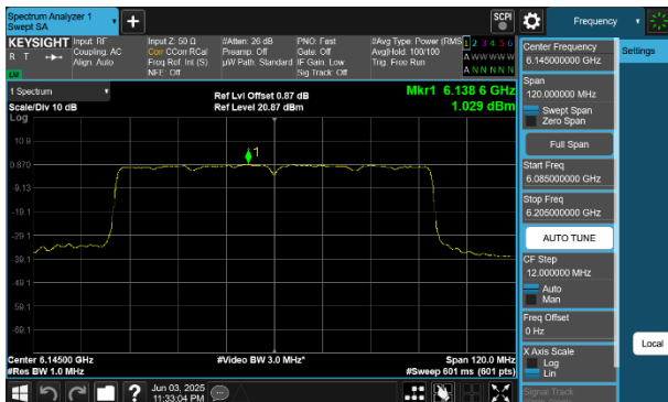
Plot 7-171 PSD CDD Primary Antenna WF5B (80MHz BW 802.11be(SU) - Ch.39)
