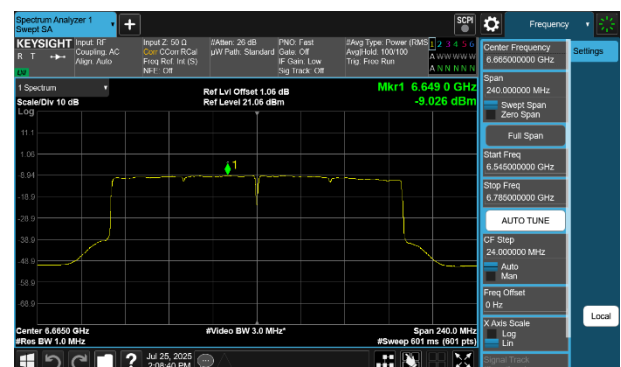
Plot 7-216 PSD SDM Primary Antenna 4a (160MHz BW 802.11be(SU) - Ch.143)
