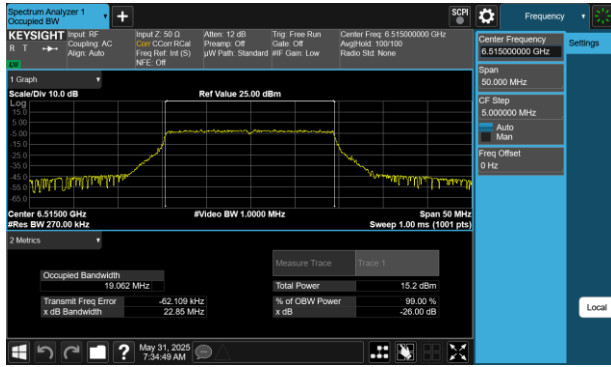
Plot 7-52 26dB BW & 99% OBW Antenna WF5B (20MHz BW 802.11be(RU) RU242 Index61 - Ch.113)
