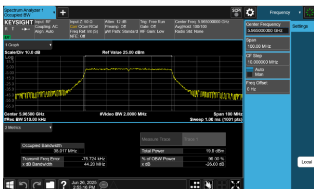
Plot 7-42 26dB BW & 99% OBW Antenna WF5B (40MHz BW 802.11be(RU) RU484 Index65 - Ch.3)
