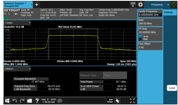
Plot 7-54 26dB BW & 99% OBW Antenna WF5B (80MHz BW 802.11be(RU) RU996 Index67 - Ch.103)
