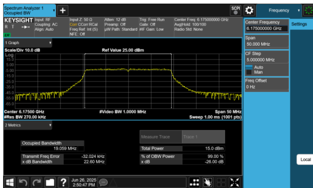
Plot 7-41 26dB BW & 99% OBW Antenna WF5B (20MHz BW 802.11be(RU) RU242 Index61 - Ch.45)
