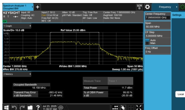
Plot 7-71 26dB BW & 99% OBW Antenna WF5B (20MHz BW 802.11be(RU) RU106+26 Index82 - Ch.229)
