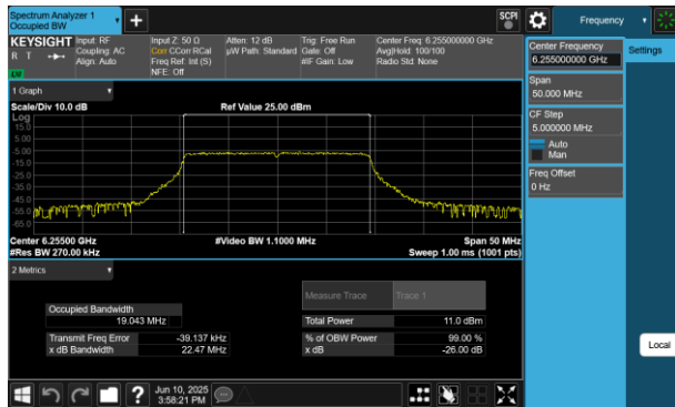
Plot 7-96 26dB BW & 99% OBW Antenna 2a (20MHz BW 802.11be(RU) RU242 Index61 - Ch.61)
