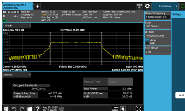
Plot 7-119 26dB BW & 99% OBW Antenna 2a (40MHz BW 802.11be(RU) RU484 Index65 - Ch.123)
