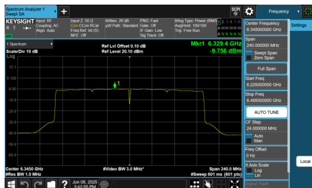
Plot 7-143 PSD Antenna WF5B (160MHz BW 802.11be(RU) RU996X2 Index68 - Ch.79)
