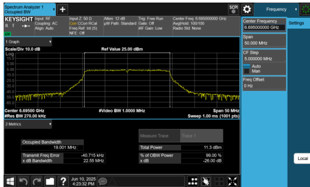
Plot 7-118 26dB BW & 99% OBW Antenna 2a (20MHz BW 802.11be(RU) RU242 Index61 - Ch.149)
