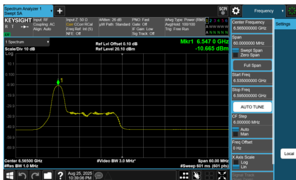
Plot 7-244 PSD Antenna 2a (40MHz BW 802.11be(RU) RU26 Index0 - Ch.123)
