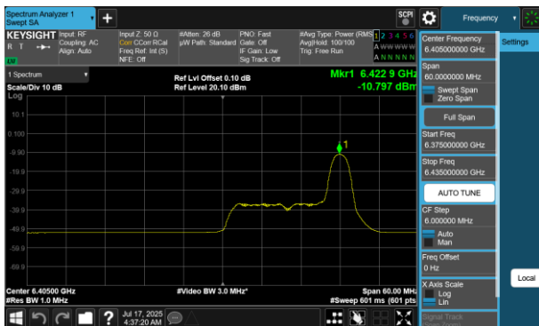
Plot 7-266 PSD SDM Primary Antenna WF5B (40MHz BW 802.11be(RU) RU26 Index17 - Ch.91)
