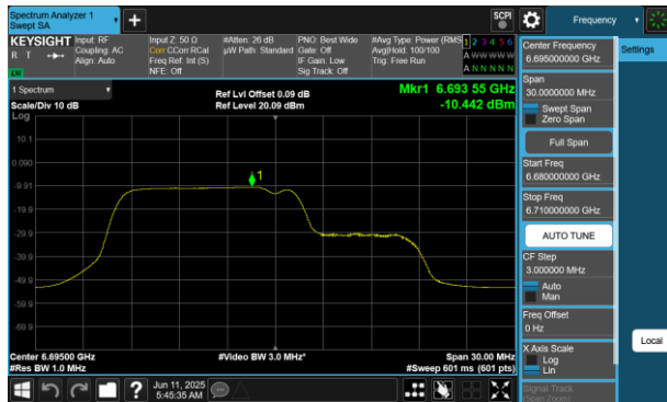
Plot 7-247 PSD Antenna 2a (20MHz BW 802.11be(RU) RU106+26 Index82 - Ch.149)
