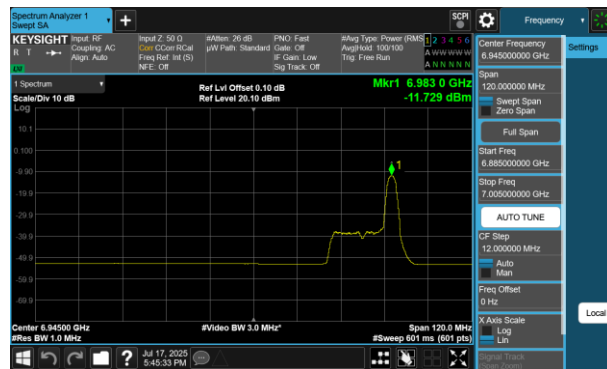
Plot 7-256 PSD Antenna 2a (80MHz BW 802.11be(RU) RU26 Index36 - Ch.199)
