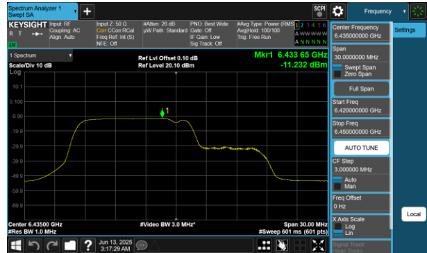
Plot 7-298 PSD SDM Primary Antenna 4a (20MHz BW 802.11be(RU) RU106+26 Index82 - Ch.97)
