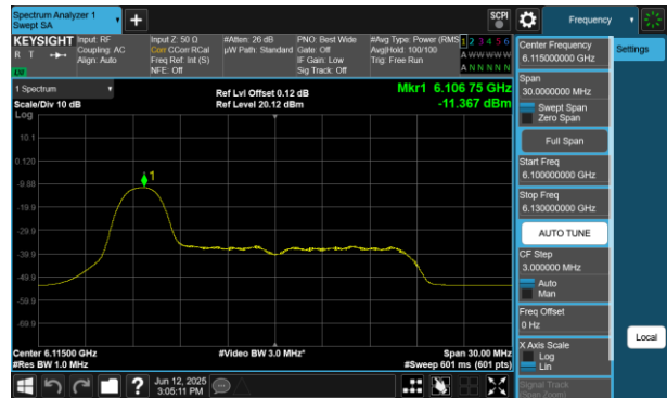
Plot 7-269 PSD SDM Primary Antenna 4a (20MHz BW 802.11be(RU) RU26 Index0 - Ch.33)
