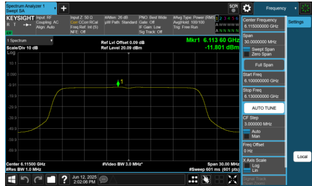
Plot 7-283 PSD SDM Primary Antenna 4a (20MHz BW 802.11be(RU) RU242 Index61 - Ch.33)
