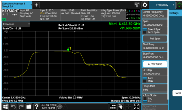
Plot 7-295 PSD SDM Primary Antenna WF5B (20MHz BW 802.11be(RU) RU106+26 Index82 - Ch.97)
