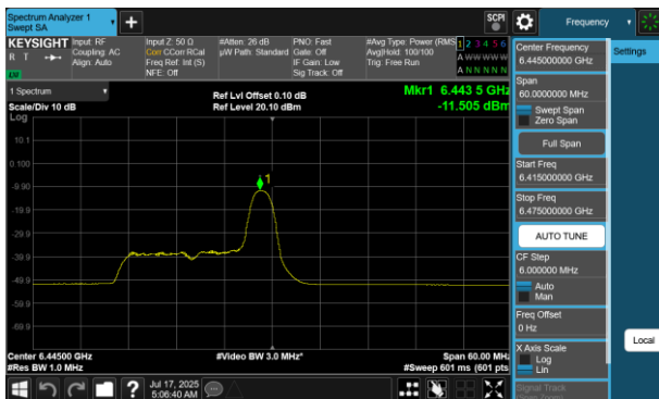
Plot 7-288 PSD SDM Primary Antenna WF5B (40MHz BW 802.11be(RU) RU26 Index8 - Ch.99)
