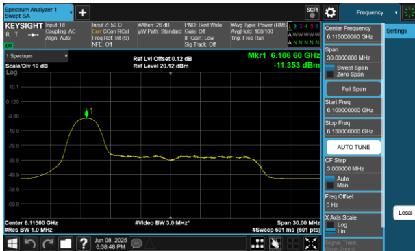
Plot 7-265 PSD SDM Primary Antenna WF5B (20MHz BW 802.11be(RU) RU26 Index0 - Ch.33)
