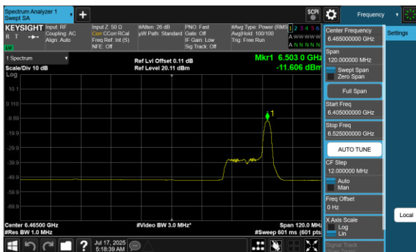
Plot 7-289 PSD SDM Primary Antenna WF5B (80MHz BW 802.11be(RU) RU26 Index36 - Ch.103)
