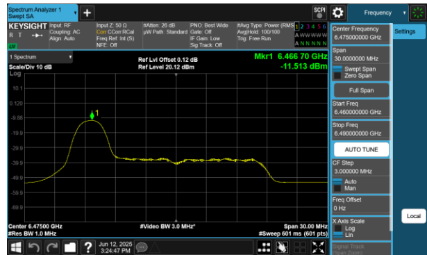
Plot 7-291 PSD SDM Primary Antenna 4a (20MHz BW 802.11be(RU) RU26 Index0 - Ch.105)
