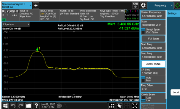
Plot 7-287 PSD SDM Primary Antenna WF5B (20MHz BW 802.11be(RU) RU26 Index0 - Ch.105)
