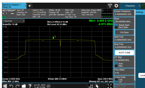
Plot 7-286 PSD Antenna WF5B (160MHz BW 802.11be(RU) RU996X2 Index68 - Ch.111)
