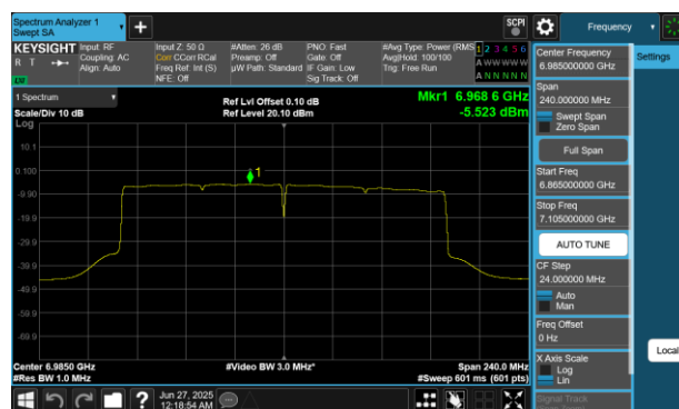
Plot 7-308 PSD Antenna WF5B (160MHz BW 802.11be(RU) RU996X2 Index68 - Ch.207)
