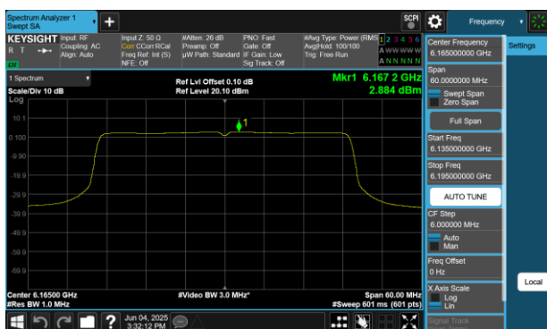
Plot 7-240 PSD Antenna WF5B (40MHz BW 802.11be(RU) RU484 Index65 - Ch.43)
