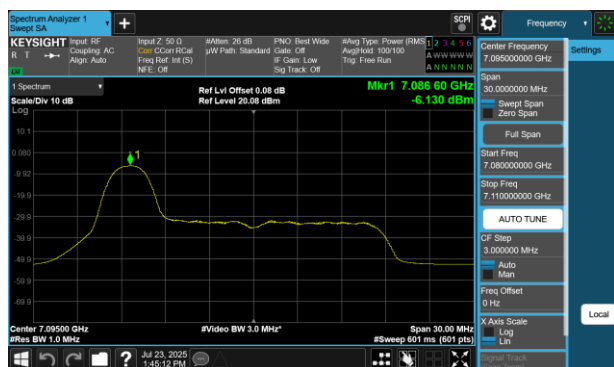
Plot 7-298 PSD Antenna WF5B (20MHz BW 802.11be(RU) RU26 Index0 - Ch.229)
