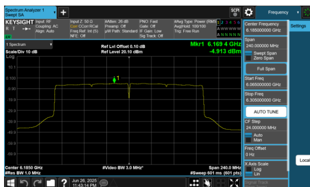
Plot 7-275 PSD Antenna WF5B (160MHz BW 802.11be(RU) RU996X2 Index68 - Ch.47)
