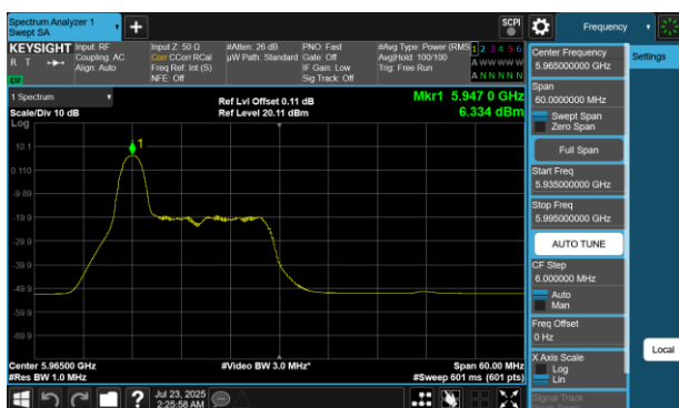
Plot 7-310 PSD Antenna 4a (40MHz BW 802.11be(RU) RU26 Index0 - Ch.3)
