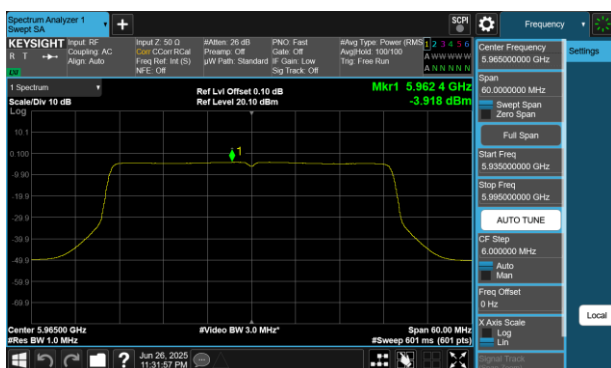
Plot 7-273 PSD Antenna WF5B (40MHz BW 802.11be(RU) RU484 Index65 - Ch.3)
