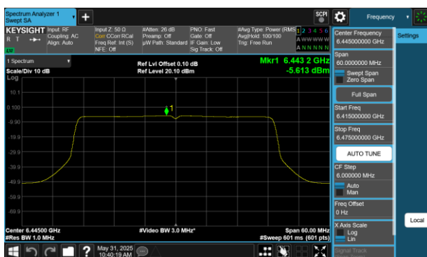
Plot 7-284 PSD Antenna WF5B (40MHz BW 802.11be(RU) RU484 Index65 - Ch.99)
