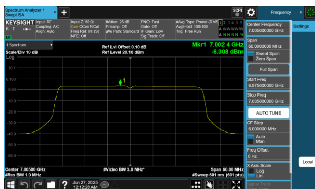
Plot 7-306 PSD Antenna WF5B (40MHz BW 802.11be(RU) RU484 Index65 - Ch.211)
