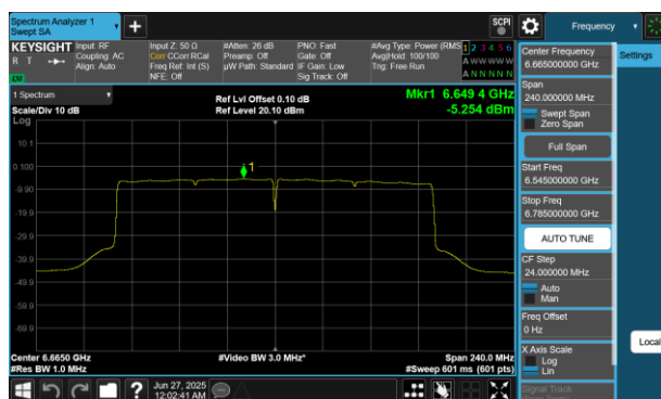
Plot 7-297 PSD Antenna WF5B (160MHz BW 802.11be(RU) RU996X2 Index68 - Ch.143)
