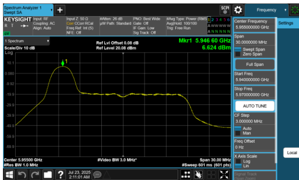
Plot 7-309 PSD Antenna 4a (20MHz BW 802.11be(RU) RU26 Index0 - Ch.1)
