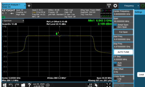
Plot 7-262 PSD Antenna WF5B (40MHz BW 802.11be(RU) RU484 Index65 - Ch.179)
