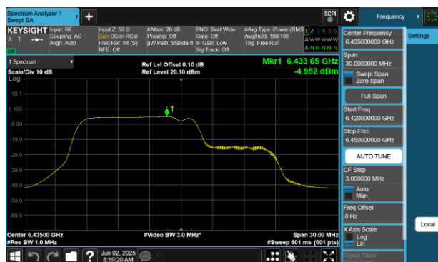
Plot 7-280 PSD Antenna WF5B (20MHz BW 802.11be(RU) RU106+26 Index82 - Ch.97)
