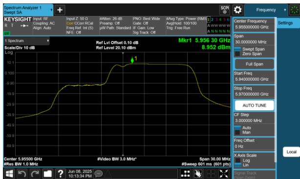
Plot 7-313 PSD Antenna 4a (20MHz BW 802.11be(RU) RU106+26 Index83 - Ch.1)
