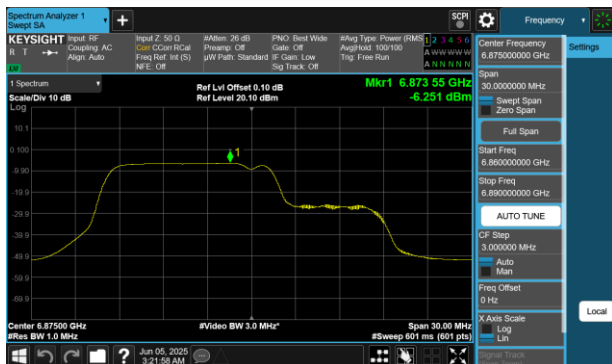
Plot 7-368 PSD Antenna 4a (20MHz BW 802.11be(RU) RU106+26 Index82 - Ch.185)
