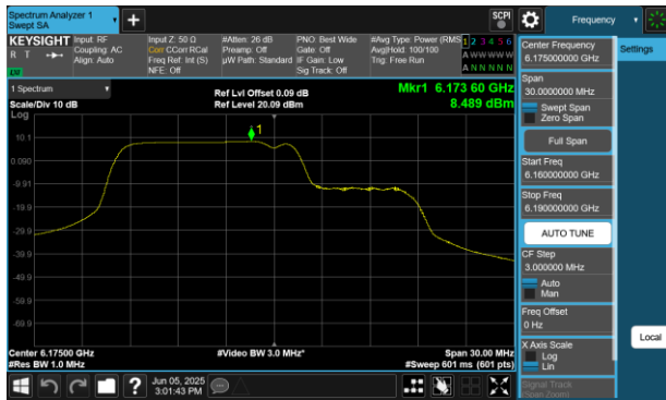
Plot 7-390 PSD Antenna 2a (20MHz BW 802.11be(RU) RU106+26 Index82 - Ch.45)
