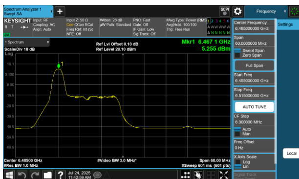
Plot 7-398 PSD Antenna 2a (40MHz BW 802.11be(RU) RU26 Index0 - Ch.107)
