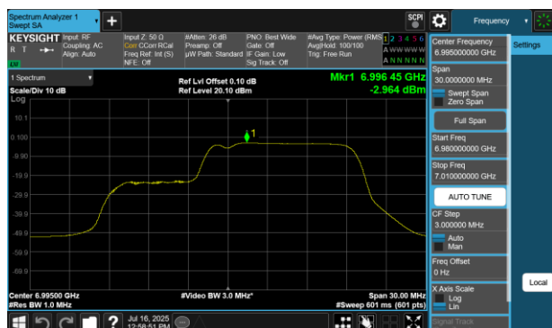
Plot 7-379 PSD Antenna 4a (20MHz BW 802.11be(RU) RU106+26 Index83 - Ch.209)
