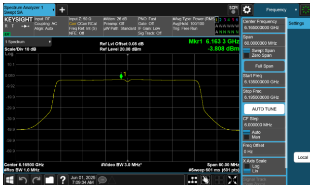
Plot 7-350 PSD Antenna 4a (40MHz BW 802.11be(RU) RU484 Index65 - Ch.43)
