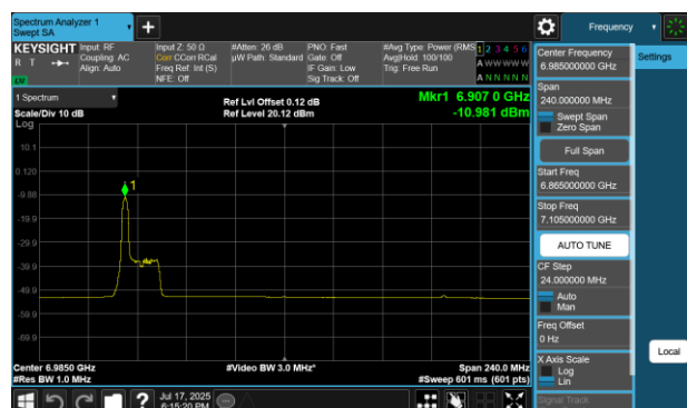
Plot 7-426 PSD SDM Diversity Antenna 2a (160MHz BW 802.11be(RU) RU26 Index0 - Ch.207)
