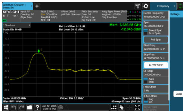
Plot 7-397 PSD SDM Diversity Antenna 4a (20MHz BW 802.11be(RU) RU26 Index0 - Ch.149)
