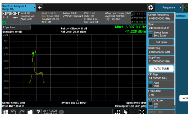
Plot 7-422 PSD SDM Diversity Antenna 4a (160MHz BW 802.11be(RU) RU26 Index0 - Ch.207)
