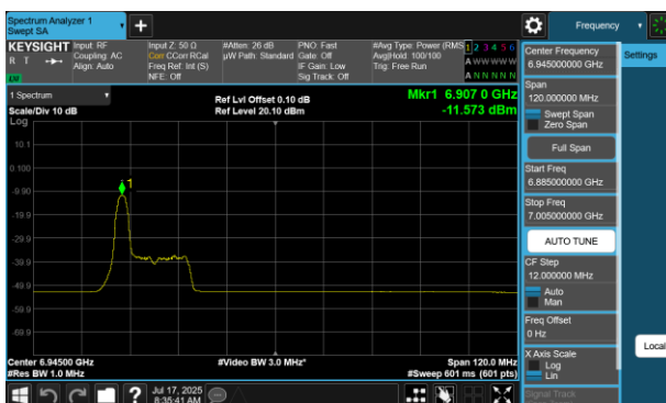
Plot 7-421 PSD SDM Diversity Antenna 4a (80MHz BW 802.11be(RU) RU26 Index0 - Ch.199)
