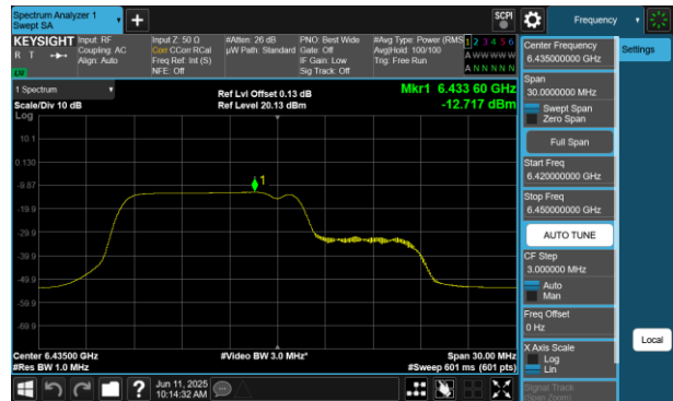
Plot 7-386 PSD SDM Diversity Antenna 2a (20MHz BW 802.11be(RU) RU106+26 Index82 - Ch.97)
