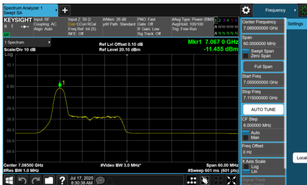
Plot 7-420 PSD SDM Diversity Antenna 4a (40MHz BW 802.11be(RU) RU26 Index0 - Ch.227)
