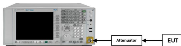
Figure 7-4. Test Instrument & Measurement Setup
