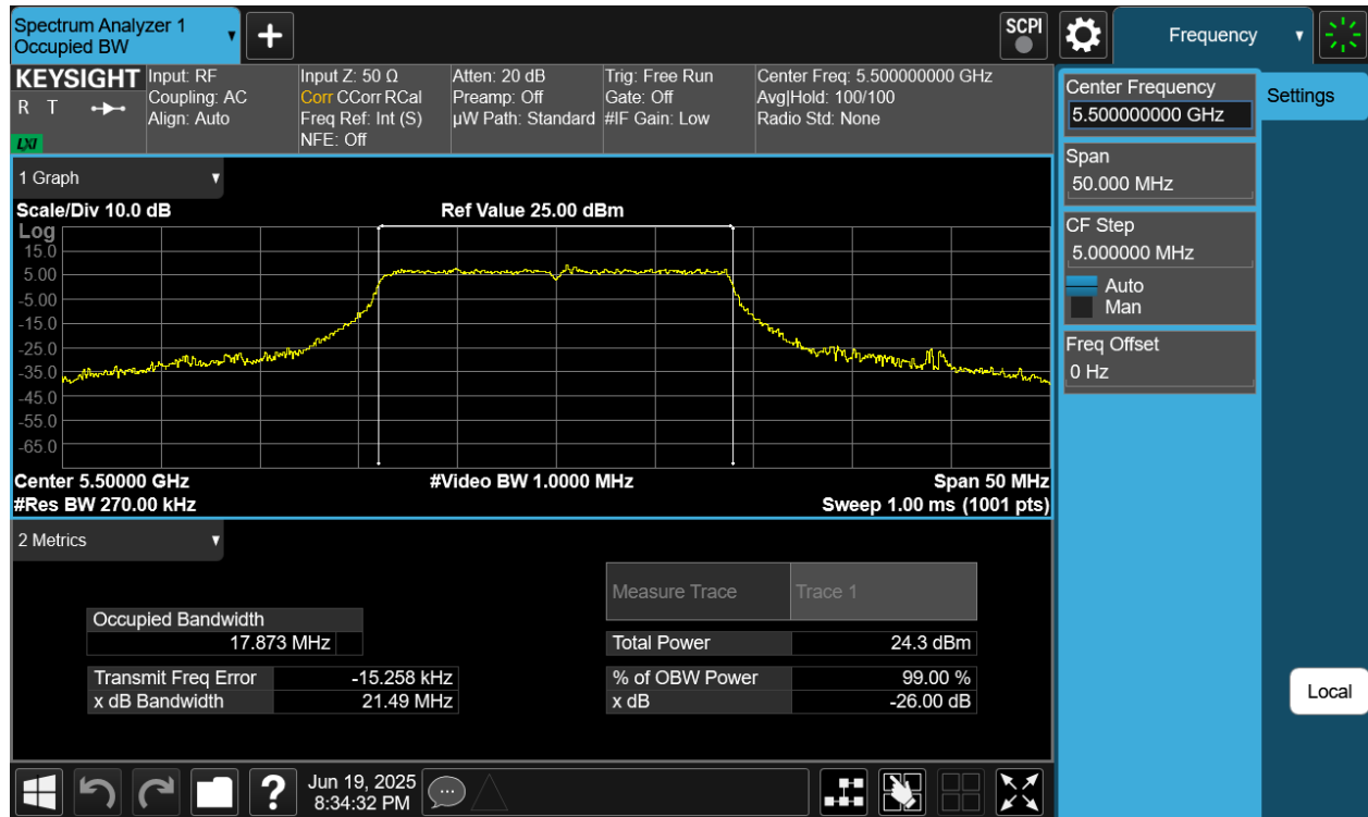
Plot 7-9 26dB BW & 99% OBW Antenna 2a (20MHz BW 802.11n - Ch.100)
