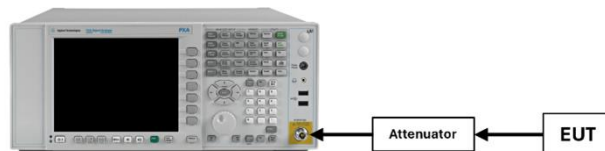
Figure 7-1. Test Instrument & Measurement Setup
