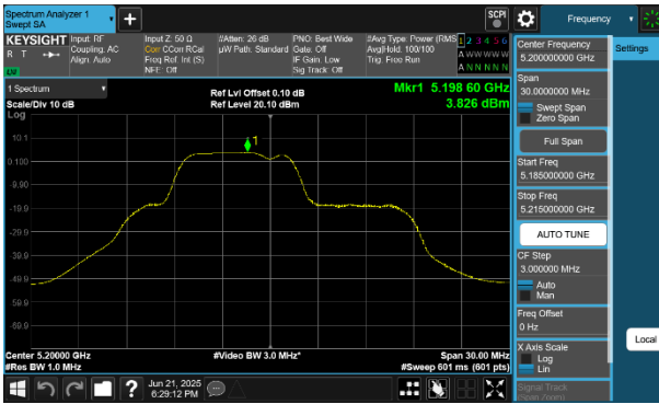
Plot 7-254 PSD SDM Diversity Antenna 2a (20MHz BW 802.11be(RU) RU52+26 Index71 - Ch.40)
