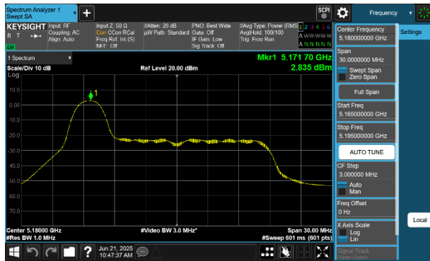
Plot 7-246 PSD SDM Diversity Antenna 2a (20MHz BW 802.11be(RU) RU26 Index0 - Ch.36)
