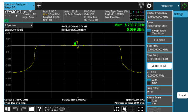
Plot 7-244 PSD CDD Diversity Antenna 4a (40MHz BW 802.11be(RU) RU484 Index65 - Ch.159)
