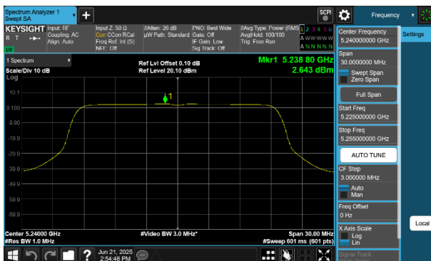
Plot 7-264 PSD SDM Diversity Antenna 4a (20MHz BW 802.11be(RU) RU242 Index61 - Ch.48)
