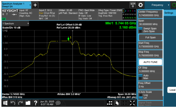
Plot 7-238 PSD CDD Diversity Antenna 4a (20MHz BW 802.11be(RU) RU52+26 Index71 - Ch.149)
