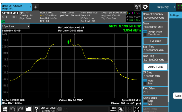
Plot 7-257 PSD SDM Diversity Antenna 4a (20MHz BW 802.11be(RU) RU52+26 Index71 - Ch.40)
