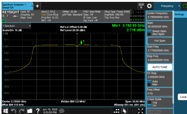
Plot 7-240 PSD CDD Diversity Antenna 2a (20MHz BW 802.11be(RU) RU242 Index61 - Ch.157)
