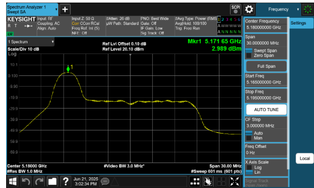
Plot 7-250 PSD SDM Diversity Antenna 4a (20MHz BW 802.11be(RU) RU26 Index0 - Ch.36)
