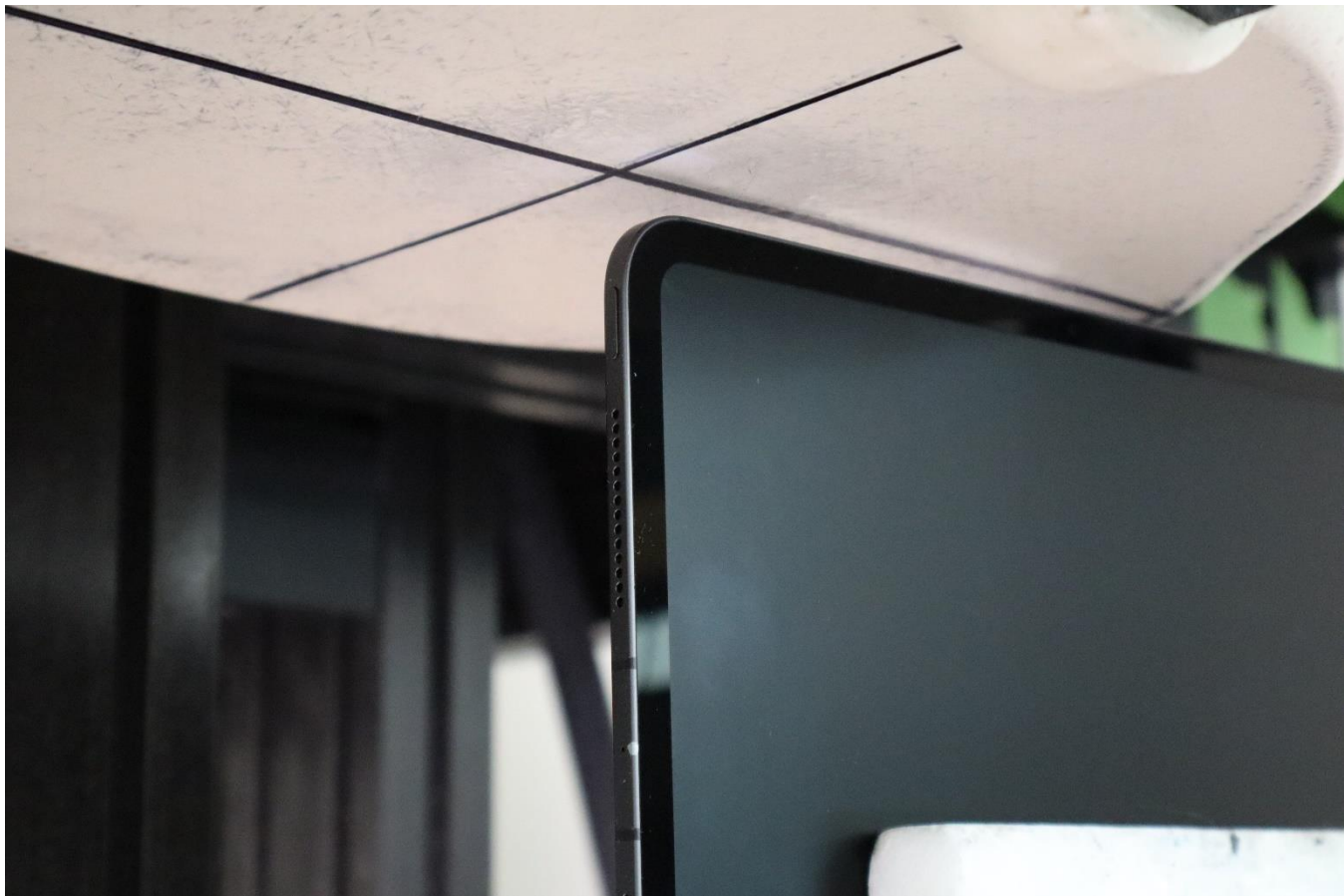
SAR Test Setup Photo 6: Body, Right Edge at 5.0 mm – Antenna 3/4a/4b
