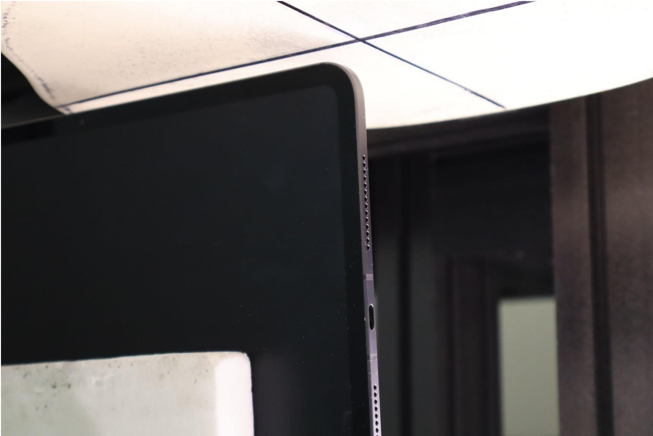
SAR Test Setup Photo 5: Body, Right Edge at 5.0 mm – Antenna 1/2a/2b/WF5B
