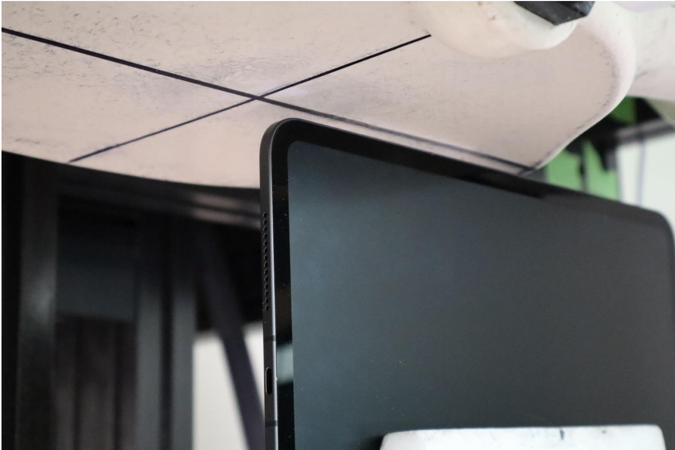
SAR Test Setup Photo 7: Body, Left Edge at 5.0 mm – Antenna 1/2a/2b/WF5B
