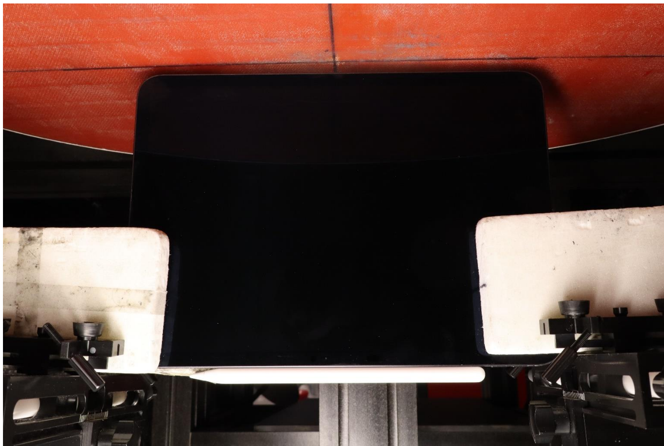
Wireless Power Transfer (wPT) Test Setup Photo 13: Left Edge at 5.0 mm
