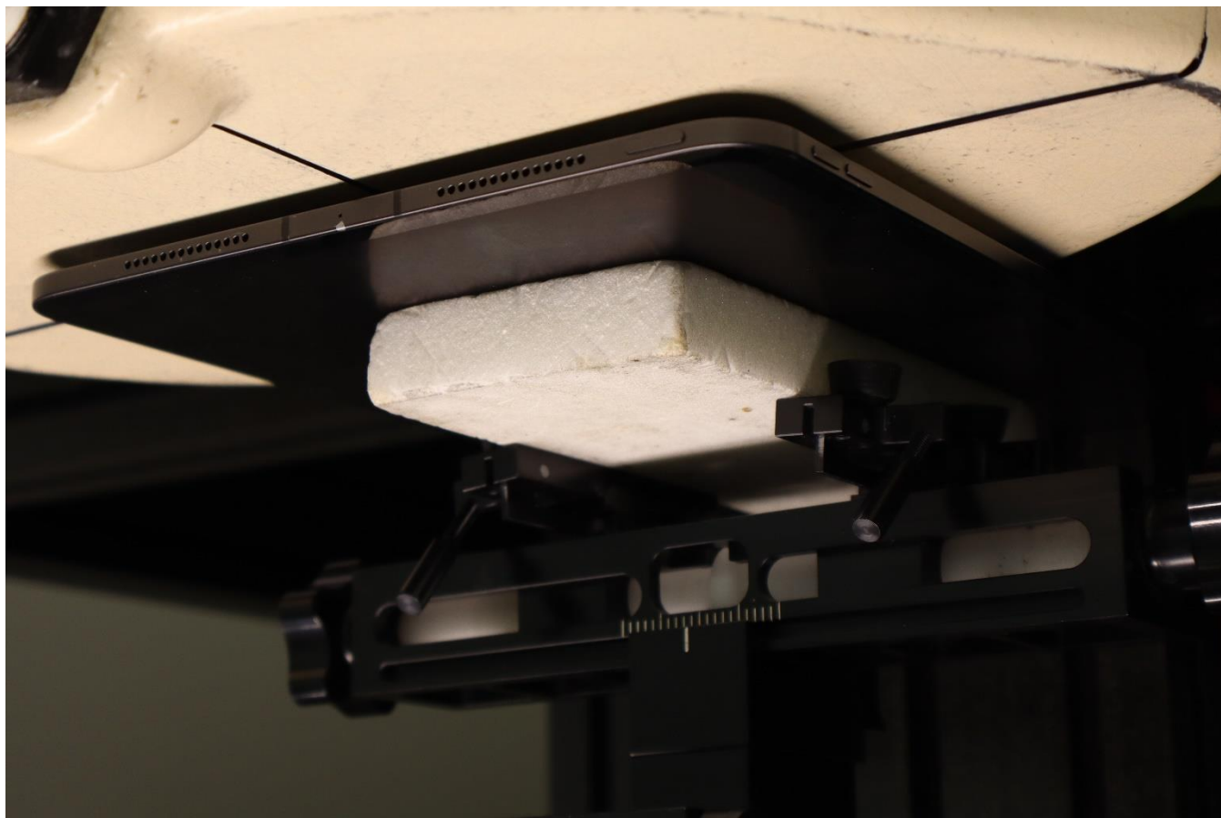
SAR Test Setup Photo 2: Body, Back Side at 5.0 mm – Antenna 3/4a/4b
