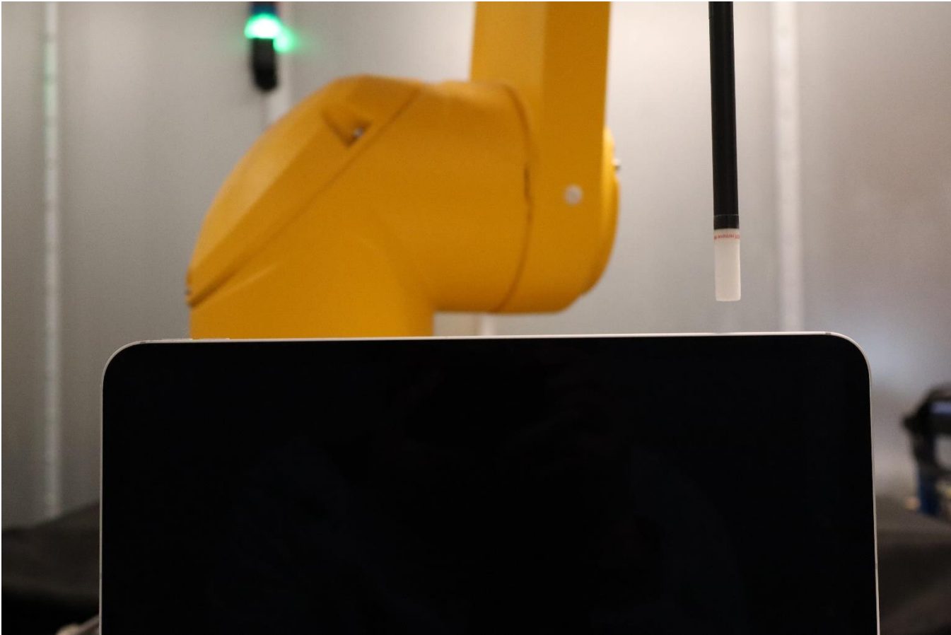
Near Field Power Density Test Setup Photo 22: Body, Right Edge at 9.69mm – WF5B
