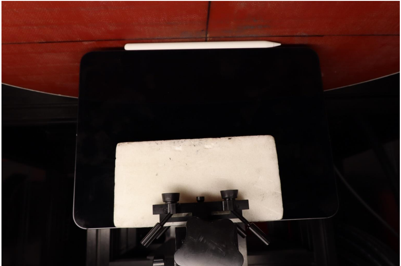
Wireless Power Transfer (wPT) Test Setup Photo 12: Right Edge at 5.0 mm
