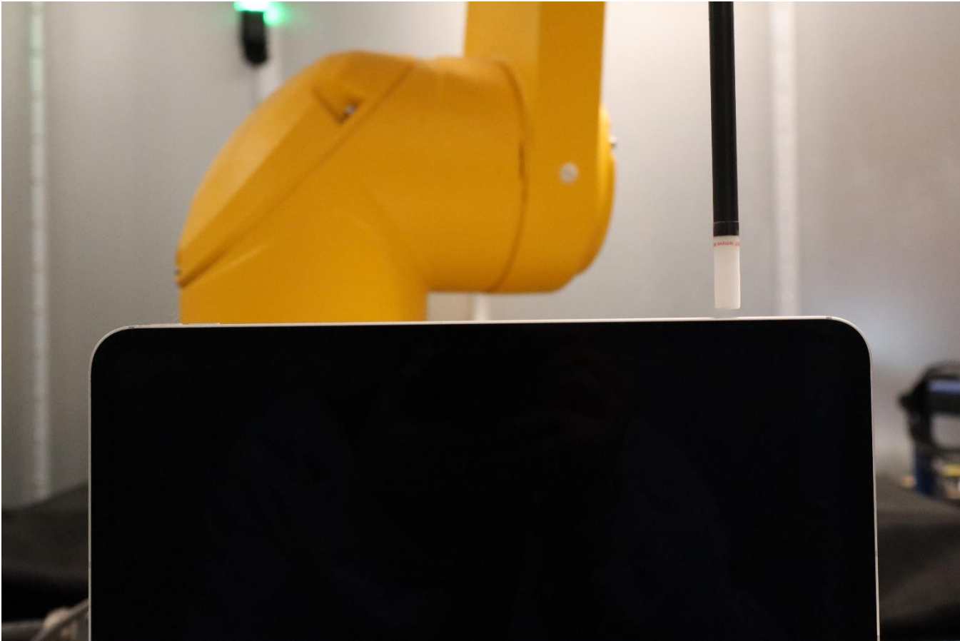
Near Field Power Density Test Setup Photo 20: Body, Right Edge at 2mm – WF5B
