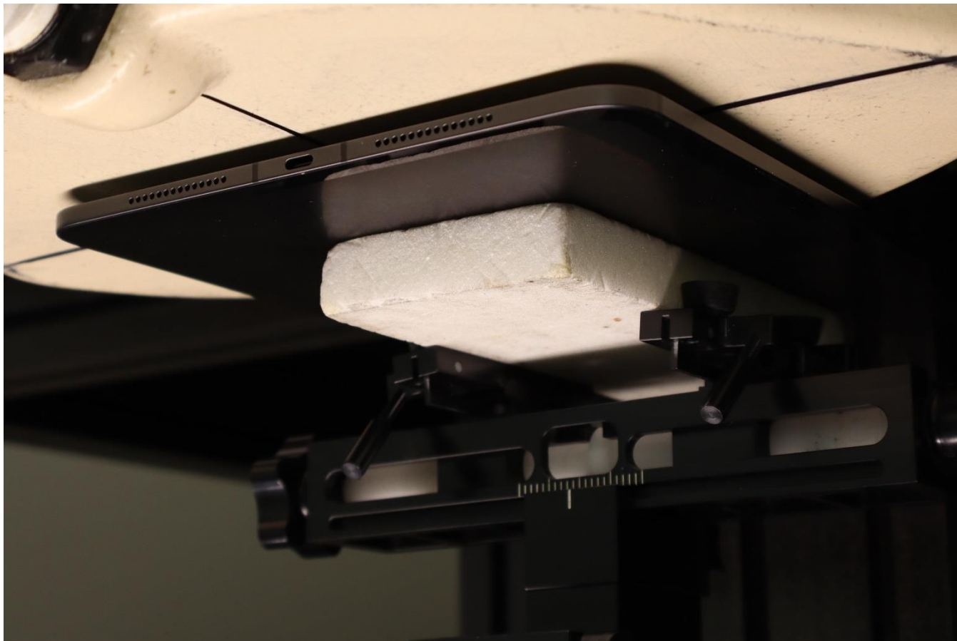
SAR Test Setup Photo 1: Body, Back Side at 5.0 mm – Antenna 1/2a/2b/WF5B
