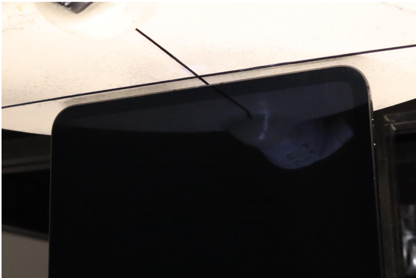
SAR Test Setup Photo 3: Body, Top Edge at 5.0 mm
