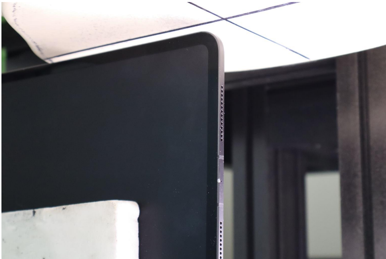
SAR Test Setup Photo 8: Body, Left Edge at 5.0 mm – Antenna 3/4a/4b
