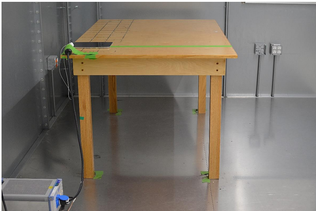
Figure 2: AC Line Conducted Emissions (Side View)
