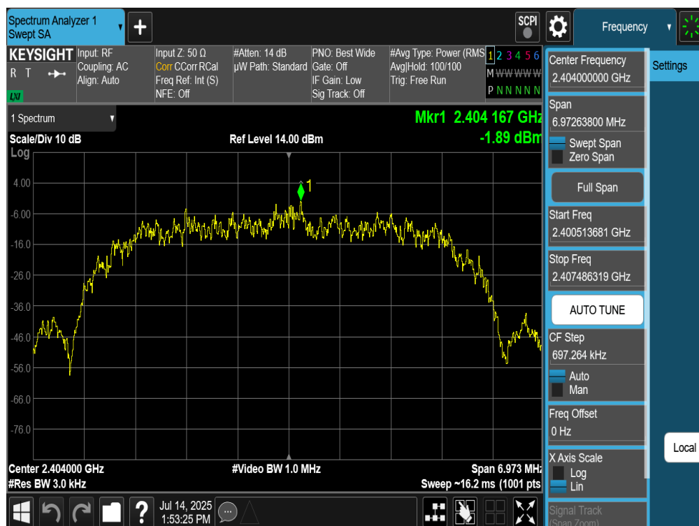
Plot 7-247. Power Spectral Density Plot TxBF Diversity Antenna WF8 (Bluetooth (HDR8), 8Mbps, ePA – Ch. 1)
