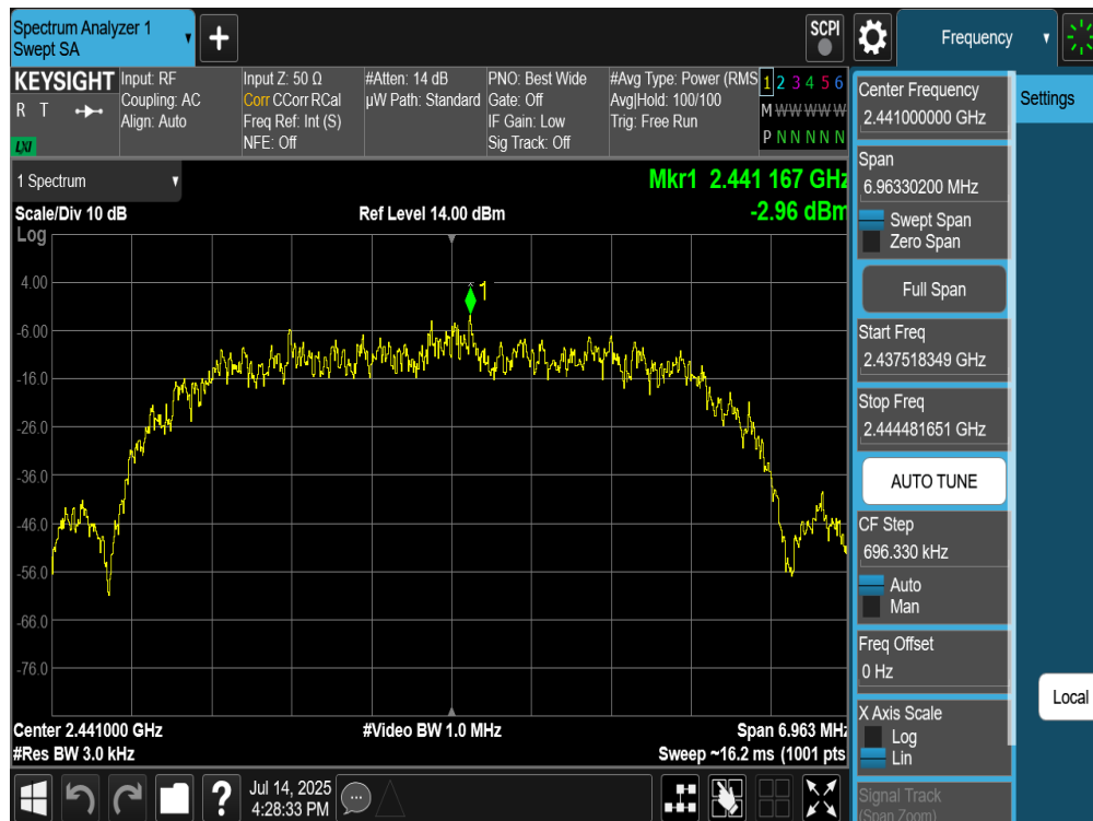
Plot 7-250. Power Spectral Density Plot TxBF Diversity Antenna WF9 (Bluetooth (HDR8), 8Mbps, ePA – Ch. 38)
