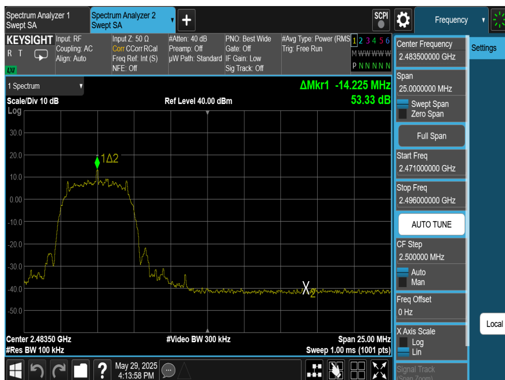
Plot 7-326. Band Edge Plot Antenna WF7 (Bluetooth (XHDRPM6), 6Mbps, ePA – Ch. 73)
