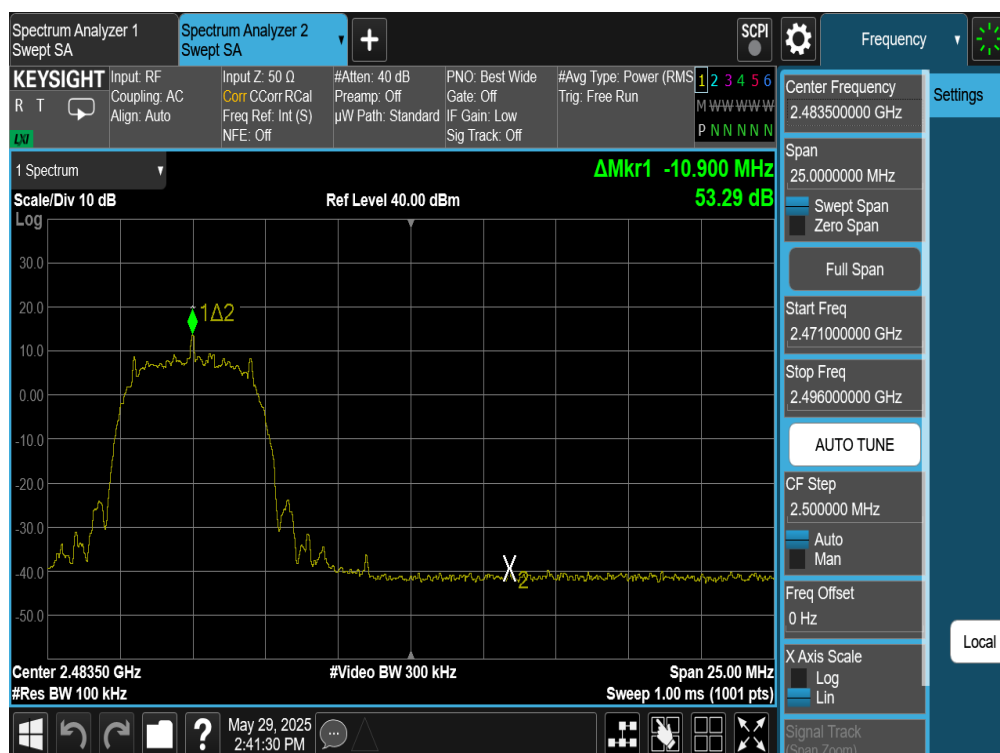
Plot 7-314. Band Edge Plot Antenna WF8 (Bluetooth (XHDRPM6), 6Mbps, ePA – Ch. 73)
