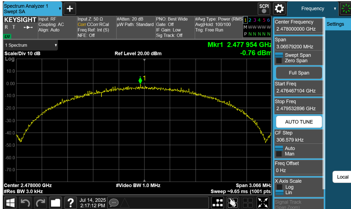
Plot 7-81. Power Spectral Density Plot Antenna WF7 (Bluetooth (LE), 2Mbps, ePA – Ch. 38)
