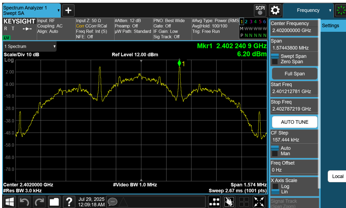
Plot 7-85. Power Spectral Density Plot Antenna WF9 (Bluetooth (LE), 125kbps, ePA – Ch. 0)
