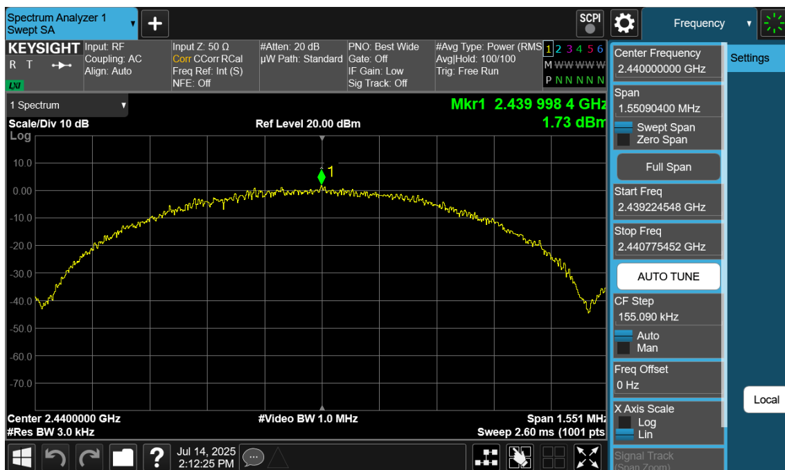
Plot 7-74. Power Spectral Density Plot Antenna WF7 (Bluetooth (LE), 1Mbps, ePA – Ch. 19)
