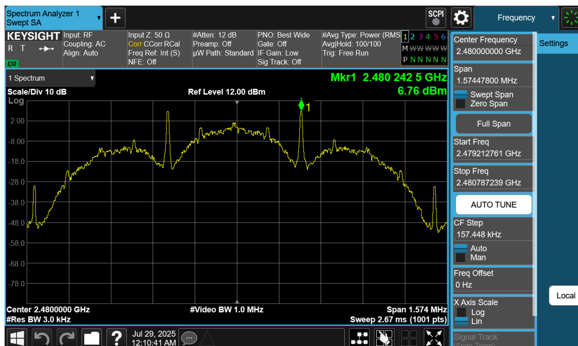
Plot 7-87. Power Spectral Density Plot Antenna WF9 (Bluetooth (LE), 125kbps, ePA – Ch. 39)
