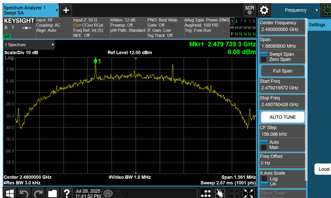
Plot 7-69. Power Spectral Density Plot Antenna WF7 (Bluetooth (LE), 500kbps, ePA – Ch. 39)
