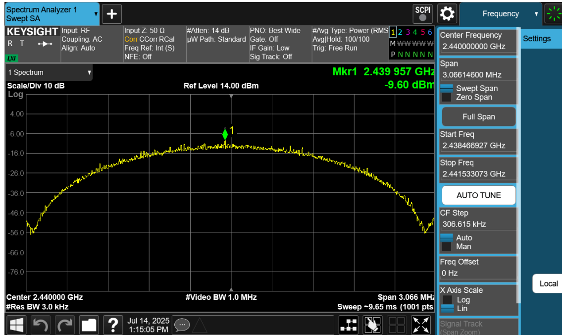
Plot 7-59. Power Spectral Density Plot Antenna WF8 (Bluetooth (LE), 2Mbps, iPA – Ch. 19)
