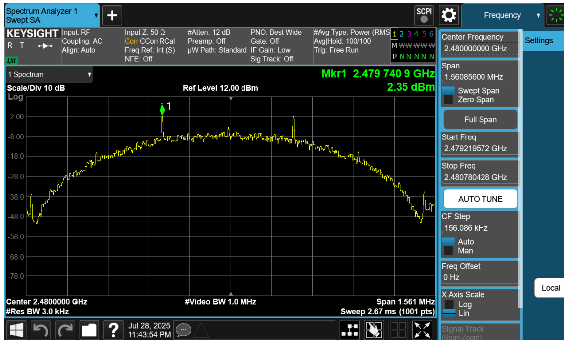
Plot 7-72. Power Spectral Density Plot Antenna WF7 (Bluetooth (LE), 500kbps, iPA – Ch. 39)
