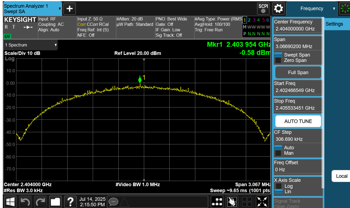
Plot 7-79. Power Spectral Density Plot Antenna WF7 (Bluetooth (LE), 2Mbps, ePA – Ch. 1)
