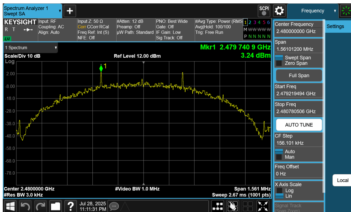
Plot 7-48. Power Spectral Density Plot Antenna WF8 (Bluetooth (LE), 500kbps, iPA – Ch. 39)
