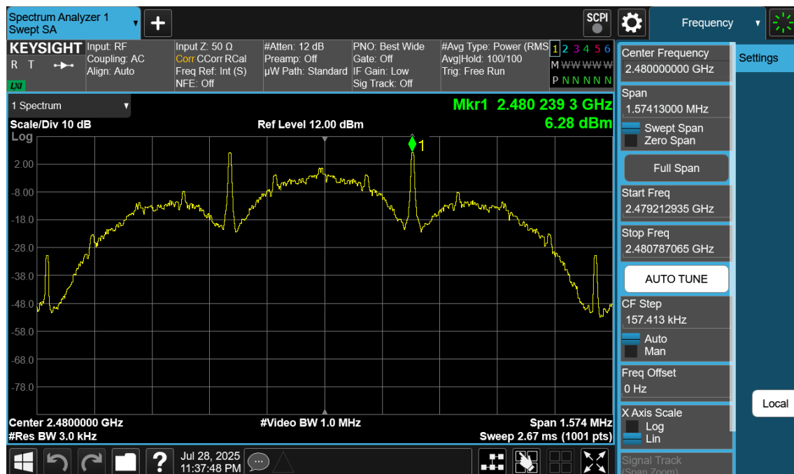
Plot 7-63. Power Spectral Density Plot Antenna WF7 (Bluetooth (LE), 125kbps, ePA – Ch. 39)
