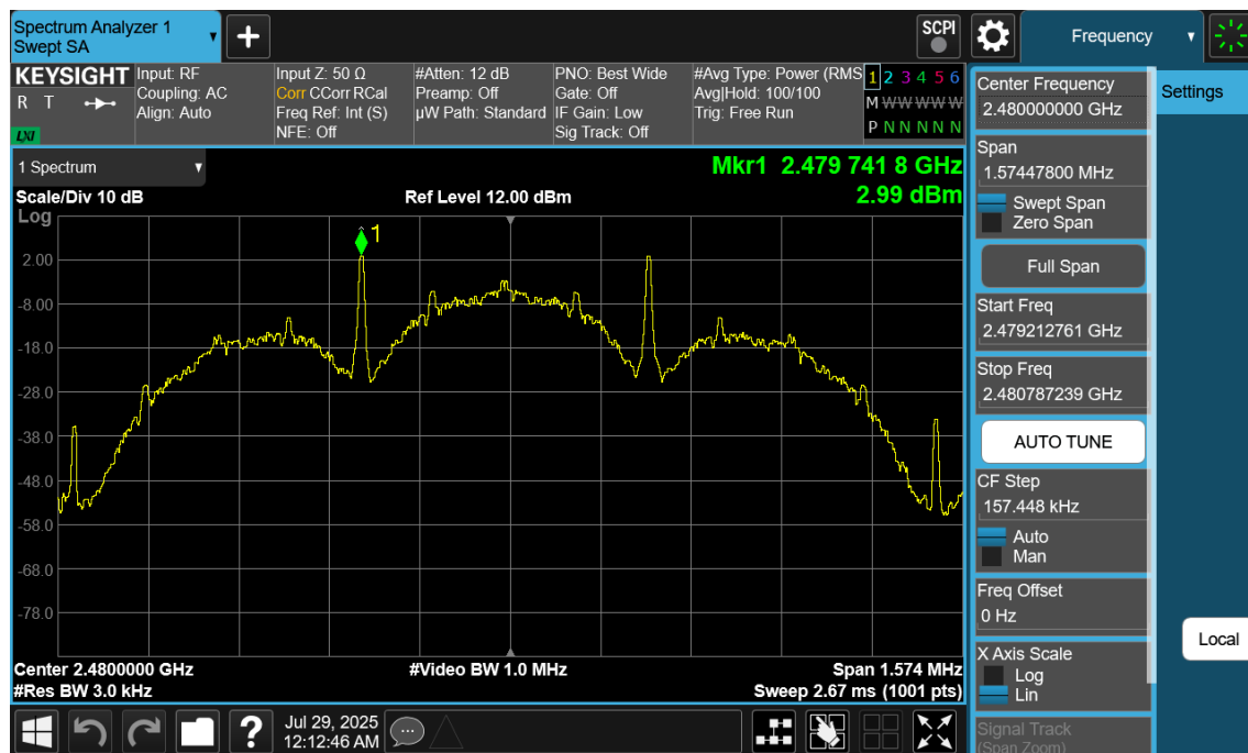
Plot 7-90. Power Spectral Density Plot Antenna WF9 (Bluetooth (LE), 125kbps, iPA – Ch. 39)
