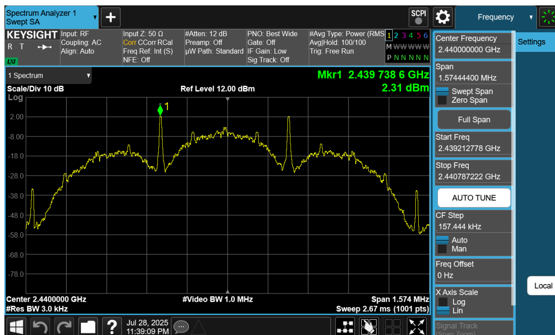
Plot 7-65. Power Spectral Density Plot Antenna WF7 (Bluetooth (LE), 125kbps, iPA – Ch. 19)
