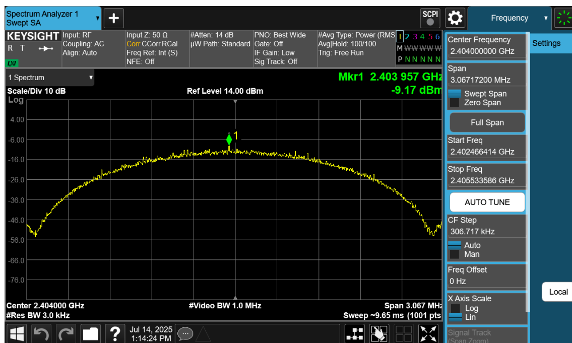
Plot 7-58. Power Spectral Density Plot Antenna WF8 (Bluetooth (LE), 2Mbps, iPA – Ch. 1)
