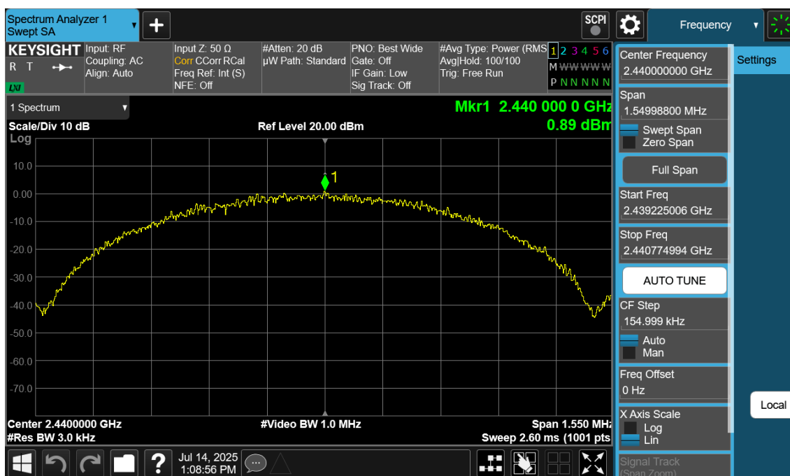
Plot 7-50. Power Spectral Density Plot Antenna WF8 (Bluetooth (LE), 1Mbps, ePA – Ch. 19)
