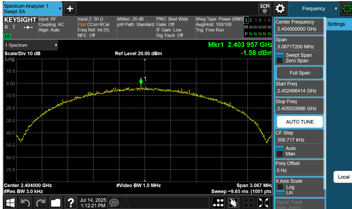
Plot 7-55. Power Spectral Density Plot Antenna WF8 (Bluetooth (LE), 2Mbps, ePA – Ch. 1)
