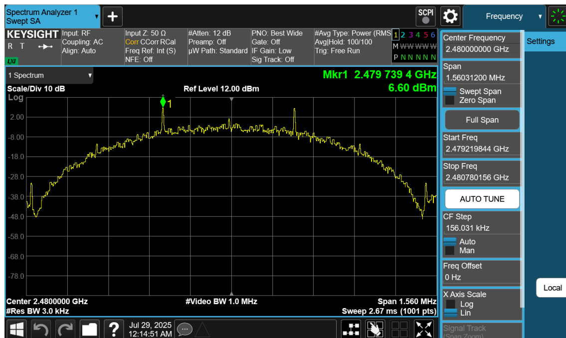
Plot 7-93. Power Spectral Density Plot Antenna WF9 (Bluetooth (LE), 500kbps, ePA – Ch. 39)
