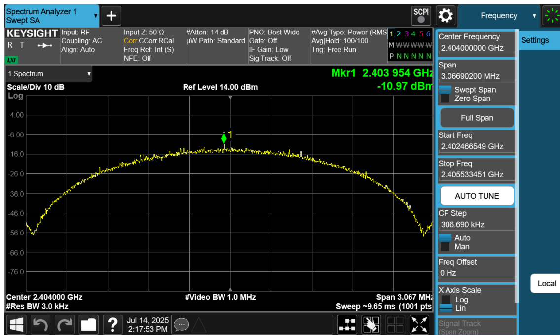
Plot 7-82. Power Spectral Density Plot Antenna WF7 (Bluetooth (LE), 2Mbps, iPA – Ch. 1)
