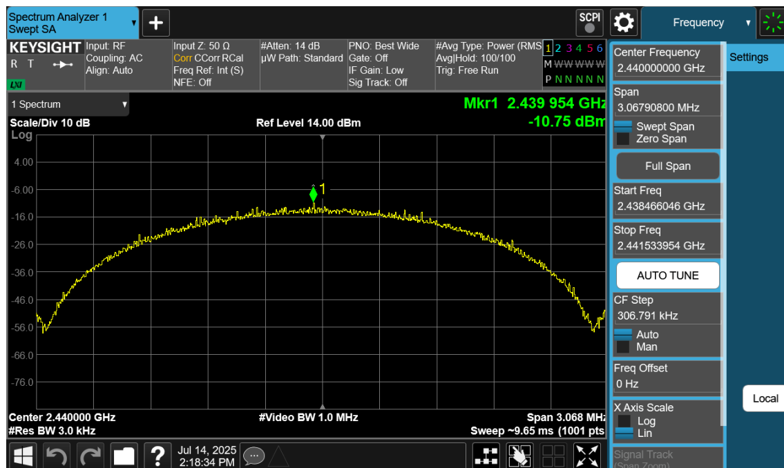
Plot 7-83. Power Spectral Density Plot Antenna WF7 (Bluetooth (LE), 2Mbps, iPA – Ch. 19)
